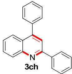
**2,4-Diphenylquinoline (3ch)<sup>11</sup>:** White solid, mp 112-115 °C; IR (KBr) cm<sup>-1</sup>: 3423, 3086, 2955, 1589, 1095, 846 cm<sup>-1</sup>; <sup>1</sup>H NMR (300 MHz, CDCl<sub>3</sub>) δ: 7.81 (d, *J* = 7.2 Hz, 4H, ArH), 7.67-7.56 (m, 4H, ArH), 7.51-7.38 (m 5H, ArH), 7.35-7.31 (m, 2H, ArH); <sup>13</sup>C NMR (75 MHz, CDCl<sub>3</sub>) δ: 163.1, 140.5, 137.5, 136.2, 136.0, 133.6, 133.0, 132.3, 131.8, 131.0, 130.0, 129.9, 129.0, 128.8, 128.5, 128.2, 128.1, 127.1, 119.4, 118.5, 118.5.
