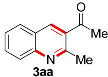
**3-Acetyl-2-methyl quinoline (3aa)<sup>1</sup>:** Pale yellow solid, mp 74-75 °C; IR (KBr) cm<sup>-1</sup>: 3053, 1788, 1624, 1579, 1456, 818 cm<sup>-1</sup>; <sup>1</sup>H NMR (300 MHz, CDCl<sub>3</sub>) δ: 8.48 (s, 1H, ArH), 8.05 (d, *J* = 8.4 Hz, 1H, ArH), 7.87-7.76 (m, 2H, ArH), 7.57-7.52 (m, 1H, ArH), 2.91 (s, 3H, COCH<sub>3</sub>) 2.72 (s, 3H, CH<sub>3</sub>); <sup>13</sup>C NMR (75 MHz, CDCl<sub>3</sub>): δ 199.9, 157.5, 138.2, 138.1, 131.6, 131.1, 128.5, 128.2, 126.6, 125.5, 29.2, 25.6.
