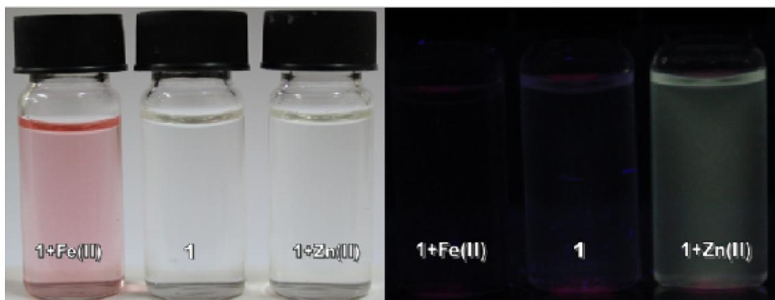
**Figure S9.** Chromogenic (left) and fluorogenic (right) responses of **1** to metal ions in aqueous 0.1 M HEPES containing 0.1% CH<sub>3</sub>OH (v/v) solution (pH= 7.2, 25°C) under room light and UV illumination (365 nm), respectively.
