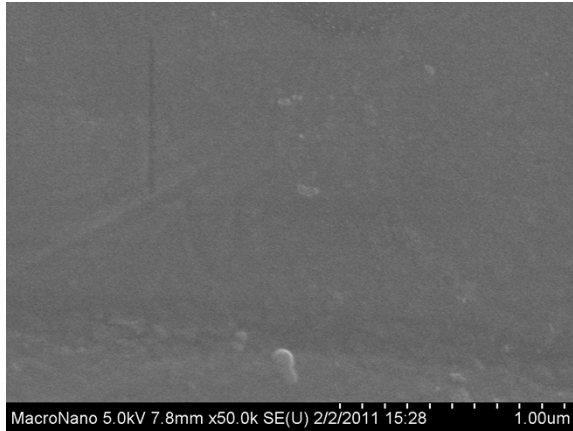
(A) Treatment of polycarbonate with 0.5% propargyl amine solution in ethanol
