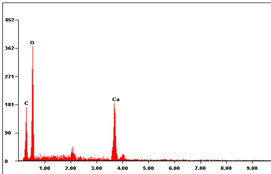
**Fig. S3** EDX spectrum of 3D hierarchical CaCO<sub>3</sub> hollow microspherical adsorbent composed of 1D spike-shaped nanorods
