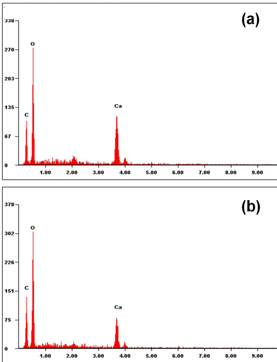
**Fig. S7** EDX spectra of Ca(OH)<sub>2</sub> and (b) CaC<sub>2</sub>O<sub>4</sub>·H<sub>2</sub>O adsorbents synthesized with (a) 6 M and (b) 10 M NaOH.
