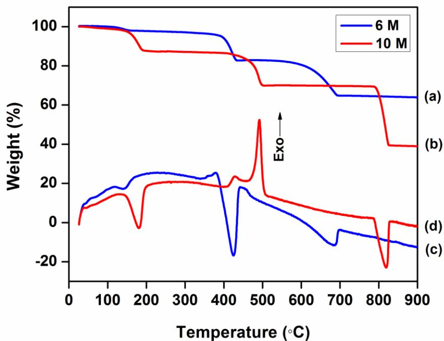
**Fig. S8** TG-DTA curves of  $\text{Ca}(\text{OH})_2$  and  $\text{CaC}_2\text{O}_4 \cdot \text{H}_2\text{O}$  adsorbents synthesized with 6 and 10 M NaOH.
