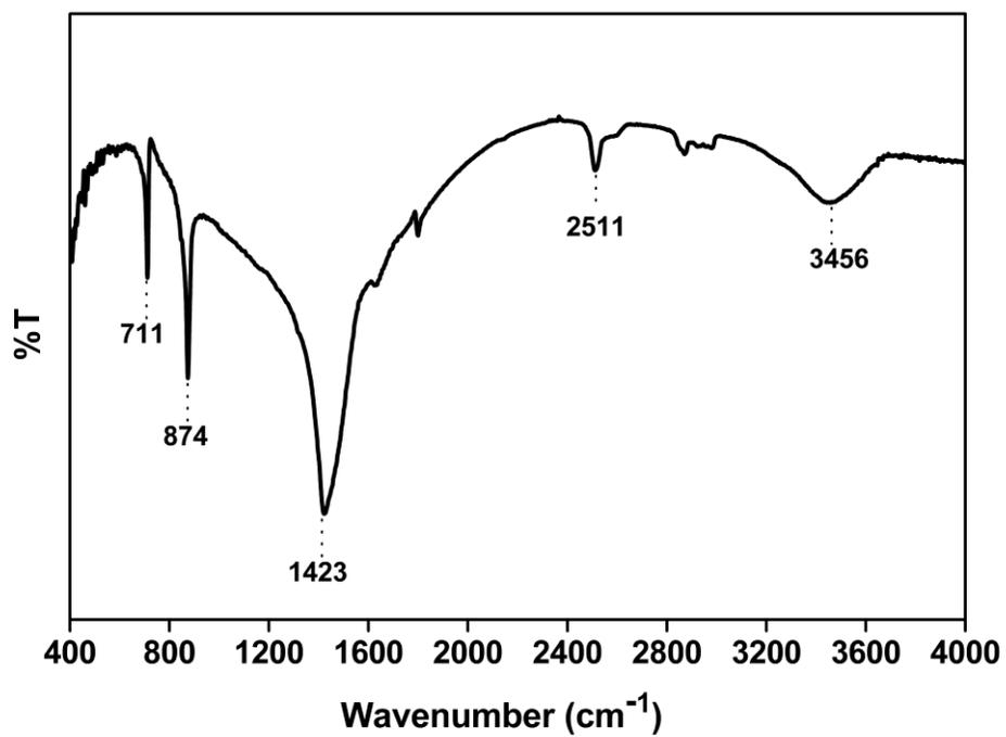
**Fig. S2** FTIR spectrum of 3D hierarchical CaCO<sub>3</sub> hollow microspherical adsorbent composed of 1D spike-shaped nanorods
