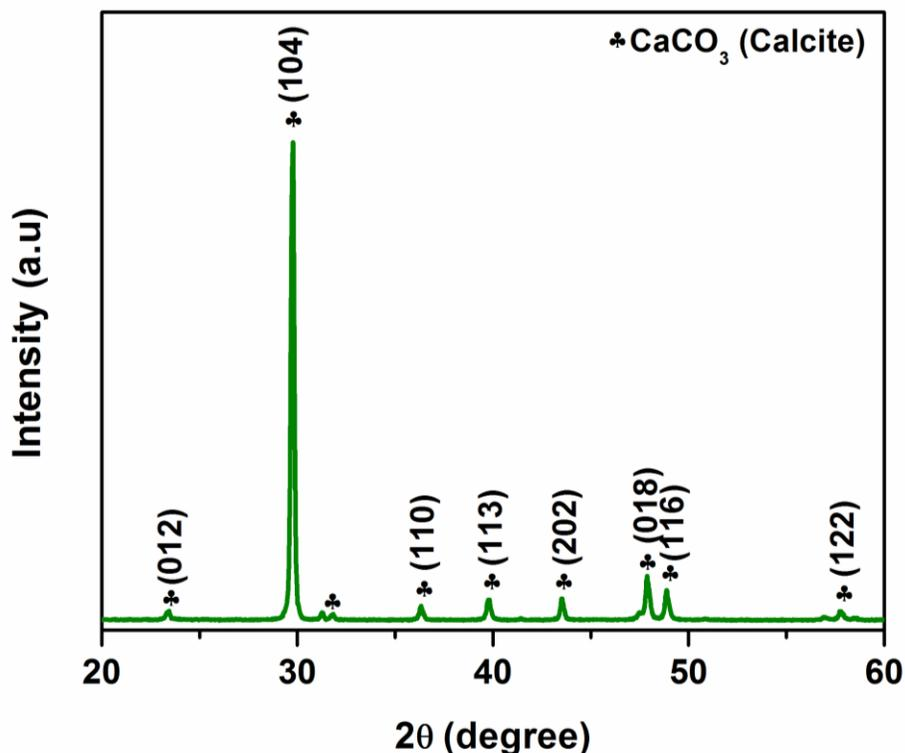
Fig. S1 XRD pattern of limestone (CaCO<sub>3</sub>).
