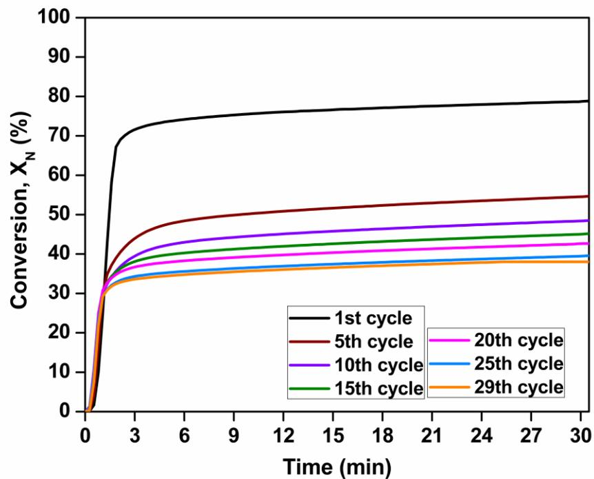
**Fig. S9** Multi cycles carbonation conversion curves of 3D hierarchical  $\text{CaCO}_3$  hollow microspherical adsorbent composed of 1D spike-shaped nanorods
