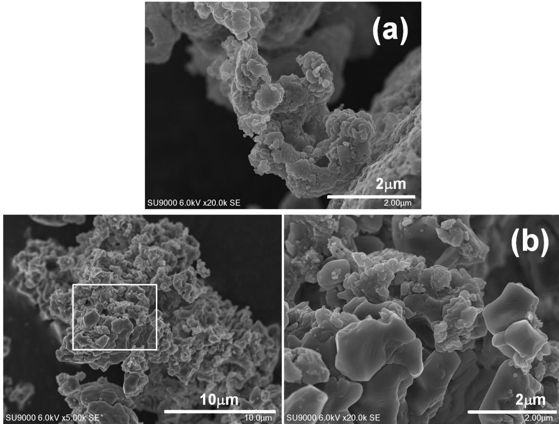
**Fig. S10** FESEM images of the calcined 3D hierarchical  $\text{CaCO}_3$  hollow microspherical adsorbent composed of 1D spike-shaped nanorods (a) after 1 cycle (b) after 29 cycles.
