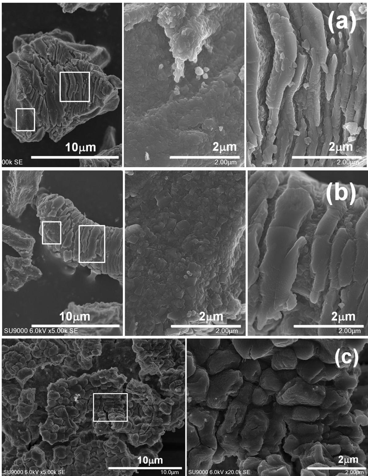
**Fig. S11** FESEM images of the calcined adsorbents after 15 cycles (a)  $\text{Ca(OH)}_2$ , (b)  $\text{CaC}_2\text{O}_4 \cdot \text{H}_2\text{O}$  and (c) limestone.
