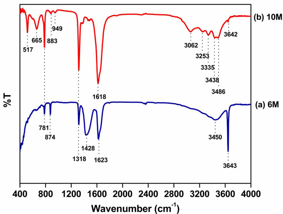
**Fig. S6** FTIR spectra of Ca(OH)<sub>2</sub> and CaC<sub>2</sub>O<sub>4</sub>.H<sub>2</sub>O adsorbents synthesized with (a) 6 M and (b) 10 M NaOH.
