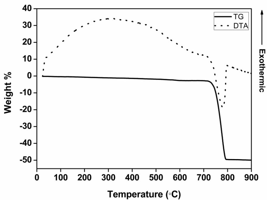
Fig. S5 TG-DTA curves of 3D hierarchical  $\text{CaCO}_3$  hollow microspherical adsorbent composed of 1D spike-shaped nanorods
