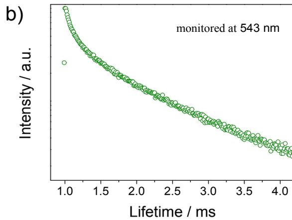
**Figure S2.** Decay curves of  $^5D_0$  state for  $\text{Eu}^{3+}$  in AC-Bipy-Eu (a) and  $^5D_4$  state for  $\text{Tb}^{3+}$  in AC-Bipy-Tb (b) after excitation at 300 nm.
