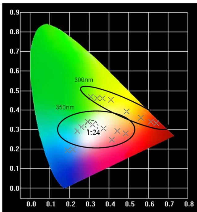
**Figure S4.** CIE 1931 chromaticity diagram within the co-ordinates of AC-Bipy-Ln (film) excited at 300 nm and 325 nm. The film of AC-Bipy-Eu<sub>1</sub>Tb<sub>24</sub> excited at 350 nm exhibits nearly perfect white light emission with the 15 corresponding CIE co-ordinate of (0.32, 0.33).
