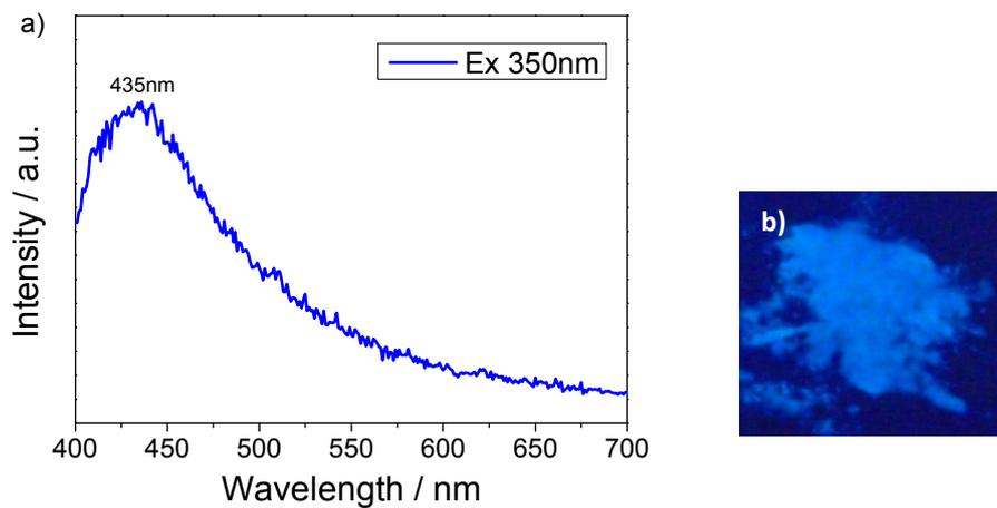
10 **Figure S1.** a) Emission spectra of AC-Bipy excited at 350 nm (room temperature) and b) digital photograph of AC-Bipy under 365 nm UV lamp illumination.
