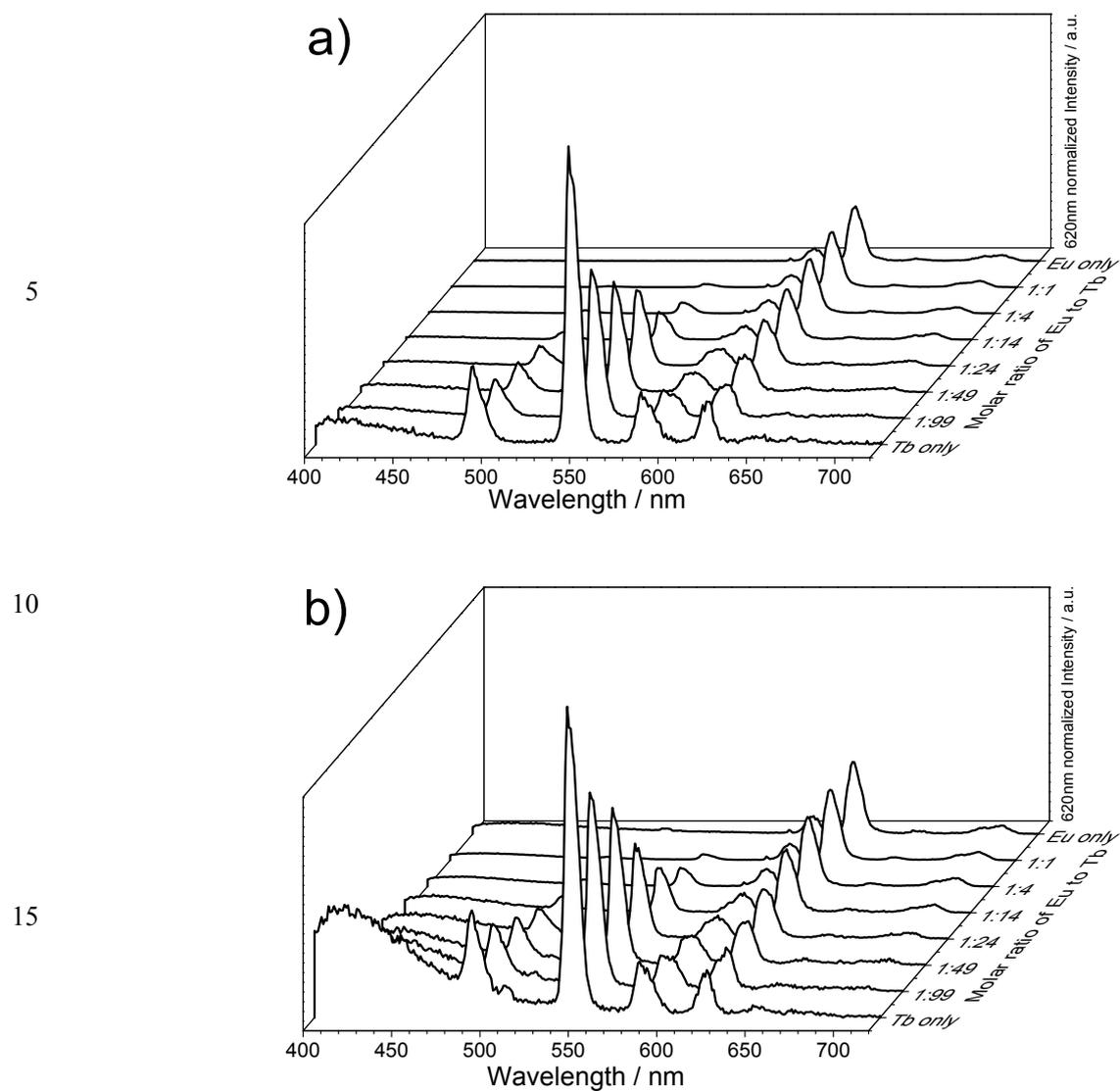
**Figure S3.** Emission spectra (normalized at 620 nm) of the transparent luminescent thin films excited at 300 nm (a) 20 and 350 nm (b). (All the spectra were obtained at room temperature)
