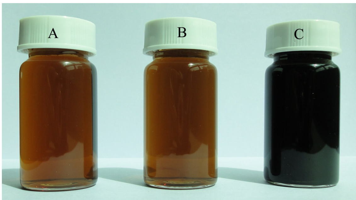
Fig. S1. The color change of exfoliated GO suspension in different procedure. A) is GO; B) is GO heated at 90 °C for 2 h; C) is GO mixed with K 2 CO 3 solution and heated at 90 °C for 2 h.
