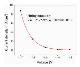
**Figure S 3.** The polarized current density with different voltages setting up in the two-electrodes cell for electrolyzing Fe<sub>2</sub>O<sub>3</sub>. The current density was recorded when electrolyzing carried on for half an hour.
