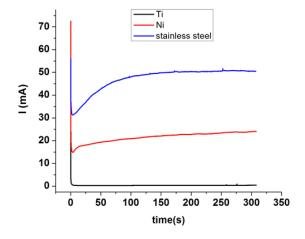
**Figure S 2.** The background current with of three kinds of current collector. Ti plate, Ni plate and stainless steel plate were immersed into NaOH solution separately, and 1.7 V of voltage was applied between the tested material and the Pt foil counter electrode.
