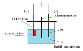
**Figure S 1.** The two-electrode electrolytic cell for Fe<sub>2</sub>O<sub>3</sub> electrolysis.
