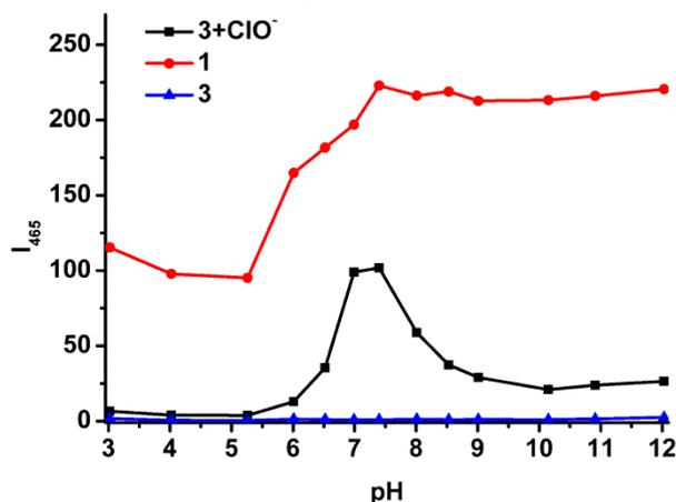
Figure S4 Effect of pH values to the relative fluorescence intensity of 5  $\mu$ M **1** (●), 5  $\mu$ M **3** (▲) and reaction between 5  $\mu$ M **3** and 50  $\mu$ M ClO<sup>-</sup> in water (0.5% DMSO in volum) buffered by 20 mM HEPES at pH 7.40 (■) for 30 min at ambient temperature. (The investigated pH values include 3.02, 4.02, 5.26, 6.01, 6.52, 6.99, 7.40, 8.01, 8.53, 9.01, 10.15, 10.91 and 12.03).
