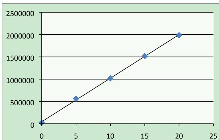
**Figure S5** Fluorescence changes with various concentrations of HClO/CIO<sup>-</sup> at 465 nm in the reaction between **3** and HClO/CIO<sup>-</sup> at ambient temperature.
