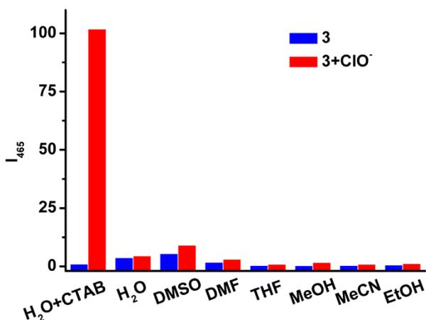
**Figure S1** Fluorescence responds of the reaction between **3** (5  $\mu\text{M}$ ) and  $\text{ClO}^-$  (50  $\mu\text{M}$ ) in HEPES buffer (0.5% DMSO, 20 mM, pH 7.40) at ambient temperature for 30 min. Fluorescence intensity was collected at 465 nm.  $\lambda_{\text{ex}}=350$  nm, slits: 5/5 nm.
