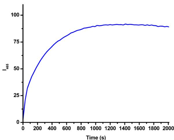
**Figure S6.** Time-dependent fluorescence changes of **3** (5 μM) in present of HClO (50 μM) at ambient temperature. λ<sub>ex</sub>=350 nm, slits: 5/5 nm, emission intensity was collected at λ<sub>em</sub>=465 nm.
