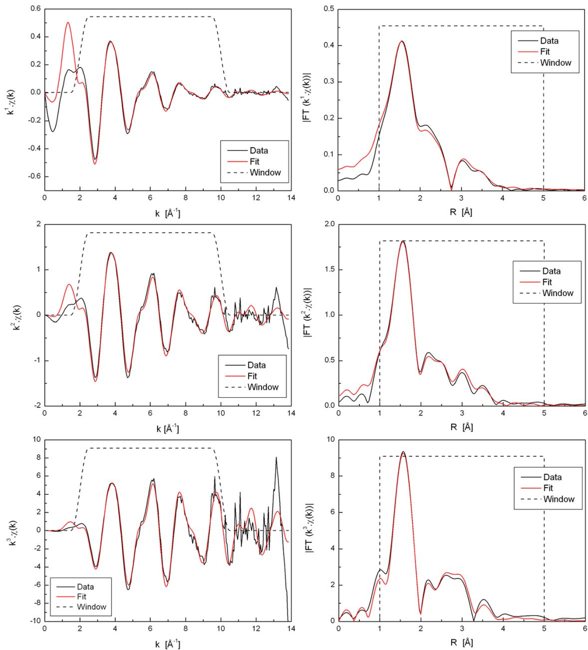
**Figure S3.**  $\text{Ni}(\text{NO}_3)_2$  in DMSO ('Sample 3') EXAFS data (black lines) and fits (red lines) in  $k$ -space (left) and  $R$ -space (right) for various  $k$ -weightings:  $k^1$  (top),  $k^2$  (middle),  $k^3$  (bottom). The data ranges used for fitting are shown by the window functions (black dashed lines).
