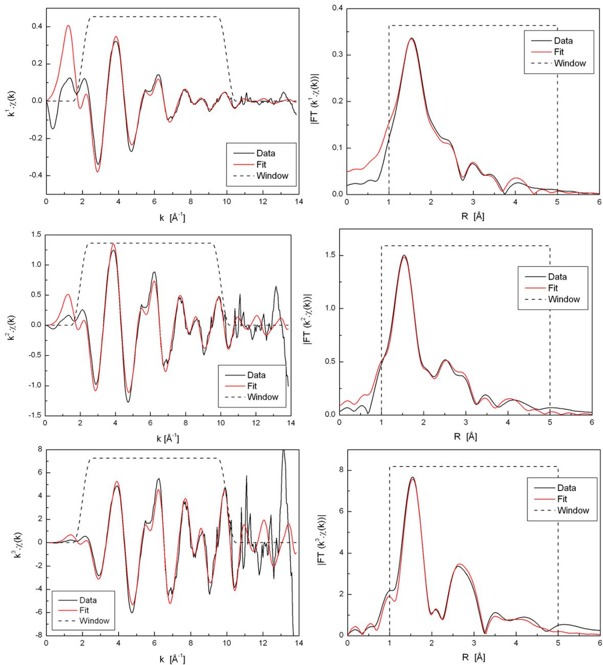
**Figure S5.** Ni-NCS 2:1 KSCN:Ni<sup>2+</sup> mole ratio model solution in DMSO ('Sample 5'), fitted using a single shell model. EXAFS data (black lines) and fits (red lines) in k-space (left) and R-space (right) for various k-weightings: k<sup>1</sup> (top), k<sup>2</sup> (middle), k<sup>3</sup> (bottom). The data ranges used for fitting are shown by the window functions (black dashed lines).
