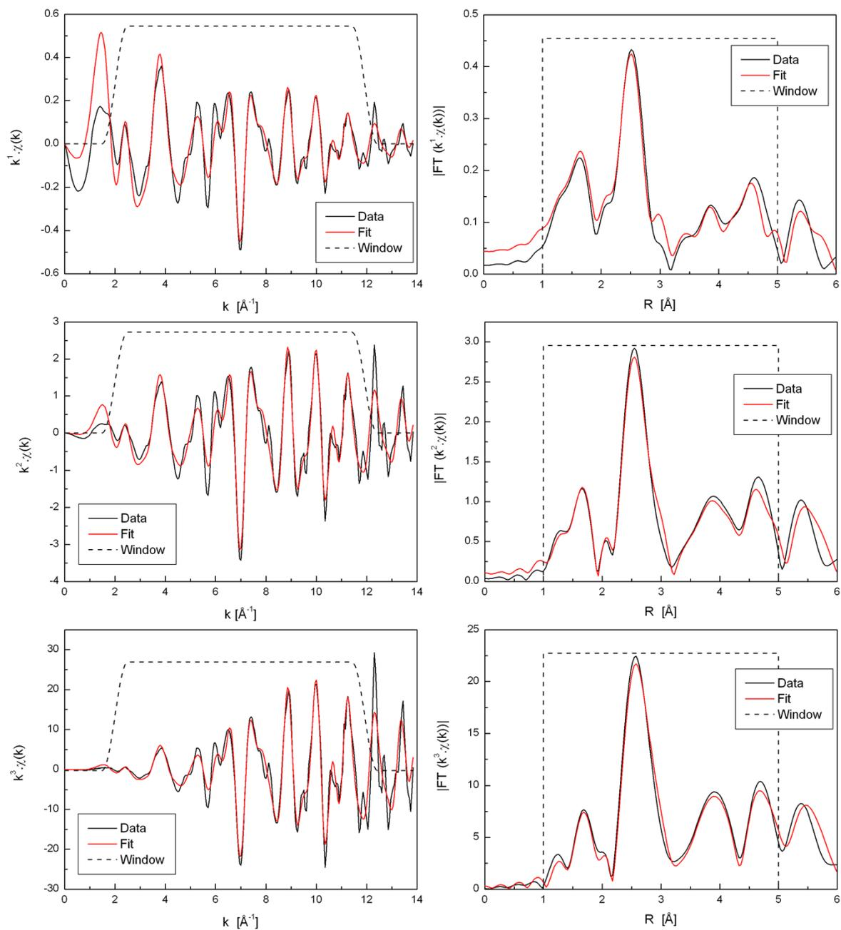
**Figure S1.** NiO powder standard ('Sample 1') EXAFS data (black lines) and fits (red lines) in  $k$ -space (left) and  $R$ -space (right) for various  $k$ -weightings:  $k^1$  (top),  $k^2$  (middle),  $k^3$  (bottom). The data ranges used for fitting are shown by the window functions (black dashed lines).
