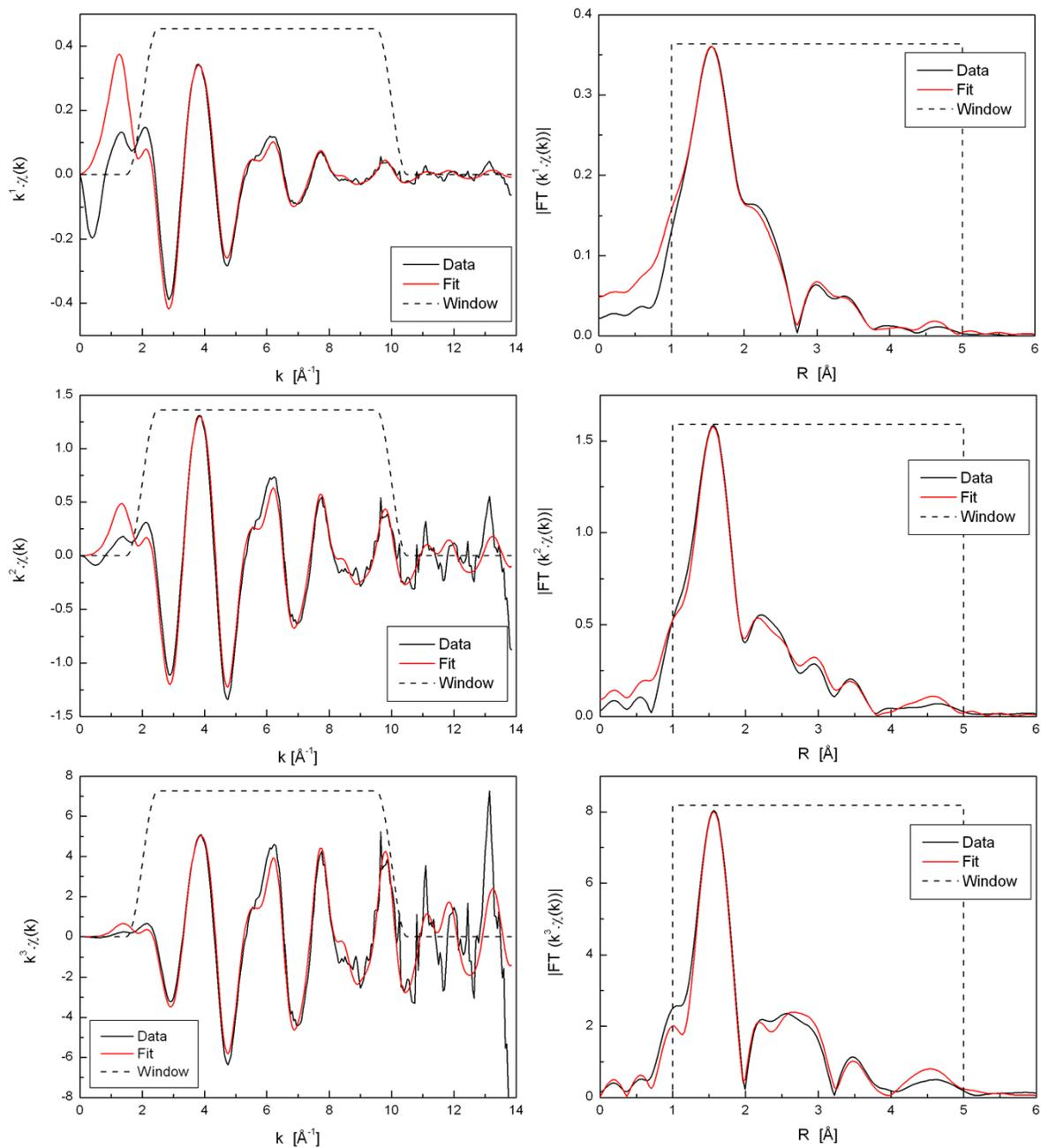
**Figure S6.** Ni-NcSe 2:1 KSeCN:Ni<sup>2+</sup> mole ratio model solution in DMSO ('Sample 6'), fitted using a single shell model. EXAFS data (black lines) and fits (red lines) in k-space (left) and R-space (right) for various k-weightings: k<sup>1</sup> (top), k<sup>2</sup> (middle), k<sup>3</sup> (bottom). The data ranges used for fitting are shown by the window functions (black dashed lines).
