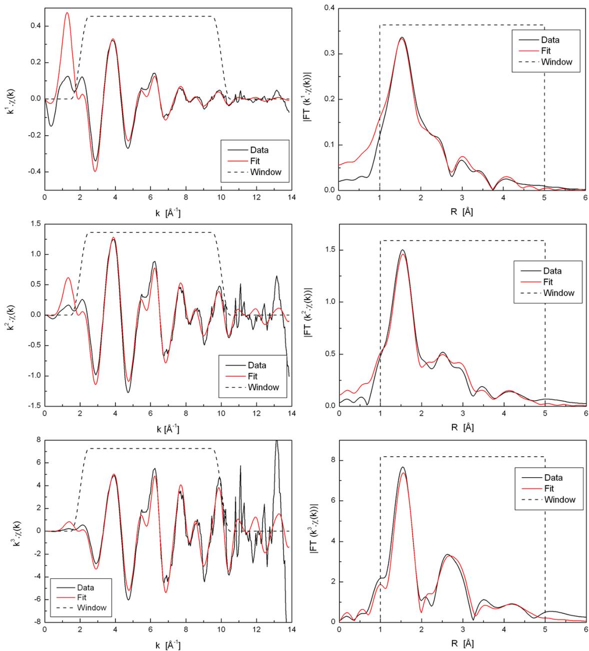
**Figure S9.** Ni-NCS 2:1 KSCN:Ni<sup>2+</sup> mole ratio model solution in DMSO ('Sample 5'), fitted using a single shell model for DMSO and a multiple-scattering model for SCN. EXAFS data (black lines) and fits (red lines) in k-space (left) and R-space (right) for various k-weightings: k<sup>1</sup> (top), k<sup>2</sup> (middle), k<sup>3</sup> (bottom). The data ranges used for fitting are shown by the window functions (black dashed lines).
