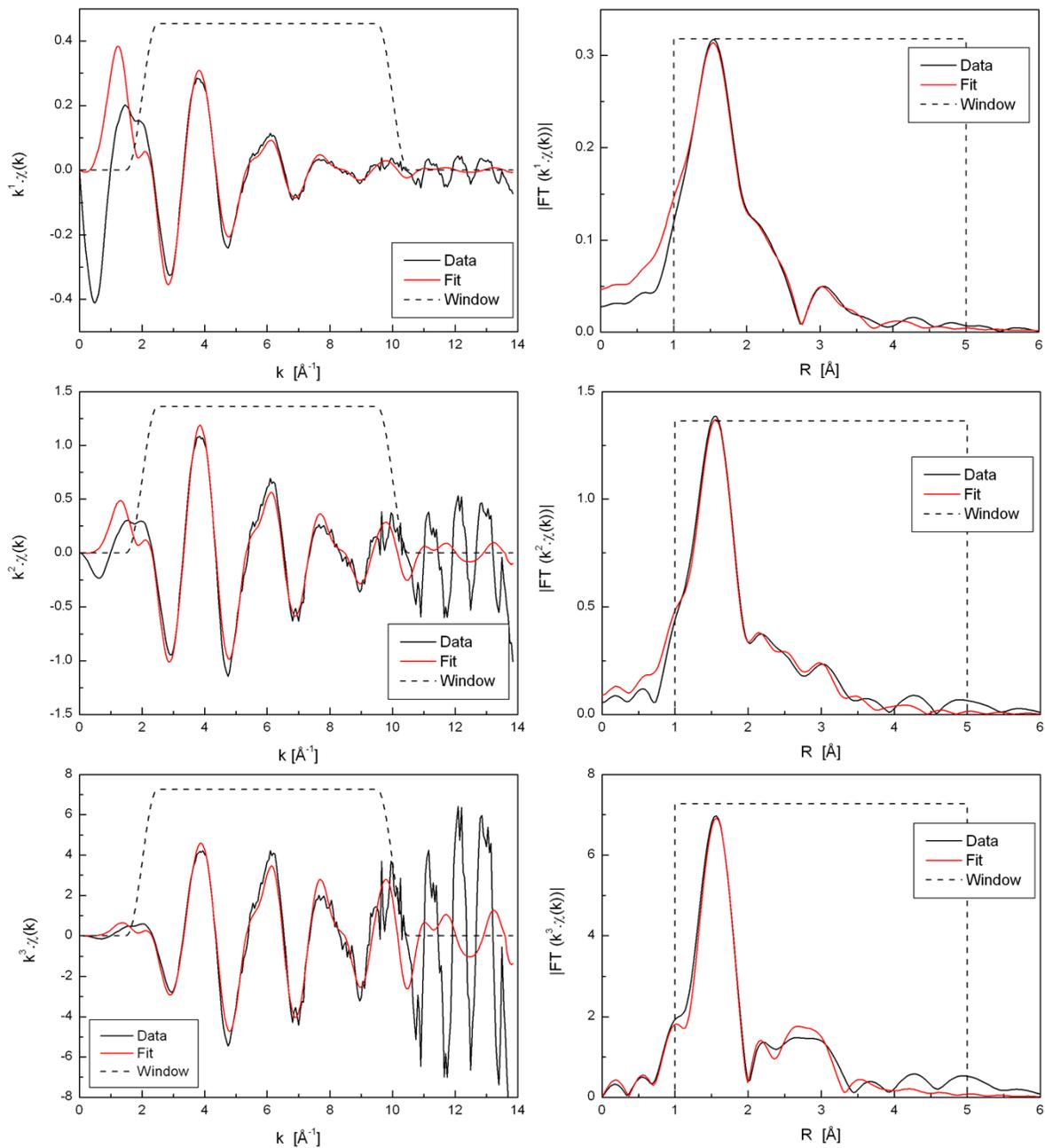
**Figure S4.** Ni-NCO 2:1 KOCN:Ni<sup>2+</sup> mole ratio model solution in DMSO ('Sample 4'), fitted using a single shell model. EXAFS data (black lines) and fits (red lines) in k-space (left) and R-space (right) for various k-weightings: k<sup>1</sup> (top), k<sup>2</sup> (middle), k<sup>3</sup> (bottom). The data ranges used for fitting are shown by the window functions (black dashed lines).
