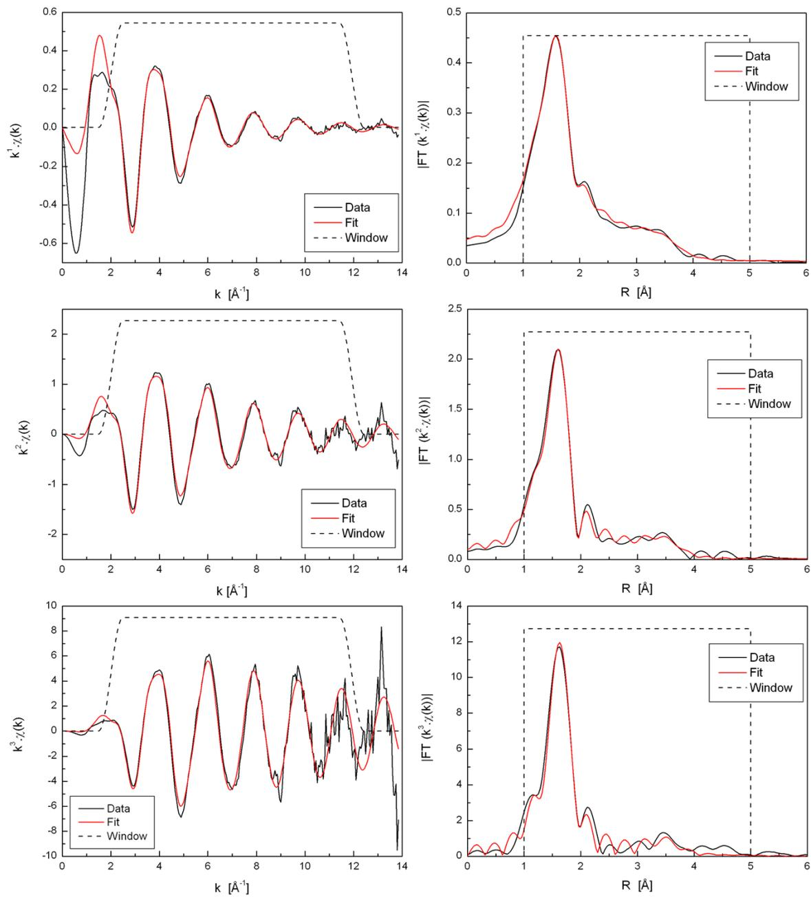
**Figure S2.**  $\text{Ni}(\text{NO}_3)_2$  in  $\text{H}_2\text{O}$  ('Sample 2') EXAFS data (black lines) and fits (red lines) in  $k$ -space (left) and  $R$ -space (right) for various  $k$ -weightings:  $k^1$  (top),  $k^2$  (middle),  $k^3$  (bottom). The data ranges used for fitting are shown by the window functions (black dashed lines).
