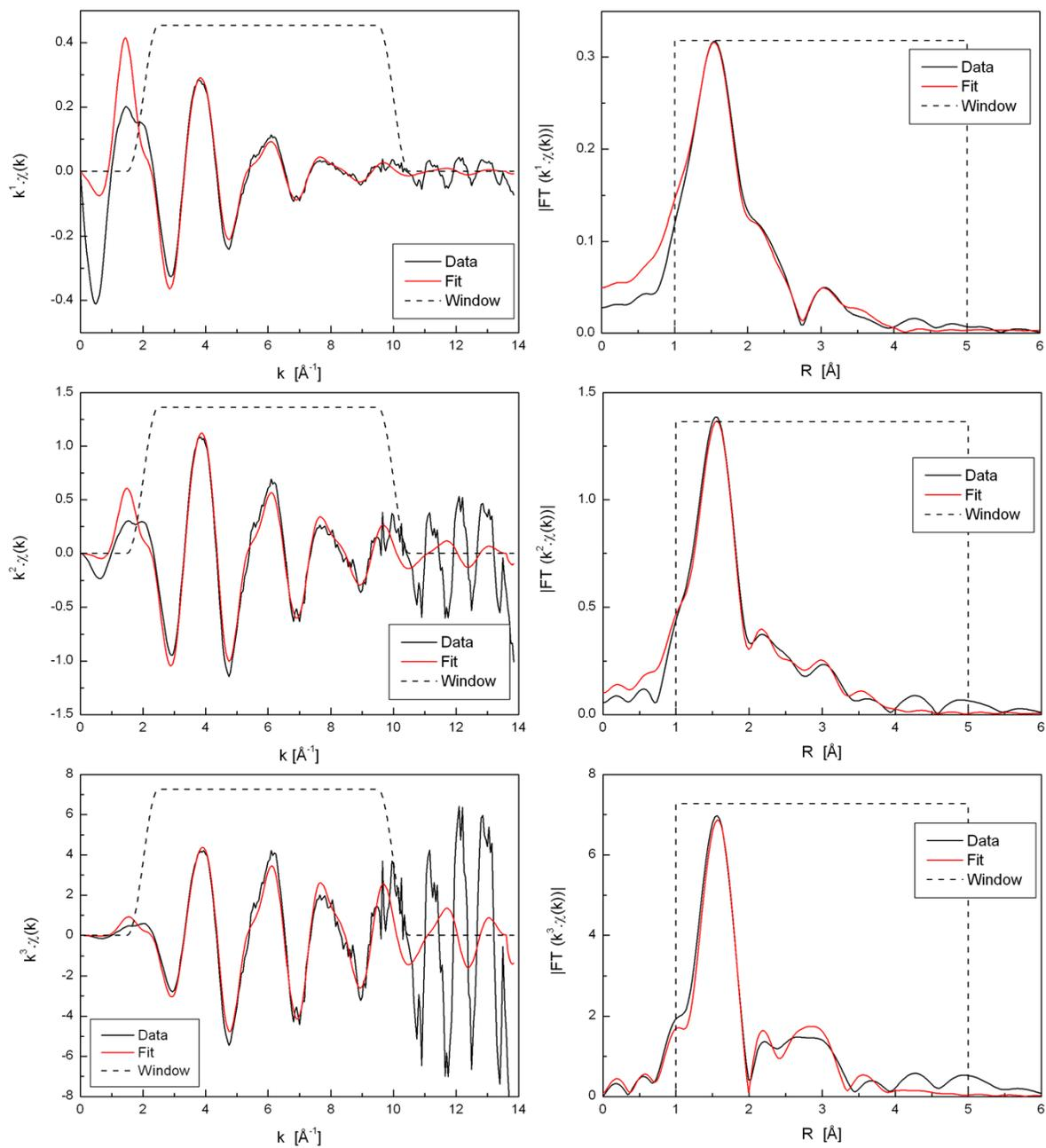
**Figure S8.** Ni-NCO 2:1 KOCN:Ni<sup>2+</sup> mole ratio model solution in DMSO ('Sample 4'), fitted using a single shell model for DMSO and a multiple-scattering model for OCN. EXAFS data (black lines) and fits (red lines) in k-space (left) and R-space (right) for various k-weightings: k<sup>1</sup> (top), k<sup>2</sup> (middle), k<sup>3</sup> (bottom). The data ranges used for fitting are shown by the window functions (black dashed lines).
