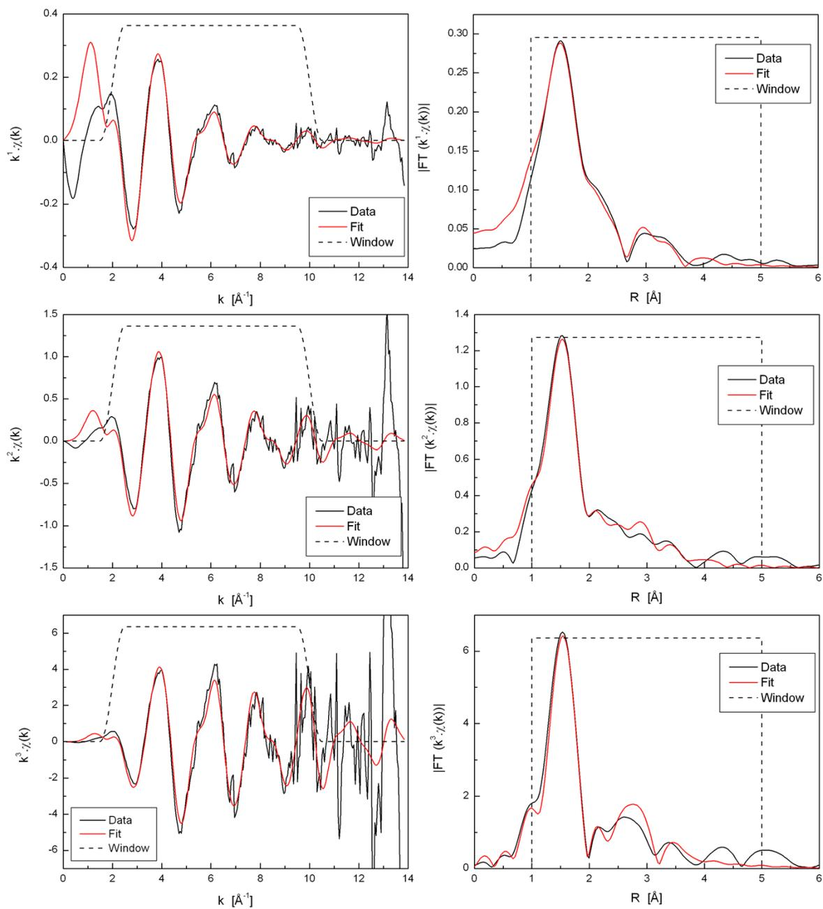
**Figure S7.** Ni-NCO electrochemically generated solution in DMSO ('Sample 7'), fitted using a single shell model. EXAFS data (black lines) and fits (red lines) in k-space (left) and R-space (right) for various k-weightings:  $k^1$  (top),  $k^2$  (middle),  $k^3$  (bottom). The data ranges used for fitting are shown by the window functions (black dashed lines).
