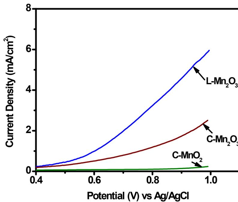
Fig. S6: LSV of L-Mn<sub>2</sub>O<sub>3</sub>, C-Mn<sub>2</sub>O<sub>3</sub> and C-MnO<sub>2</sub> recorded in 1M NaOH at scan rate of 5 mV/sec.
