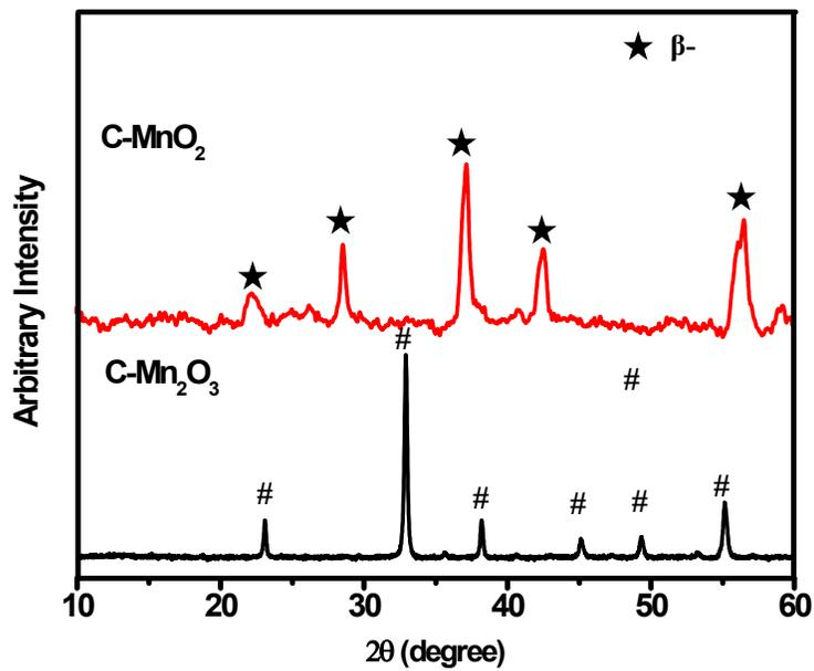
**Fig. S4:** PXRD patterns obtained for C-MnO<sub>2</sub> and C-Mn<sub>2</sub>O<sub>3</sub>, where ★ refers to the peaks corresponding to the β-MnO<sub>2</sub> phase, and # refers to the peak corresponding to pure Mn<sub>2</sub>O<sub>3</sub> phase.
