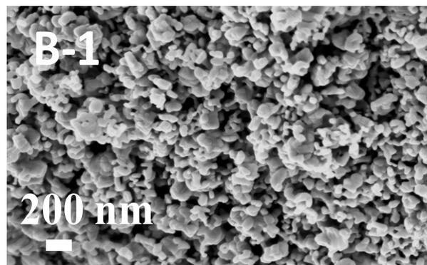
Fig. S5: Low magnification SEM images of the C-MnO<sub>2</sub> (A), low and high magnification image of C-Mn<sub>2</sub>O<sub>3</sub> (B, B-1).
