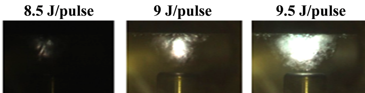
Fig. S1 Discharge photographs for capacitor energy of <10 J.
