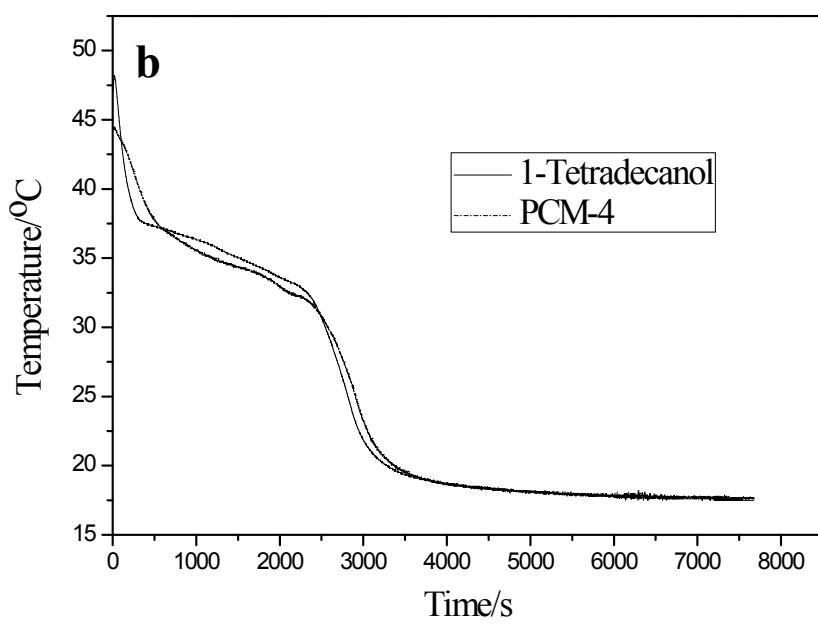
Fig. S12 Endothermic (a) and Exothermic (b) curves of 1-tetradecanol and PCM-4
