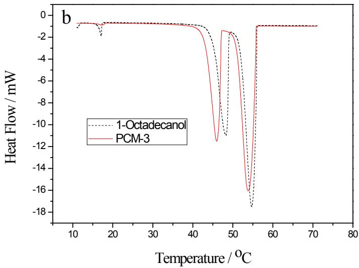
Fig. S3 DSC curves of 1-octadecanol and PCM-3; (a) melting process and (b) solidifying process
