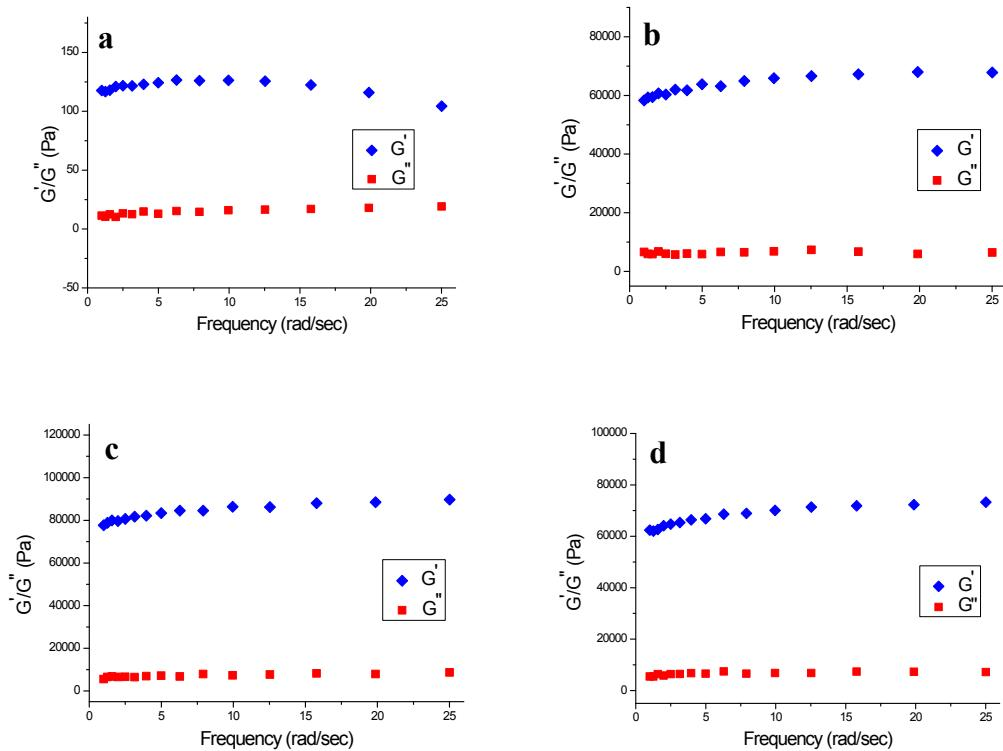
Fig. S5 Frequency dependence of the dynamic storage moduli  $G'$  and loss moduli  $G''$  of different composite PCMs: (a) PCM-1; (b) PCM-2; (c) PCM-3; (d) PCM-4.
