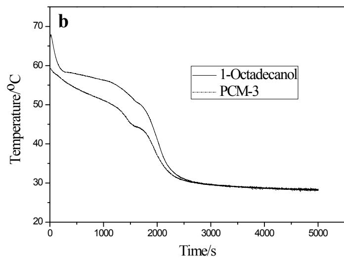
Fig. S11 Endothermic (a) and Exothermic (b) curves of 1-octadecanol and PCM-3
