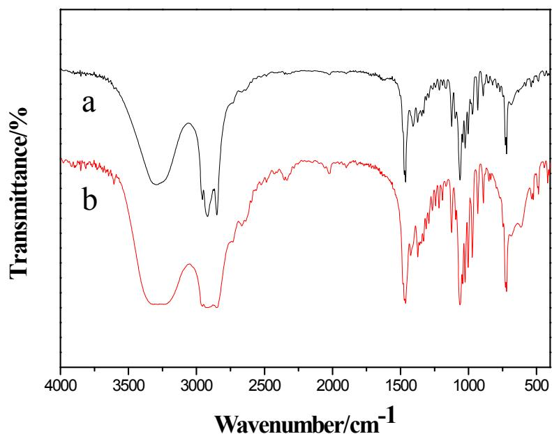
Fig. S8 FTIR spectra of (a) 1-tetradecanol, (b) PCM-4
