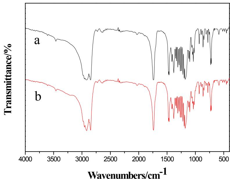
Fig. S6 FTIR spectra of (a) ethyl palmitate, (b) PCM-2
