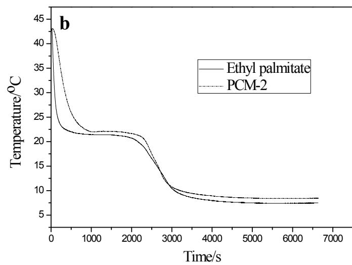
Fig. S10 Endothermic (a) and Exothermic (b) curves of ethyl palmitate and PCM-2
