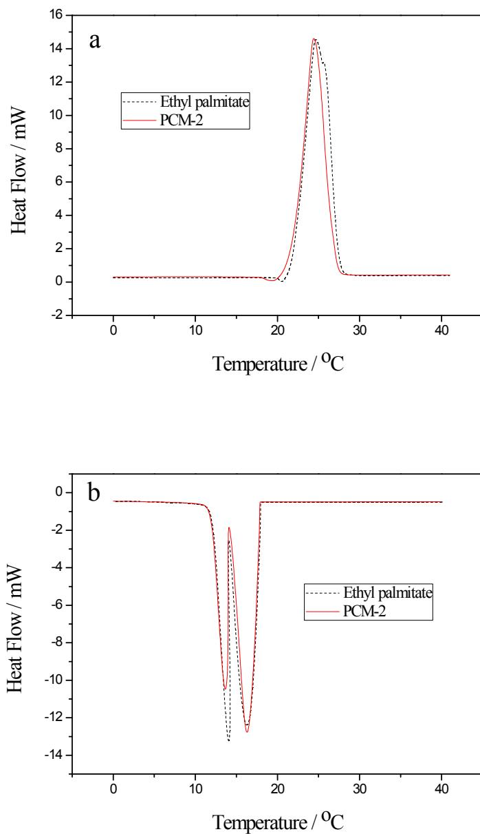
Fig. S2 DSC curves of ethyl palmitate and PCM-2: (a) melting process and (b) solidifying process
