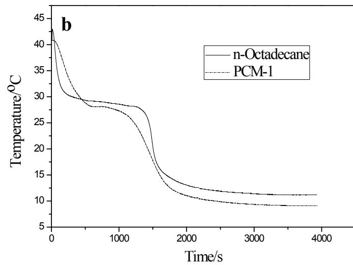
Fig. S9 Endothermic (a) and Exothermic (b) curves of n-octadecane and PCM-1
