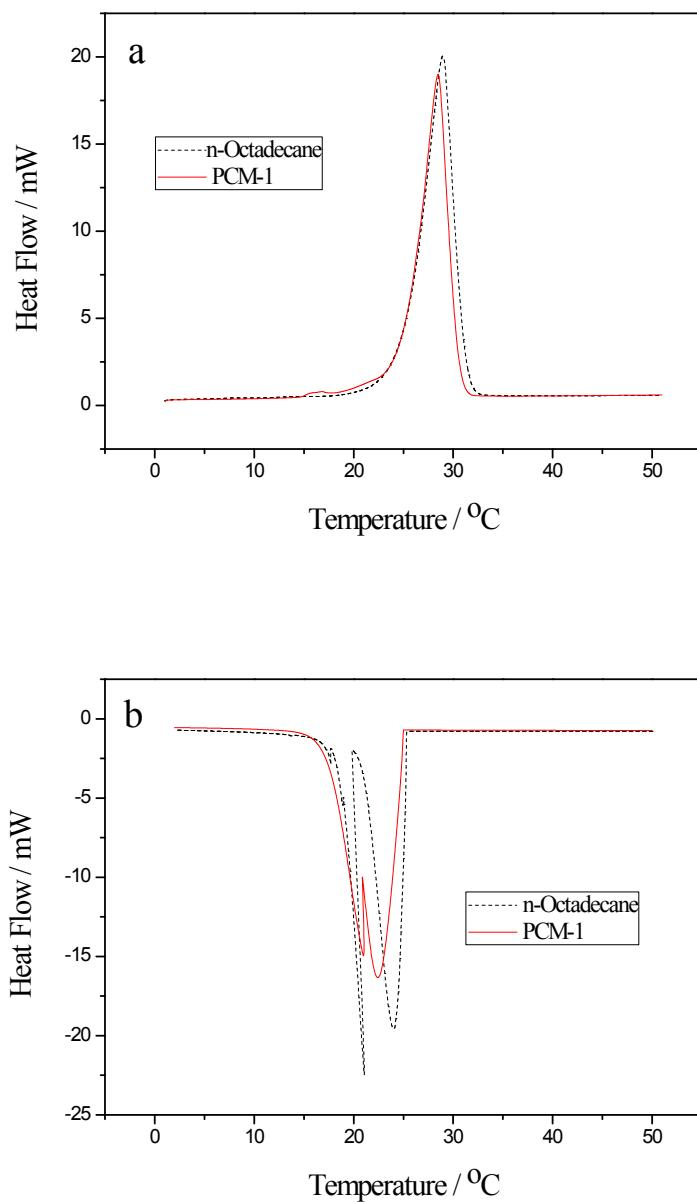
Fig. S1 DSC curves of n-octadecane and PCM-1: (a) melting process and (b) solidifying process
