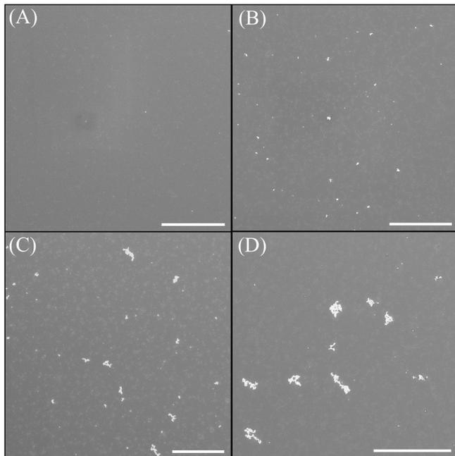
**Figure S1.** SEM images of aggregation of Au NPs with increasing  $\text{Mg}^{2+}$  concentration and hybridization time.  $\text{Mg}^{2+}$  concentrations and hybridization times for the samples were: (A) 40 mM and 10 min, (B) 70 mM and 30 min, (C) 100 mM and 90 min, and (D) 130 mM and 90 min. Scale bars are 5  $\mu\text{m}$ .
