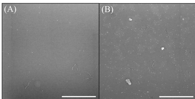
**Figure S2.** Background Au NP deposition with increasing Au NP concentration. SEM images of samples with (A) 4 nM and (B) 40 nM Au NPs. Scale bars are 500 nm.
