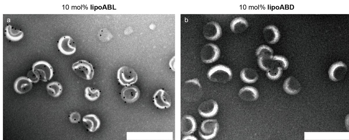
**Fig. S2** TEM images (negative stained with 2% uranyl acetate) of vesicles prepared from (a)  $A_3BL + ABD + \text{lipoABL}$  (0.4/0.5/0.1) and (b)  $A_3BL + ABD + \text{lipoABD}$  (0.5/0.4/0.1) in milliQ upon a heat treatment at 90 °C for 1 h. An aliquot of a 10 nm AuNP suspension was added to the vesicles on the TEM grid. Bars indicate 200 nm.
