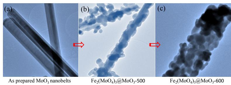
**Scheme. S1.** Schematic illustration of the morphology evolution process of  $\text{MoO}_3$  nanobelts. (a)  $\text{MoO}_3$  nanobelts; (b) FM-500 nanowires and (c) hollow hierarchical structural FM-600.
