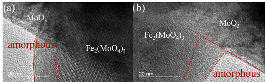
**Fig. S6** Two typical HRTEM images of FM-500 nanowires (a)-(b), showing the location position relationship of  $\text{MoO}_3$  nanobelts,  $\text{Fe}_2(\text{MoO}_4)_3$  nanoparticles and amorphous layer.
