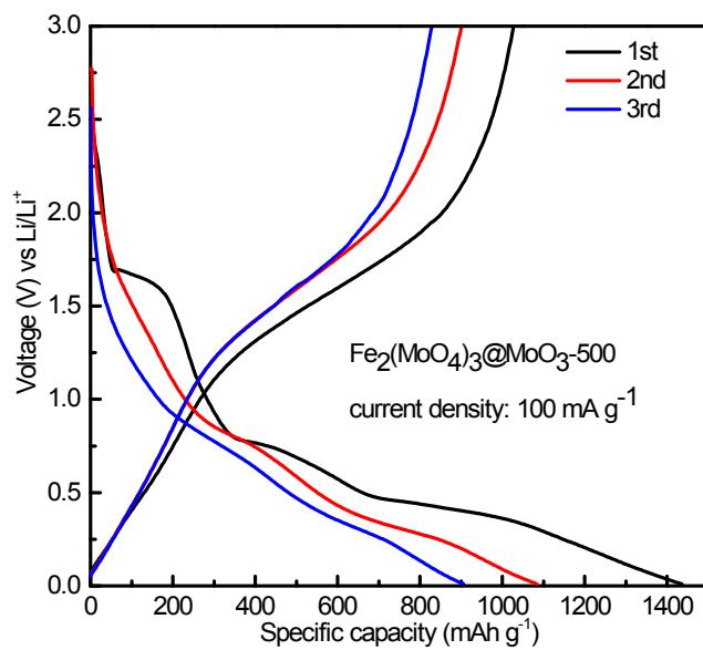
**Fig. S8** The voltage profiles plotted for the first three charge-discharge cycles of the FM-500 nanobelts electrode at a current density of  $100 \text{ mA g}^{-1}$ .
