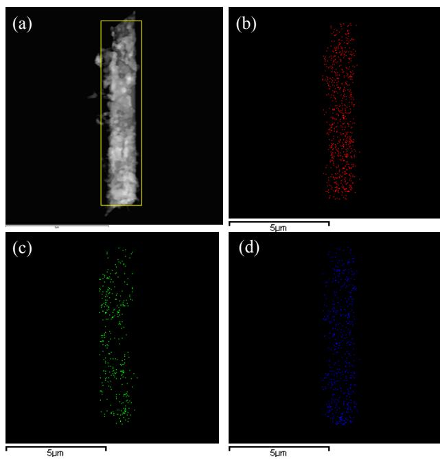
**Fig. S3** (a) STEM image of an individual FM-500 nanobelts and corresponding EDX elemental mapping of (b) Fe, (c) Mo and (d) O, respectively.
