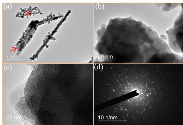
**Fig.S2** A typical TEM images of FM-600 (a)-(b), (c) HRTEM images of an individual nanoparticles composites and (d) the corresponding SAED. The two red arrow indicate some hollow hierarchical heterostructures.
