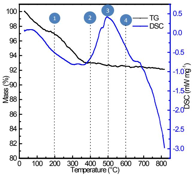
**Fig. S1.** TG-DSC pattern of  $\text{MoO}_3$  nanobelts soaked in  $\text{FeCl}_3 \cdot 6\text{H}_2\text{O}$  via hydrothermal treatment at 90  $^{\circ}\text{C}$  for 6 h.
