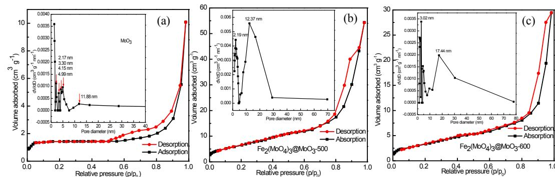
**Fig. S7.** Nitrogen adsorption and desorption isotherms and pore-size distribution curves (inset) of the MoO<sub>3</sub> nanobelts (a), FM-500 nanowires (b), and MF-600 (c) sample. According to BJH method, a maximum of the pore size distribution taken from the description branch.
