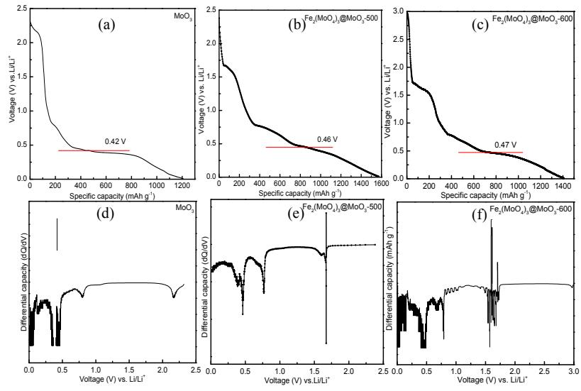
**Fig. S4** The charge-discharge profiles of the MoO<sub>3</sub> nanobelts, FM-500, and FM-600 (a)-(c) and their corresponding dQ/dV profiles (d)-(f).
