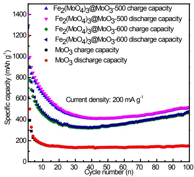
**Fig. S5** The cycle performance of the  $\text{MoO}_3$  nanobelts, FM-500 nanowires and FM-600 at  $200 \text{ mA g}^{-1}$ .
