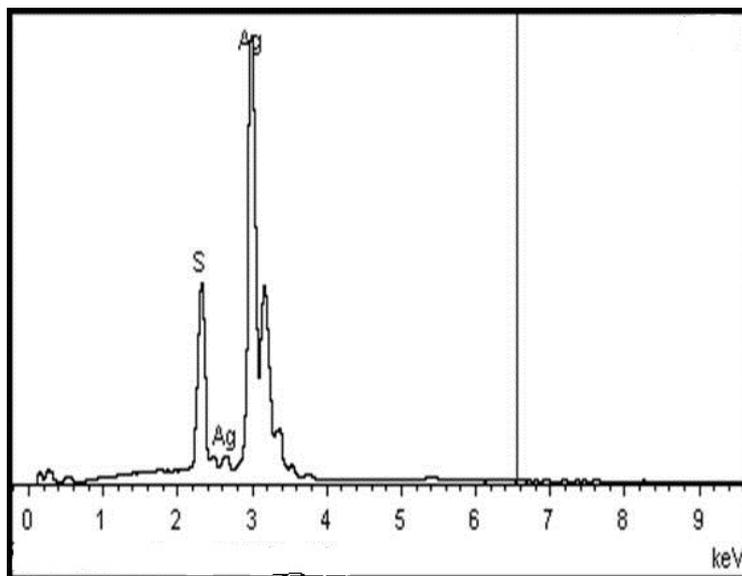
Fig. S1 EDS result of  $\text{Ag}_2\text{S}$
