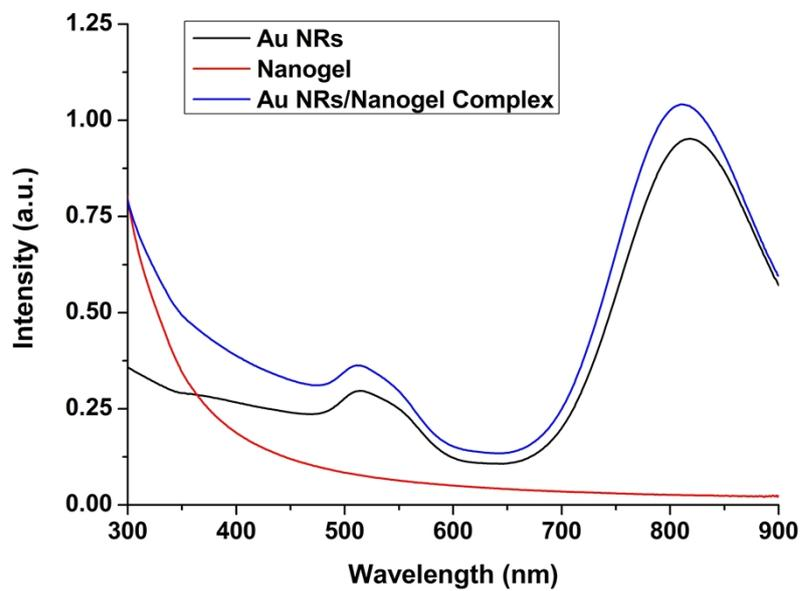
**Fig. S2** UV-Vis spectra of Au nanorods and heparin-PEI-LA/Au NRs nanogels complexes at room temperature. The concentration of Au nanorod in each group was all 0.5 nM.
