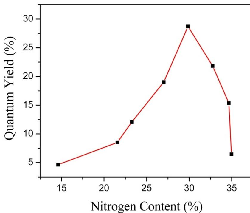
**Fig. S5.** Effect of the nitrogen's content in CDs on the quantum yield of CDs.
