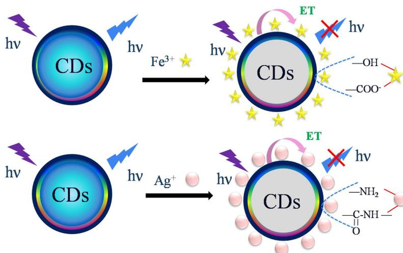
**Fig. S10.** Sensing principle of the CDs based probe for  $\text{Fe}^{3+}$  and  $\text{Ag}^+$ .
