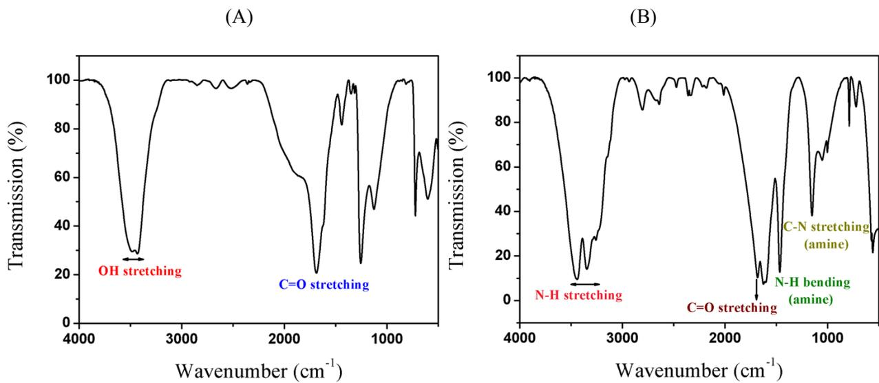
**Fig. S7.** FTIR spectra of (A) oxalic acid and (B) urea.
