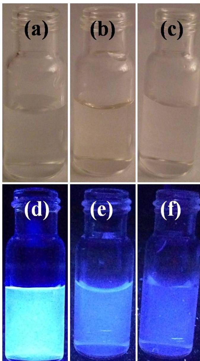
**Fig. S11.** Photographic images of CDs (0.50 mg/mL) before and after adding  $\text{Fe}^{3+}$  (0.20 mM) and  $\text{Ag}^+$  (0.20 mM) under daylight (a, b and c) and UV irradiation (d, e and f), respectively.
