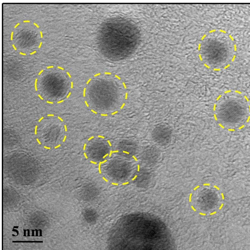
**Fig. S3.** HRTEM image of CDs. The yellow circles highlight examples of CDs with obvious lattice spacings.
