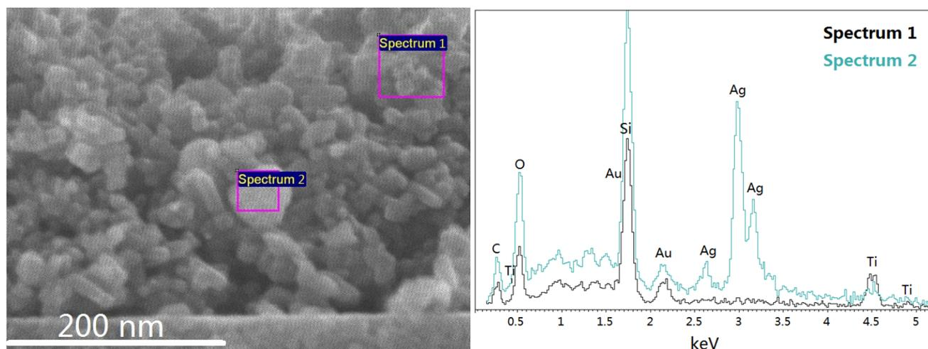
**Fig. S1** Energy dispersive spectroscopy (EDS) spectra of popcorn nanoparticle (NP) and mesoporous TiO<sub>2</sub>. Spectrum 1 and 2 represents the EDS spectra of mesoporous TiO<sub>2</sub> and popcorn NP, respectively. The C peak in both spectra is due to the carrier and clamp used in scanning electron microscope (SEM) measurements, while the Si peak comes from the silicon substrate on which the samples are prepared just for SEM measurement.
