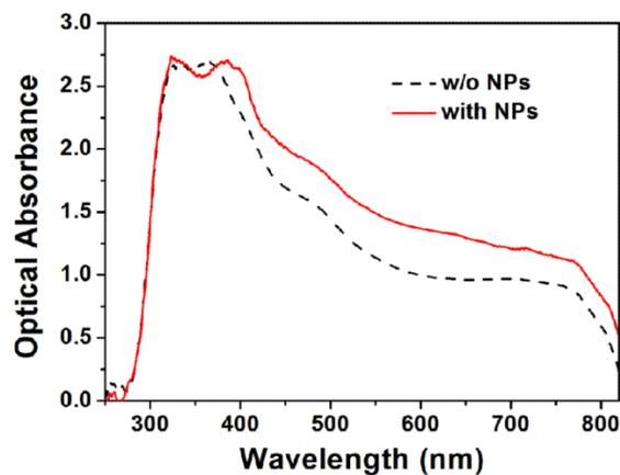
**Fig. S2** Optical absorption of thinner perovskite films on mesoporous TiO<sub>2</sub> framework with and without popcorn NPs, respectively.
