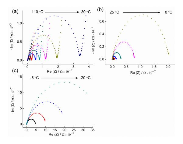
**Figure S1**. Impedance spectra for  $\alpha$ -LiZr<sub>2</sub>(PO<sub>4</sub>)<sub>3</sub> measured using Au electrodes (frequency range from 10 MHz to 1 Hz; 20 mV amplitude) in the temperature range 20 110 °C.
