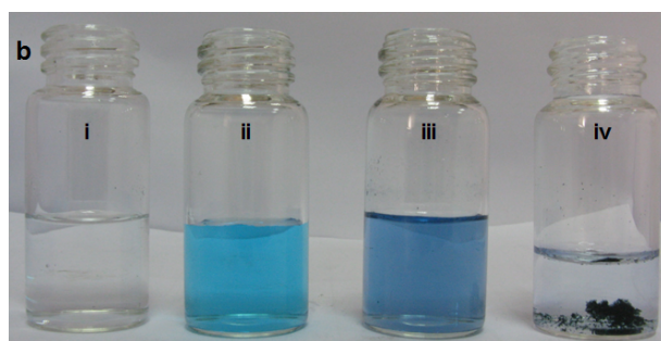
Fig S6. (a) Vigorous stirring (1000 rpm) for 30s (b) and then kept quietly for 2 days. (i) D.I. water; (ii) MB (5 ppm); (iii) MB (5 ppm) and GO (15 ppm), without NaCl; (iv) MB (5 ppm) and GO (15 ppm) with NaCl (5 mM).
