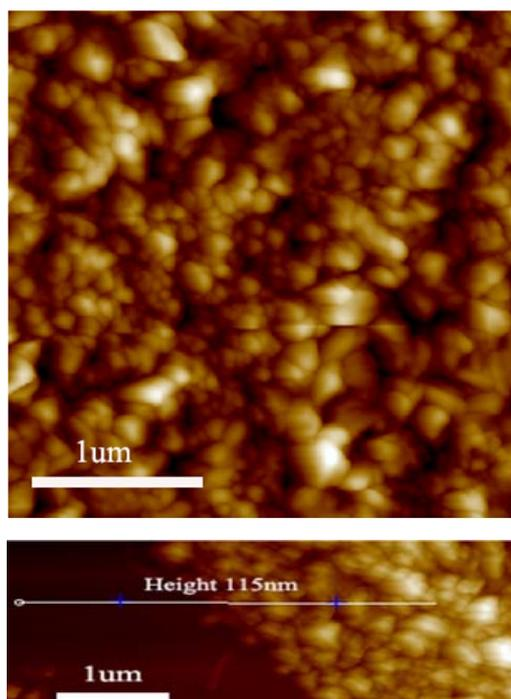
**Fig. S19** AFM topography image of spin-coated film of **4e** on OTS-modified SiO<sub>2</sub>/Si substrates. The concentration of the stock solution in CH<sub>2</sub>Cl<sub>2</sub> was 12 mg/mL.
