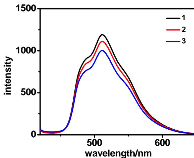
**Fig. S18** Fluorescence spectra of **4e** in the spin-coated films prepared from the different concentrations of the stock solutions in CH<sub>2</sub>Cl<sub>2</sub> at room temperature and same rotate speed. The concentrations of the stock solutions were 10 mg/mL (1), 12 mg/mL (2), and 15 mg/mL (3), respectively.  $\lambda_{\text{ex}} = 407$  nm.
