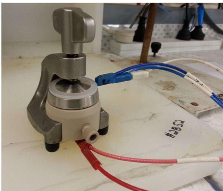
Figure S1. Digital photo of electric double layer capacitor (EDLC) constructed with N-doped graphene.
