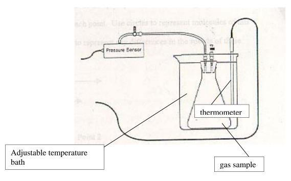
Assume that this device could be used to take pressure readings on gas samples for a range of gas temperatures between 25.0 °C and 100.0 °C. Assume gas samples behave ideally. Question 1: What will happen if the gas is heated? Please explain your answer. *Answer. The measured pressure will increase as the gas is heated.*
