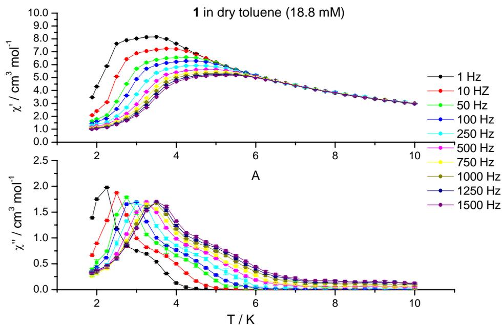
Figure ESI 3. Temperature dependence of the in-phase ( $\chi'$ ) and out-of-phase ( $\chi''$ ) a.c. molar magnetic susceptibility of an 18.8 mM solution of **1** in dry toluene, in the temperature range 2 to 10 K and for a.c. fields oscillating at frequencies in the range 1 to 1500 Hz.
