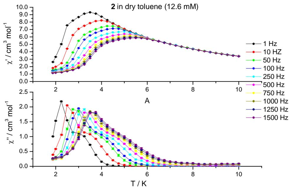
Figure ESI 4. Temperature dependence of the in-phase ( $\chi'$ ) and out-of-phase ( $\chi''$ ) a.c. molar magnetic susceptibility of a 12.6 mM solution of **2** in dry toluene, in the temperature range 2 to 10 K and for a.c. fields oscillating at frequencies in the range 1 to 1500 Hz.
