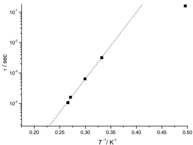
Figure ESI 7. Relaxation times  $\tau$  for a 33.1 mM solution of  $[\text{Mn}_3\text{O}(\text{Et-sao})_3(\text{MeOH})_3](\text{ClO}_4)$  in methanol. The dot line represents the fit of the experimental data to the Arrhenius model of equation (1). This yielded:  $\tau_0 = 1.7 \cdot 10^{-10}$  sec and  $U_{\text{eff}} = 50.4$  K.
