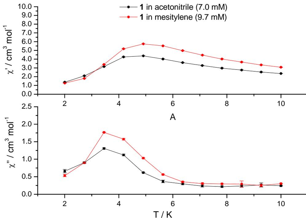
Figure ESI 5. Temperature dependence of the in-phase ( $\chi'$ ) and out-of-phase ( $\chi''$ ) a.c. molar magnetic susceptibility of a 7.0 mM and a 9.7 mM solutions of **1** in acetonitrile and mesitylene, respectively, in the temperature range 2 to 10 K and for an a.c. field oscillating at a frequency of 1500 Hz.
