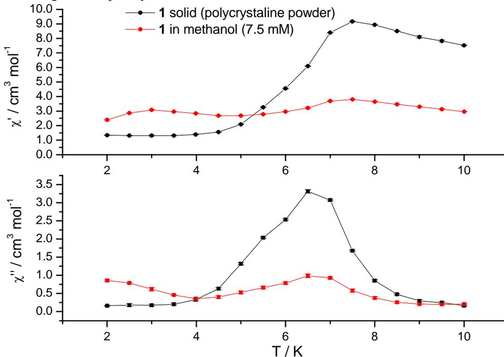
Figure ESI 6. Temperature dependence of the in-phase ( $\chi'$ ) and out-of-phase ( $\chi''$ ) a.c. molar magnetic susceptibility of a 7.6 mM solution of **1** in methanol and of **1** as polycrystalline powder in the temperature range 2 to 10 K and for an a.c. field oscillating at a frequency of 1500 Hz.
