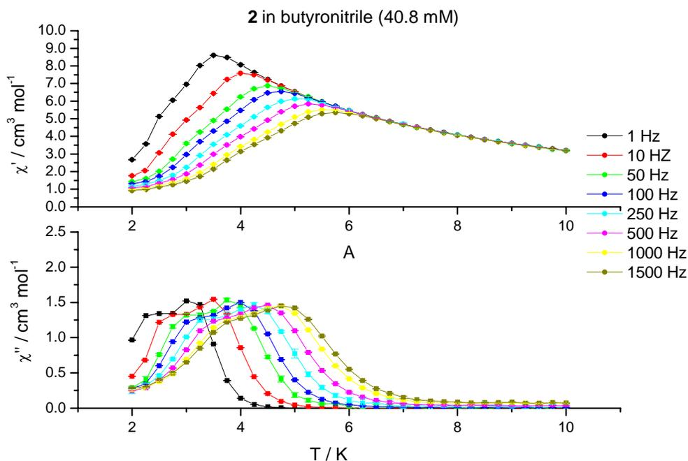
Figure ESI 2. Temperature dependence of the in-phase ( $\chi'$ ) and out-of-phase ( $\chi''$ ) a.c. molar magnetic susceptibility of a 40.8 mM solution of **2** in butyronitrile, in the temperature range 2 to 10 K and for a.c. fields oscillating at frequencies in the range 1 to 1500 Hz.
