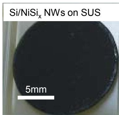
Figure S2 A photograph of the a -Si/NiSi x NW grown on the whole SUS substrate of 15 Φ diameter.
