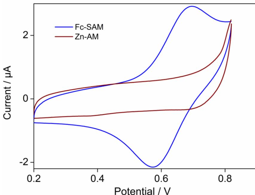
**Figure S6.** CV plots of SAM-Fc (blue) and Zn-AM (brown) in 0.73 M NaClO<sub>4</sub>/0.09 M Tris (PH=7.51) under the scan rate 0.1 V·s<sup>-1</sup>.
