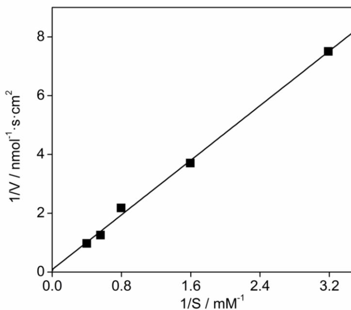
**Figure S11.** The Lineweaver-Burk plot of Zn-AM in *p*-NPA assay.  $1/V$  represents the reciprocal of catalytic rate  $V$ , while  $1/S$  represents the reciprocal of the *p*-NPA concentration. The fitting equation is  $(1/V) = 0.08554 + 2.32426 (1/S)$ .
