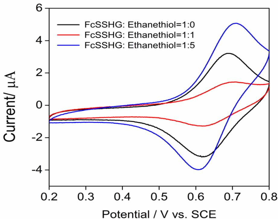
**Figure S7.** The representative CV plots for SAM-Fc, SAM2-Fc and SAM3-Fc are obtained in 0.73 M NaClO<sub>4</sub>/0.09 M Tris (PH=7.51) under the scan rate 0.1 V·s<sup>-1</sup>. The film SAM2-Fc incubated in the 1:1 (FcSSHG:Ethanethiol) mixed solution and the film SAM3-Fc incubated in the 1:5 (FcSSHG:Ethanethiol) mixed solution.
