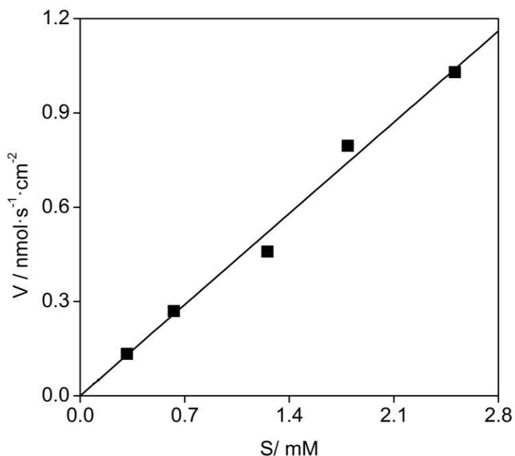
**Figure S10.** Effect of the *p*-NPA concentration on the activity of Zn-AM. The horizontal axis represents the original *p*-NPA concentration, and the vertical axis represents the catalytic rate over 180 s catalysis.
