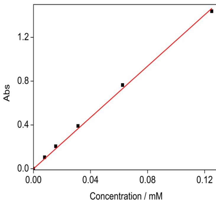
**Figure S9.** Calibration plot of *p*-NP in 0.73 M NaClO<sub>4</sub>/0.09 M Tris buffer solution (pH=7.51) in presence of 9% (V/V) CH<sub>3</sub>CN. The black spots represented the absorbance of *p*-NP at 400 nm recorded at 0, 0.0078, 0.0156, 0.0313, 0.0625 and 0.125 mM, respectively. The red trace was the fitting line, corresponding to the equation  $y=11.71536x$ .
