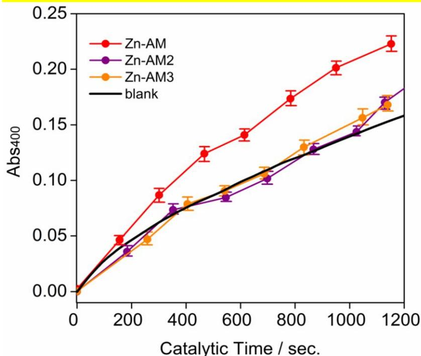
**Figure S12.** The UV kinetics plots of *p*-NPA hydrolysis at the presence of Zn-AM, Zn-AM2 and Zn-AM3, observed through the absorbance at 400 nm in 0.73 M NaClO<sub>4</sub>/0.09 M Tris (pH =7.51) containing 9% (V/V) acetonitrile, 25 °C. The orange line represents the blank affected by the self-hydrolysis of *p*-NPA.
