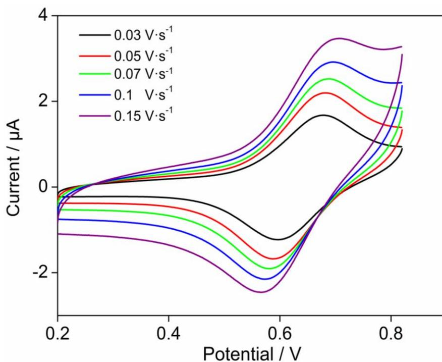
**Figure S4.** CV plots of SAM-Fc film under different scan rates in 0.73 M NaClO<sub>4</sub>/0.09 M Tris (pH=7.51).
