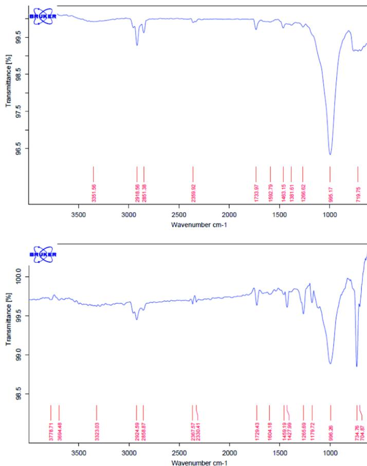
**Figure S5.** Fourier Transform Infrared (FTIR) spectra of exTTFaunPs (top) and exTTFaunPs•C<sub>60</sub> (bottom).
