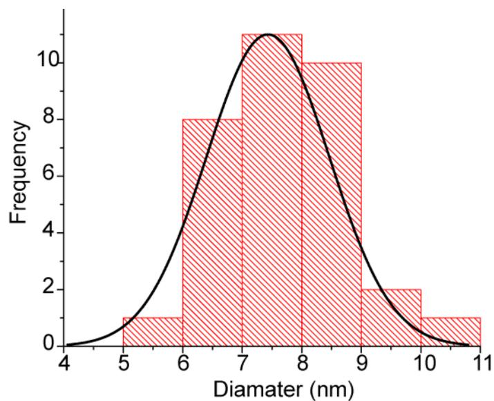
**Figure S1.** Statistical analysis of the diameter of the exTTF AuNPs.
