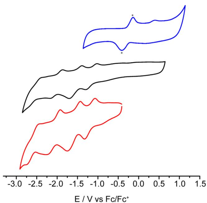
**Figure S6.** Cyclic voltammograms of exTTFaunPs (blue), exTTFaunPs•C<sub>60</sub> (black) and C<sub>60</sub> (red).
