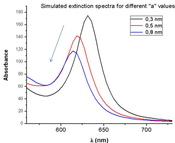
Figure S3. Model for the computational simulation of the impact of the disaggregation process on their UV-vis spectra, and results of the simulation. For three dimensional ensembles the extinction band of coupled free electron oscillation will be broader as in case of Figure 1 (main text).
