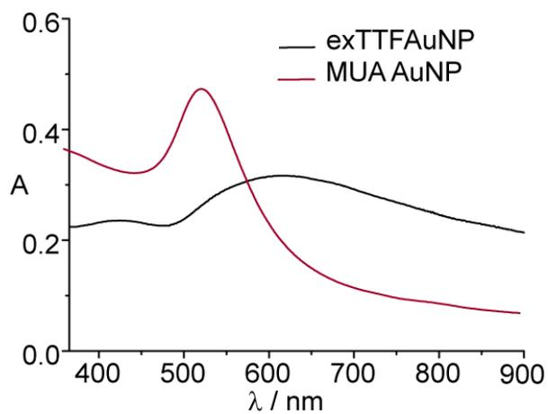
**Figure S2.** UV-vis spectra of exTTF AuNP and MUA AuNP in o-DCB at room temperature.
