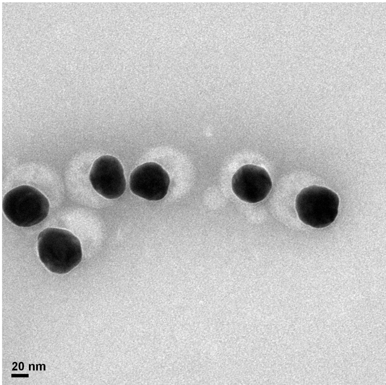
**Figure S6.** TEM image of the Au@vesicle NPs,  $d_{\text{Au}} = 40$  nm, [SDS] = 2.5 mM,  $t = 1.5$  h (large-area view of Figure 3c).
