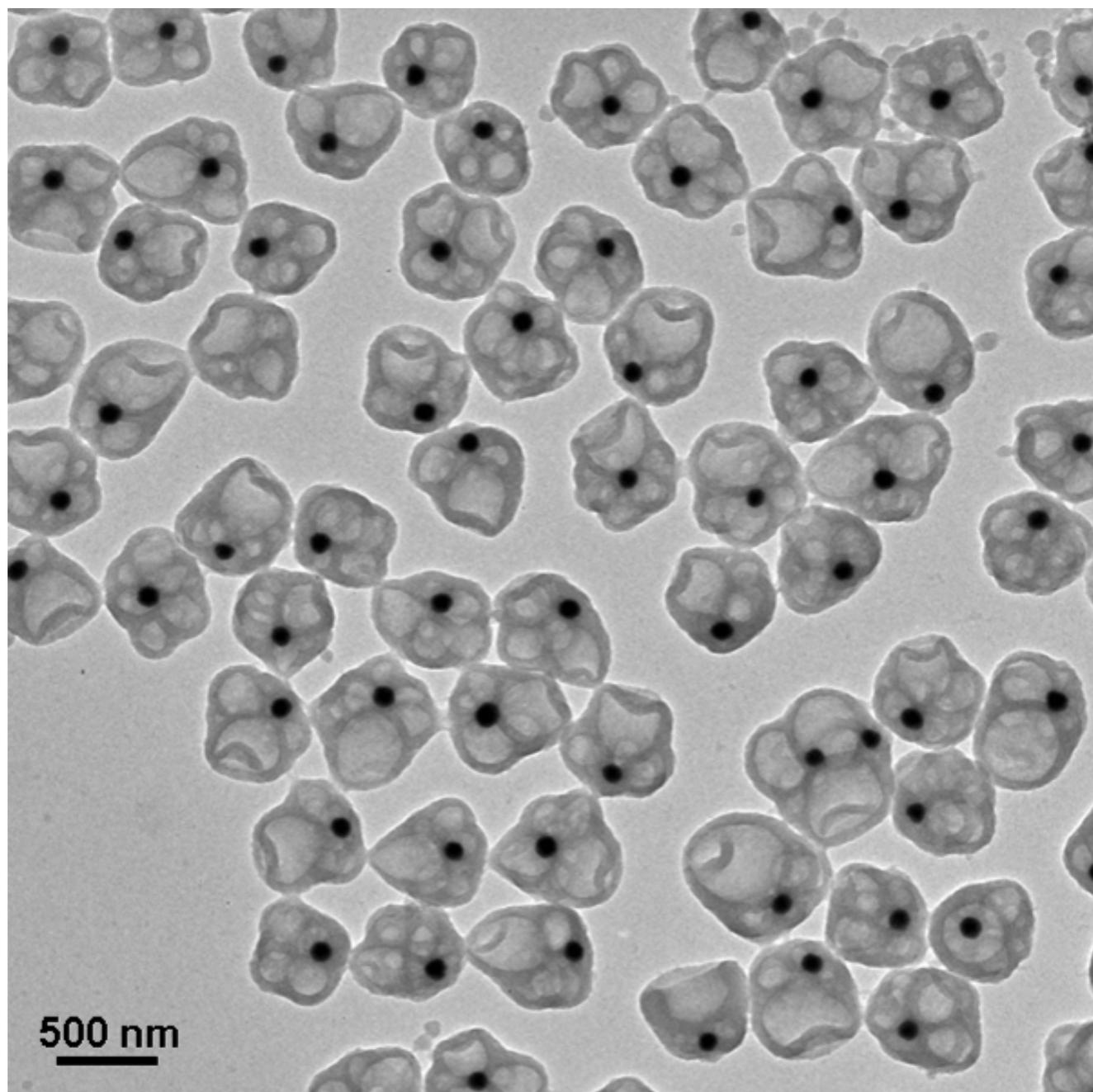
**Figure S4.** TEM image of the Au@vesicle NPs,  $d_{\text{Au}} = 80$  nm,  $[\text{SDS}] = 2.5$  mM, (large-area view of Figure 3b).
