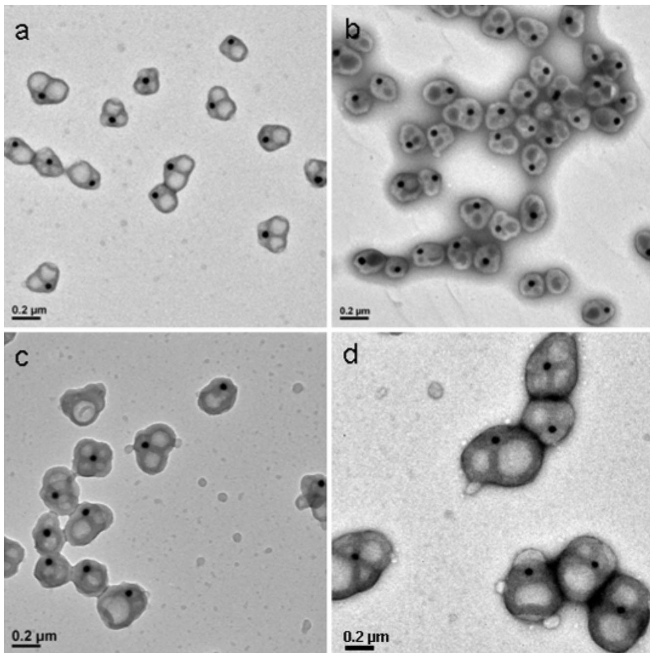
**Figure S14.** TEM images of (a) Au@vesicle NPs, (b) sample a after incubating in THF, (c) sample b after the 2nd growth cycle, and (d) after the 3rd growth cycle, respectively,  $d_{\text{Au}} = 40$  nm,  $[\text{SDS}] = 2.5$  mM.
