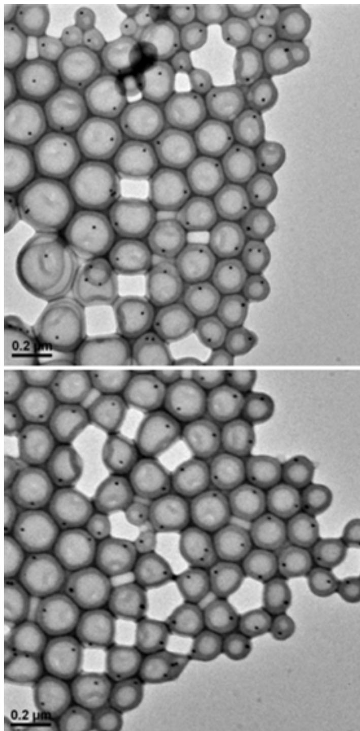
**Figure S3.** TEM images of the Au@vesicle NPs,  $d_{\text{Au}} = 18 \text{ nm}$ ,  $[\text{SDS}] = 1 \text{ mM}$ , (large-area view of Figure 3a). Most (98% out of 132 nanocomposites) of the vesicles have only one cavity, though some of the AuNPs were aggregated.
