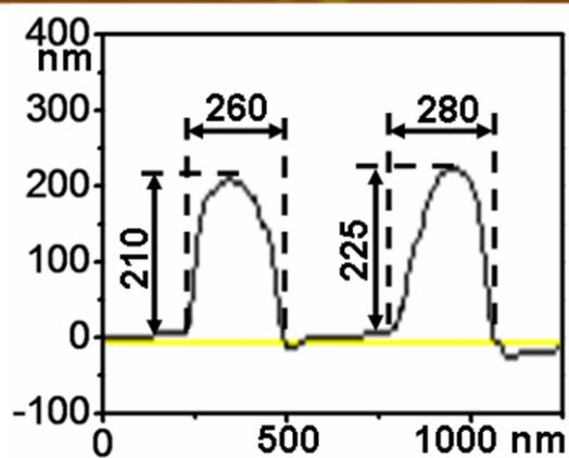
**Figure S2.** AFM image of Au@vesicle NPs,  $d_{\text{Au}} = 40$  nm,  $[\text{SDS}] = 2.5$  mM,  $t = 12$  h, and the cross-sectional height profile along the white line is shown at the bottom.
