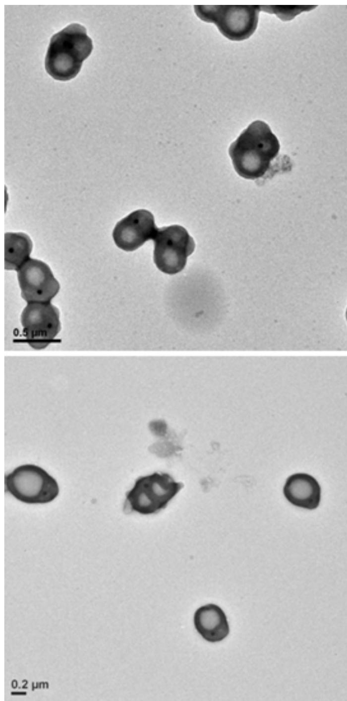
**Figure S13.** TEM images of Au@vesicle NPs after 3 growth cycles, [SDS] = 2.5 mM. The average diameter of the cavity is 210 nm and the average thickness of the cavity wall is 65 nm calculated from 11 vesicles.
