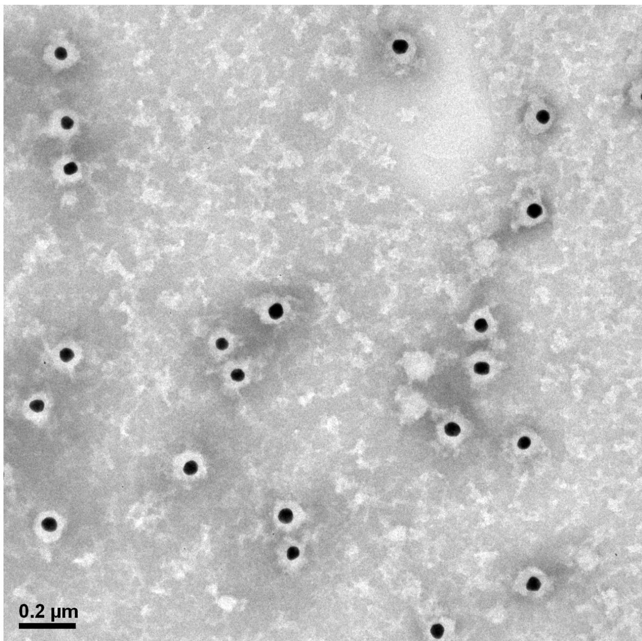
**Figure S8.** TEM image of the Au@PTh core-shell NPs,  $d_{\text{Au}} = 40$  nm, [SDS] = 5 mM,  $t = 12$  h, before purification. The polymer NPs in the dark brown supernatant can be identified as the white particles.
