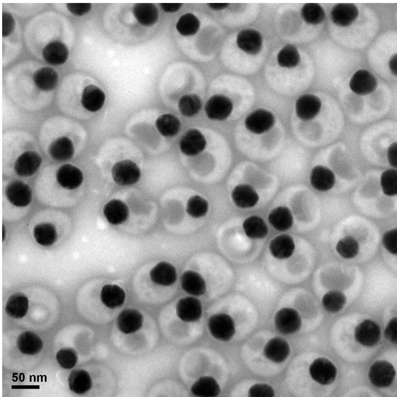
**Figure S7.** TEM image of the Au@vesicle NPs,  $d_{\text{Au}} = 40$  nm, [SDS] = 2.5 mM,  $t = 2.5$  h (large-area view of Figure 3d).
