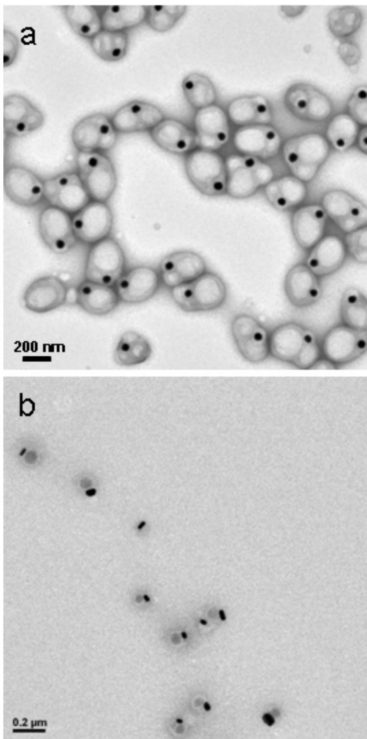
**Figure S5.** TEM images of (a) Ag@vesicle NPs,  $d_{\text{Ag}} = 50$  nm, [SDS] = 2.5 mM,  $t = 12$  h, and (b) AuNR@vesicle NPs,  $d_{\text{AuNR}} = 62$  nm,  $l_{\text{AuNR}} = 30$  nm, [SDS] = 2.5 mM,  $t = 12$  h.
