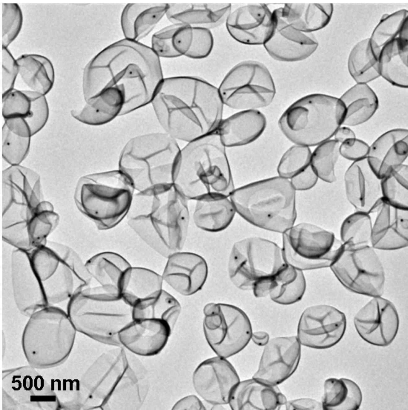
**Figure S9.** TEM image of the Au@vesicle NPs,  $d_{\text{Au}} = 40$  nm,  $[\text{SDS}] = 0.8$  mM,  $t = 12$  h (large-area view of Figure 3f).
