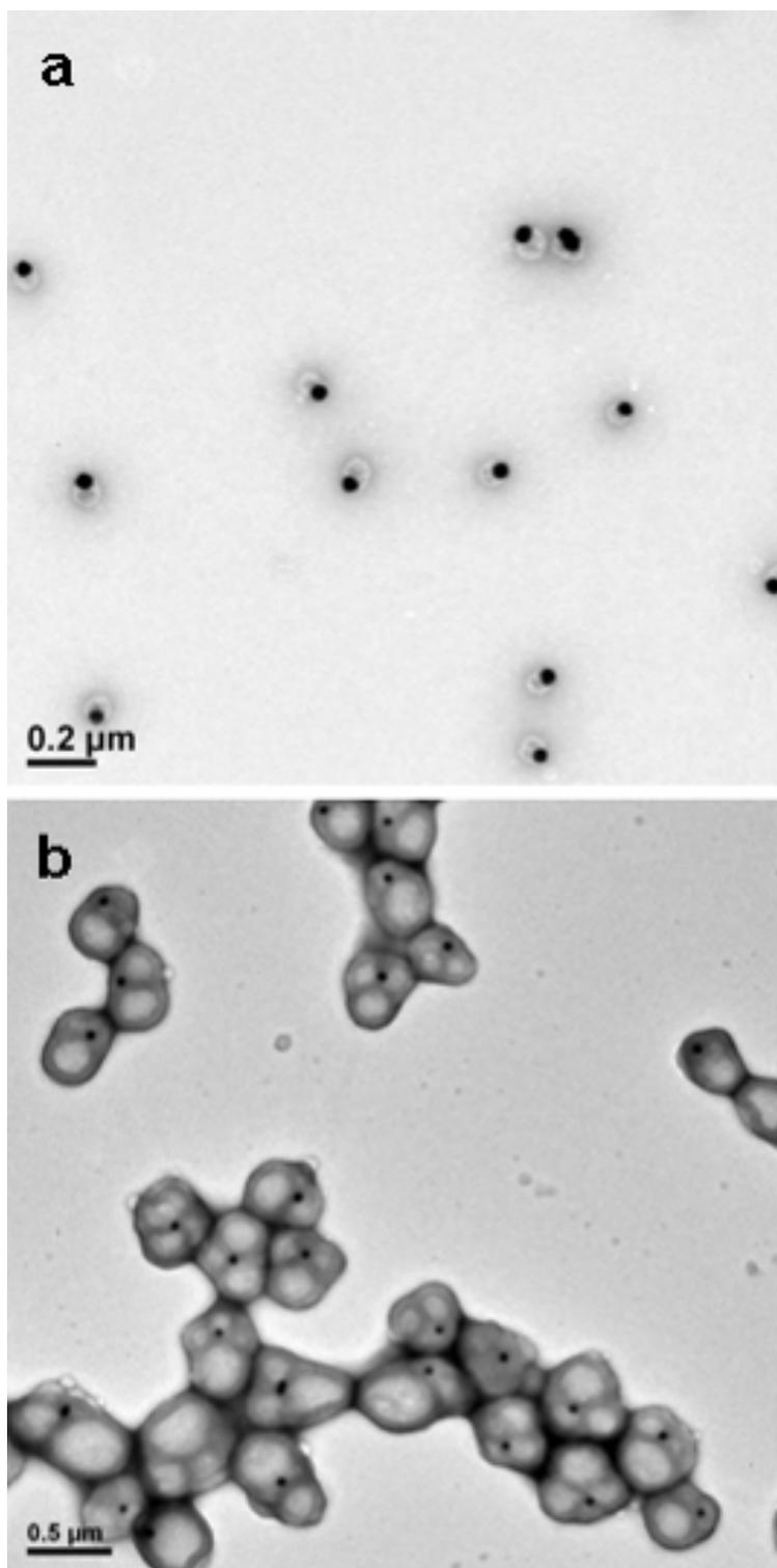
**Figure S15.** TEM images of (a) Au@vesicle NPs after oxidation by  $\text{H}_2\text{O}_2$ ,  $t = 2$  h; (b) sample a after purification and an additional growth cycle (large-area view of Figure 4b and 4c, respectively).
