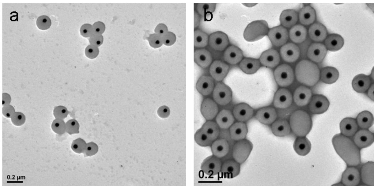
**Figure S16.** TEM images of (a) Au@polyaniline and (b) Au@polypyrrole core-shell NPs. The nanocomposites were prepared following the same method for the preparation of thiophene-based Au@vesicle NPs, but aniline or pyrrole was used instead of thiophene. The final reaction mixture contained aniline or pyrrole (50 mM), AuNPs (estimated 0.062 nM), SDS (2.5 mM), H<sub>2</sub>O<sub>2</sub> (60 mM), FeCl<sub>3</sub> (9 μM), and H<sub>2</sub>O (1.5 mL).
