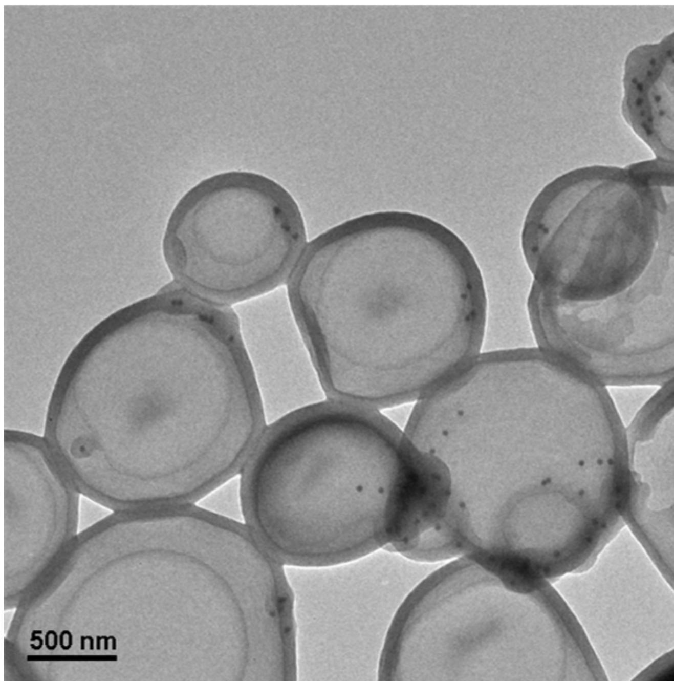
**Figure S10.** TEM image of the Au@vesicle NPs formed in the absence of SDS,  $d_{\text{Au}} = 40$  nm,  $t = 12$  h (large-area view of Figure 3g).
