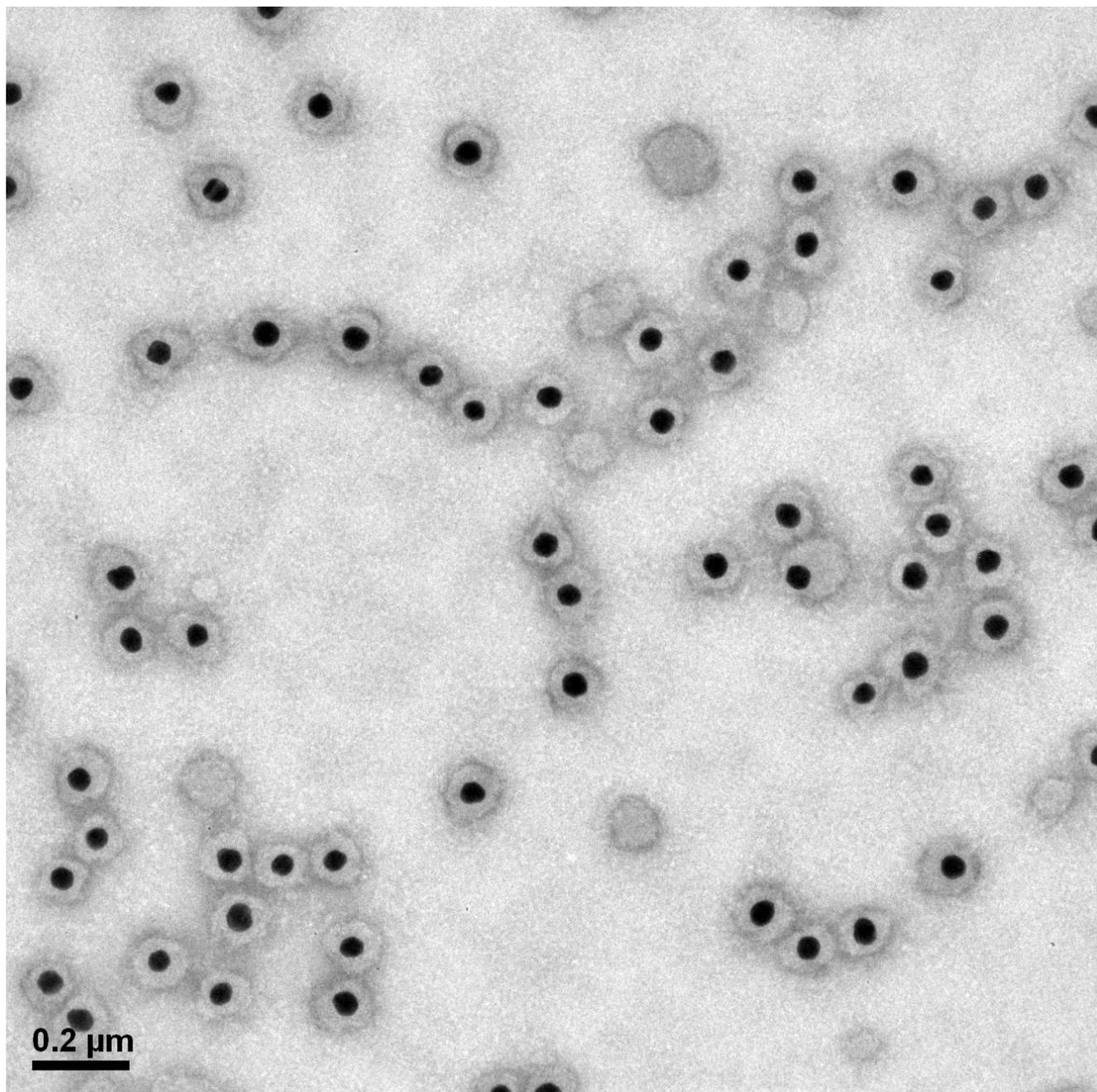
**Figure S1.** TEM image of the Au@PTh core-shell NPs,  $d_{\text{Au}} = 40$  nm, [SDS] = 5 mM,  $t = 12$  h (large-area view of Figure 1b).
