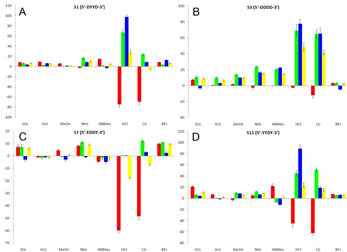
**Figure S8.** Quantitative color-change profiles of sensor sequences S1 (A), S3 (B), S7 (C) and S11 (D), showing spectral changes upon exposure to the eight selected toxic gases (1000 ppm). Error bars show variance in data averaged over 5 sensor beads.
