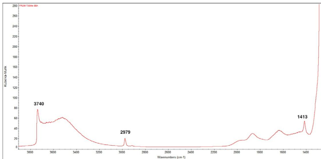
**Figure S4.** Diffuse reflectance infrared spectrum (DRIFT) of methyl-passivated silica (SBA-15).
