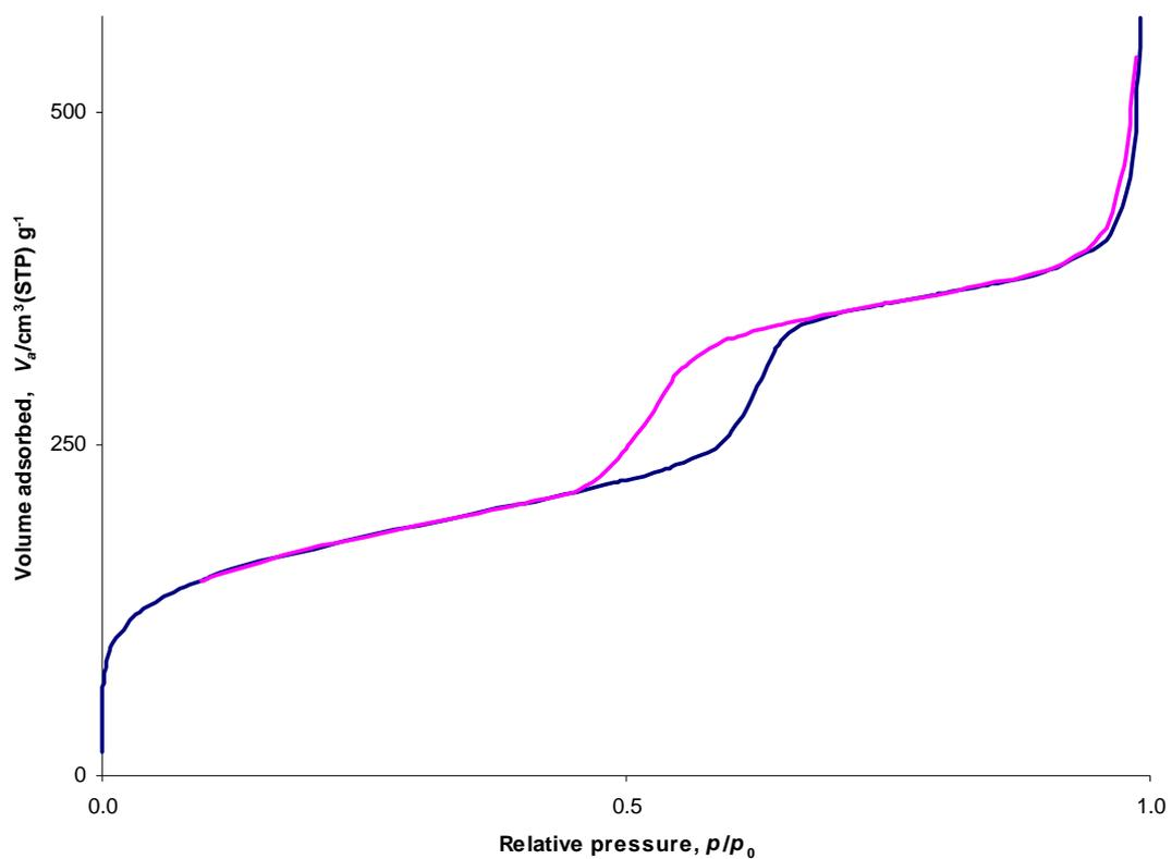
**Figure S3.** Nitrogen adsorption-desorption isotherm of methyl passivated silica (SBA-15). Isotherm type IV, characteristic of a mesoporous material. Surface (BET) Area =  $888 \pm 4 \text{ m}^2 \text{ g}^{-1}$ , Pore diameter (BJH) = 4.61 nm, Total pore volume (BET) =  $1.16 \text{ cm}^3 \text{ g}^{-1}$ .
