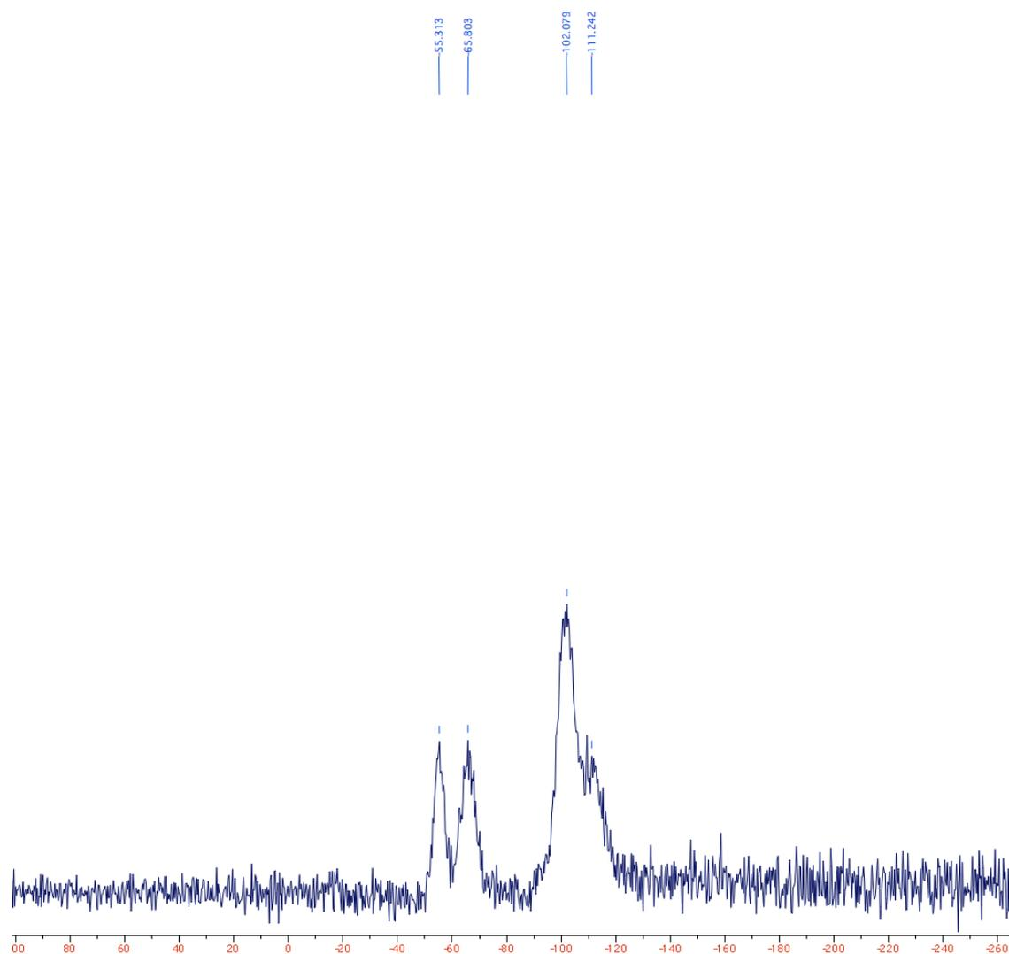
**Figure S7.**  $1\text{H}$ - $^{29}\text{Si}$  CP/MAS solid-state NMR spectrum of methyl-passivated silica (SBA-15) acquired with a sample spinning rate of 5 kHz with a total of 9060 scans, a contact time of 5 ms and a recycle delay of 16 s.
