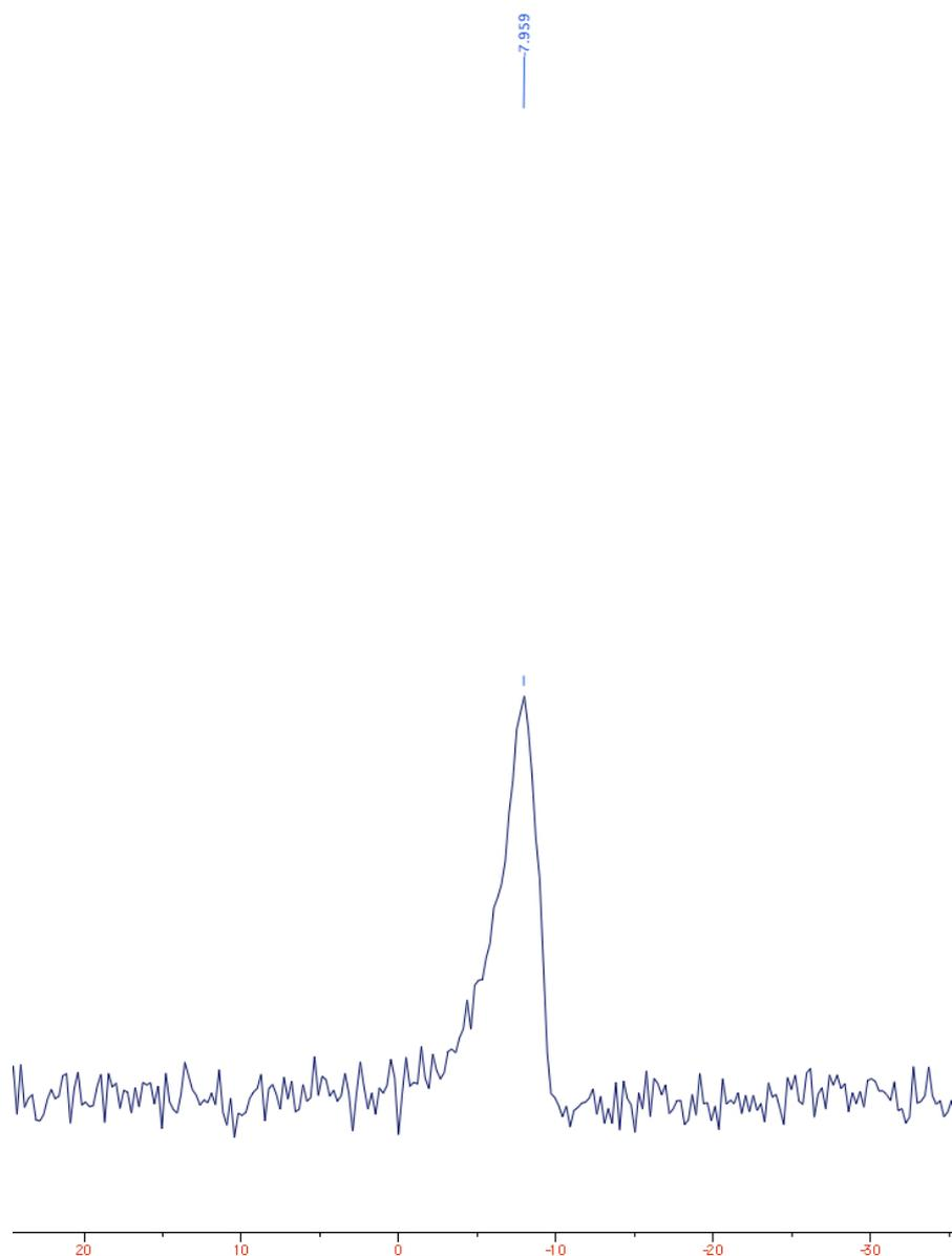
**Figure S6.**  $^1\text{H}$ - $^{13}\text{C}$  CP/MAS solid-state NMR spectrum of methyl-passivated silica (SBA-15), acquired with a sample spinning rate of 10 kHz.
