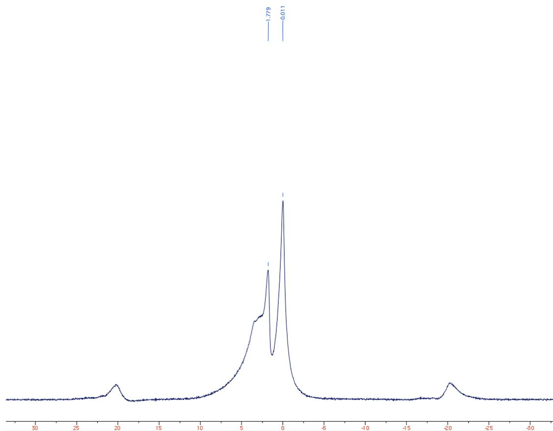
**Figure S5.**  $^1\text{H}$  Solid-state nuclear magnetic resonance spectrum of methyl-passivated silica (SBA-15) acquired with a sample spinning rate of 10 kHz with a total of 8 scans and a recycle delay of 256 s.
