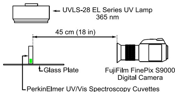
**Figure S2.** Darkroom setup for taking emission color photographs.
