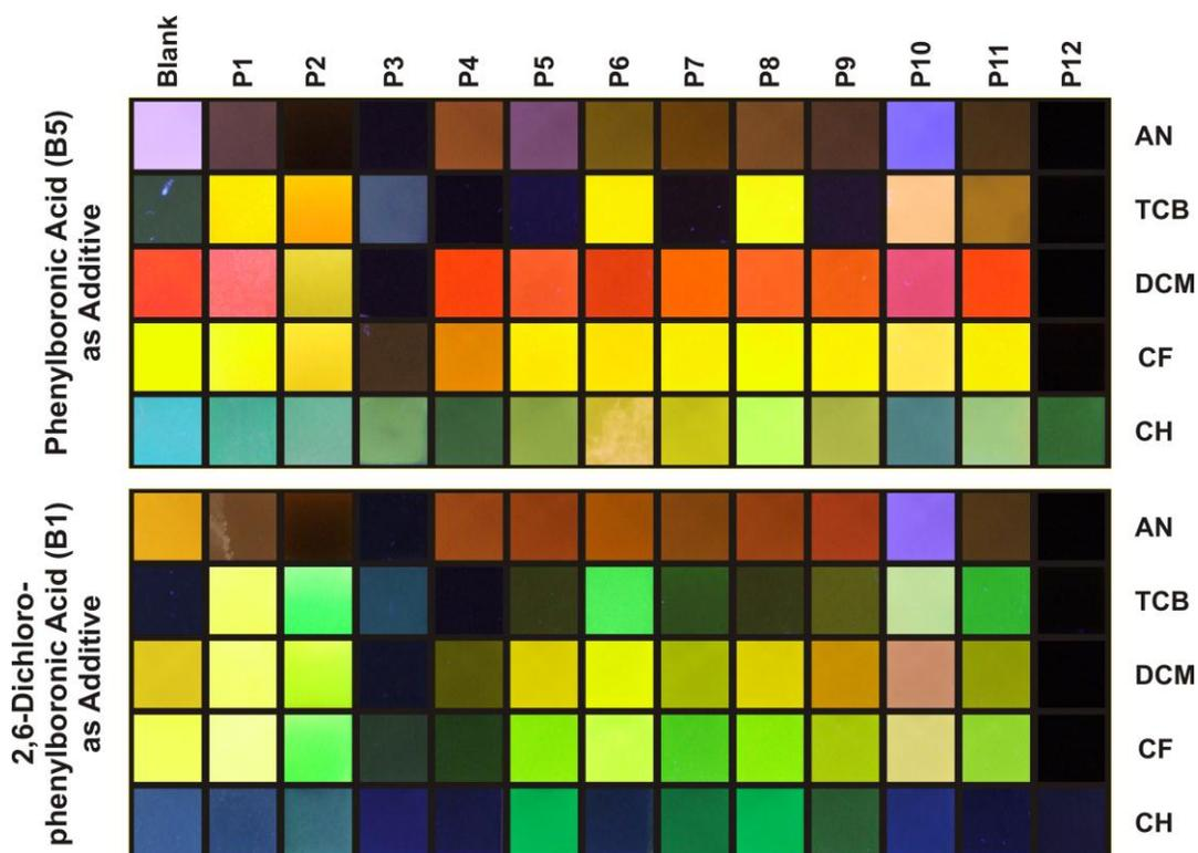
**Figure S6.** Panels with the photographs of the emission colors observed when the solutions of cruciform **1** and **B5** (top) and **B1** (bottom) were exposed to phenols **P1–P12**, and irradiated at 365 nm.
