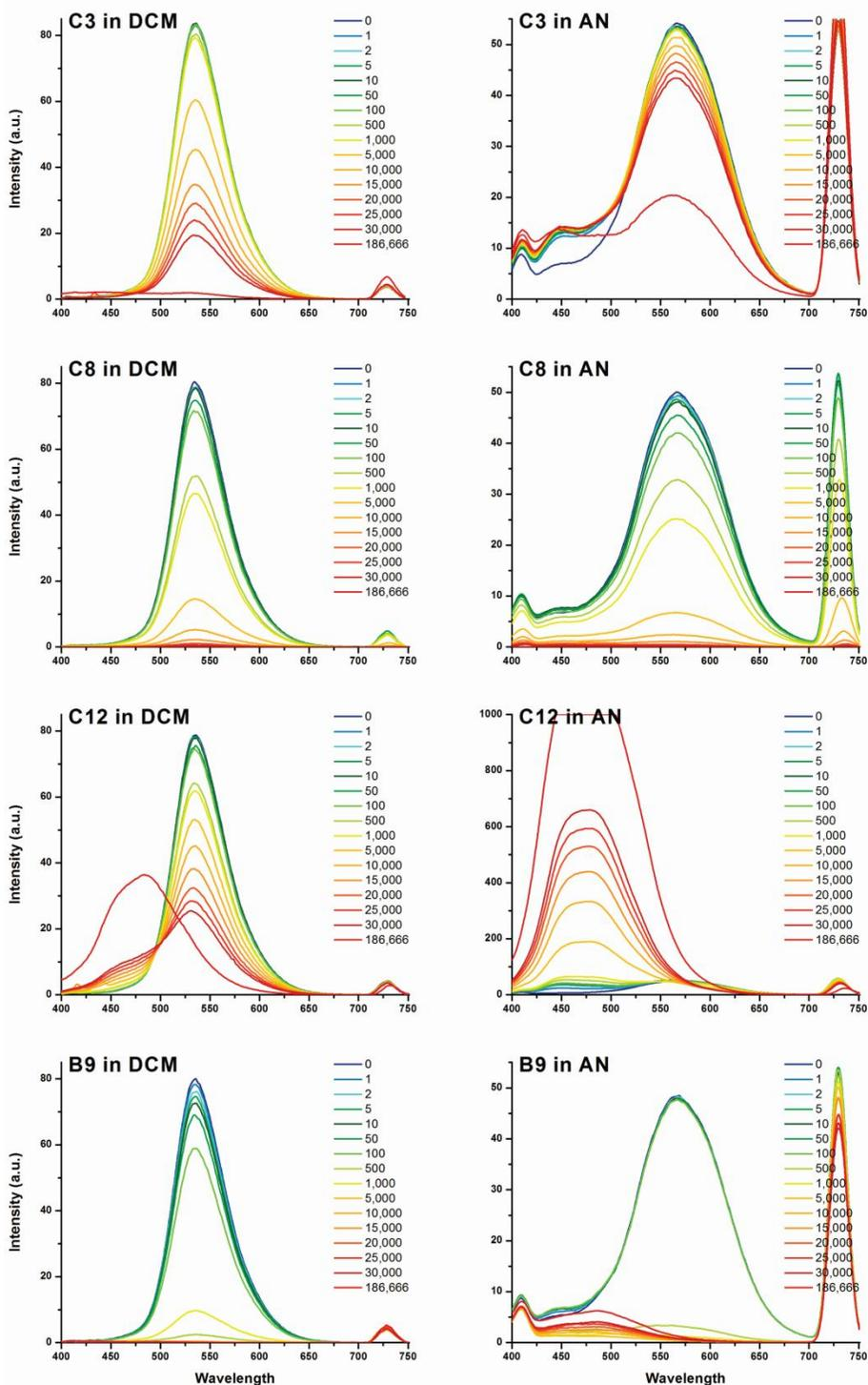
**Figure S10.** Fluorescence spectral titrations of cruciform **1** with analytes **C3**, **C8**, **C12**, and **B9** (from top to bottom), in DCM (left) and AN (right). Acids **C8** and **B9** quench **1**'s fluorescence quickly; compound **C3** partially quenches it, while **C12** causes a blue emission shift at high analyte concentrations. Numbers on the right-hand side of each graph indicate the number of equivalents of the analyte.
