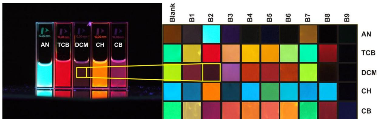
**Figure S4.** The original photo of emission colors of five **B2** solutions in UV/Vis spectroscopy cuvettes (left) and the panel of all boronic acids' emission colors in five solvents (right).
