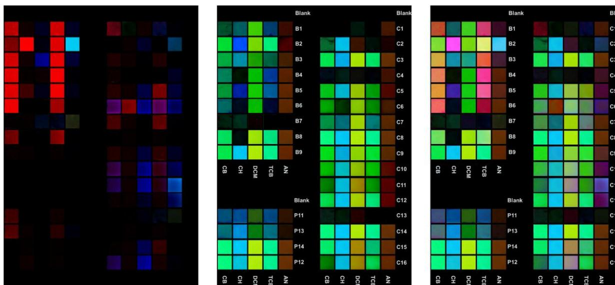
**Figure S9.** Three possible ways of subtracting the two images shown in Figure S6 from each other, using ImageJ image processing software. On the left, blank image is subtracted from the sample image (using ImageJ *Subtract* command). In the center, *Subtract* command was used to achieve the inverse—subtraction of the sample image from the blank image. Finally, image on the right shows the use of ImageJ's *Difference* command, the outcome of which is independent on the order of image input.
