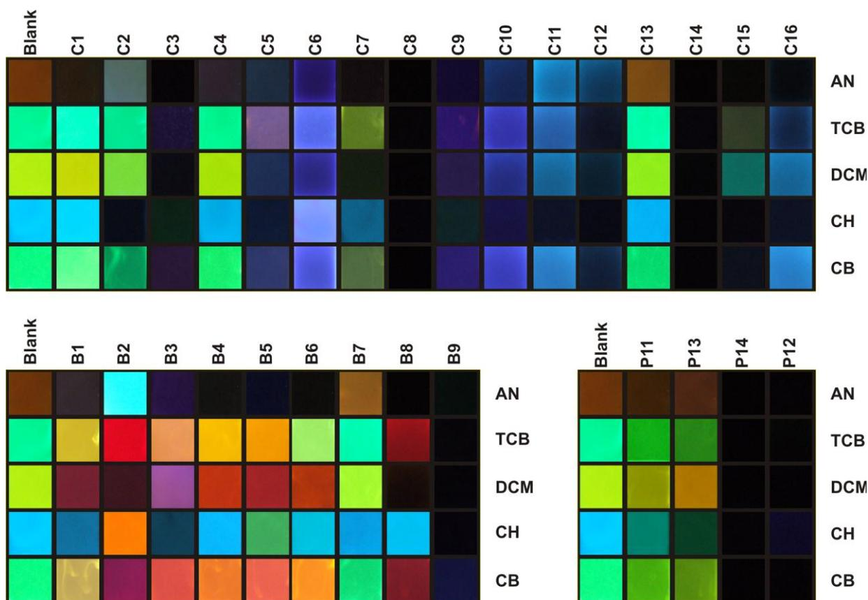
**Figure S5.** Panels with the photographs of the emission colors observed when the solutions of cruciform **1** were exposed to carboxylic acids **C1–C16** (top), boronic acids **B1–B9** (bottom left), and phenols **P11–P14** (bottom right), and irradiated at 365 nm.
