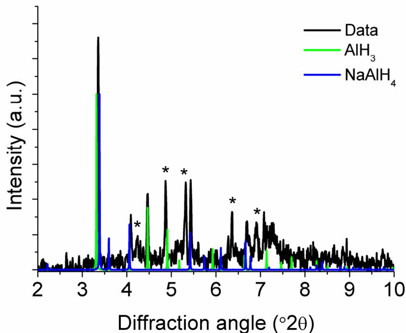
**Figure S3:** (a) Individual diffraction pattern of the series of phases located in the small portion of the catalyst body marked (●) in Figure 1 prior to oxidation along with simulated patterns of the phases which best fit the data. Unassigned peaks are marked \*.
