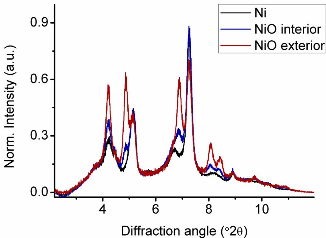
**Figure S5:** The summed XRD plot of the interior of the pellet clearly demonstrates the presence of NiO after oxidation. For comparison the summed plot from the exterior of the pellet and from a sample containing metallic Ni are also given.
