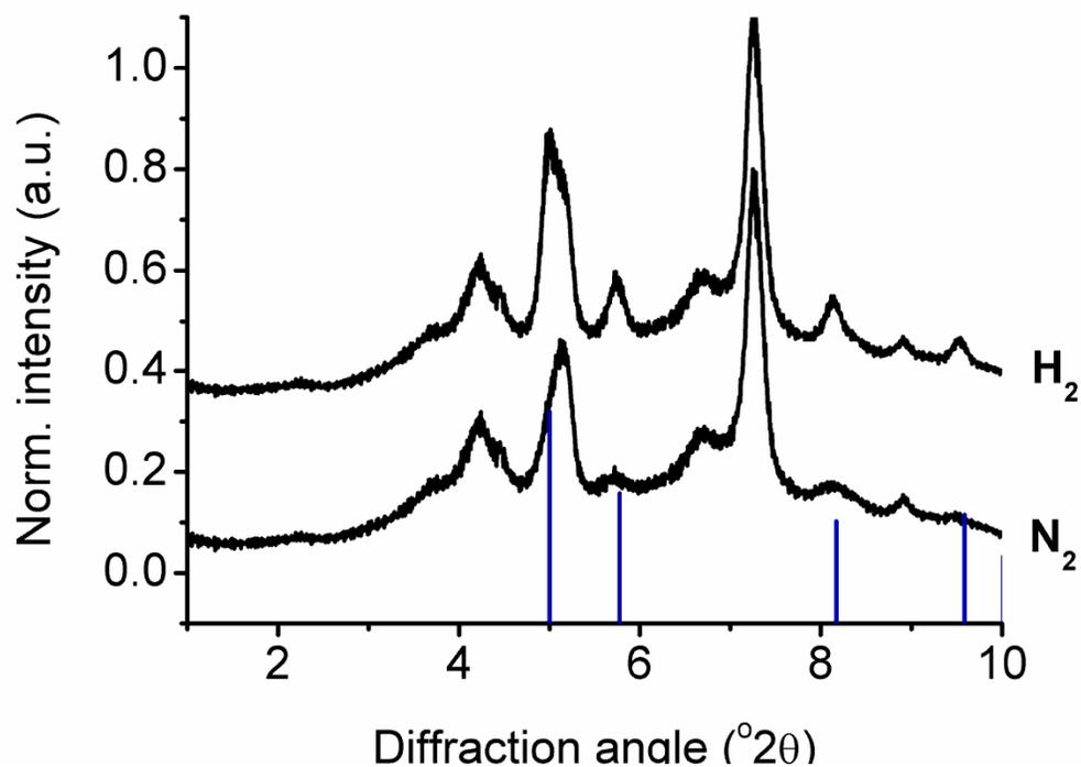
**Figure S7:** A comparison of the summed 1D XRD pattern for the entire catalyst slice after treatment in N<sub>2</sub> and H<sub>2</sub>. There is clearly far more scattering from metallic Ni after treatment in H<sub>2</sub> (the simulated pattern of cubic fcc Ni is given in blue).
