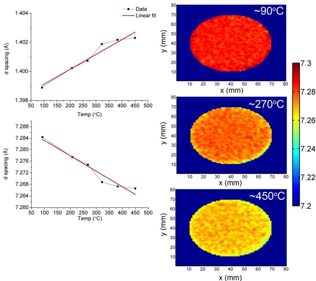
**Figure S1:** 1 dimensional plots of the variation in the d-spacing/ $2\theta$  position of the strong (2 0 0) reflection of  $\gamma$ - $\text{Al}_2\text{O}_3$  (left) and 2D plots of the variation in  $2\theta$  ° over the catalyst body at selected temperature in this range (right). Note that a common scale is used for comparison of the 2D plots.
