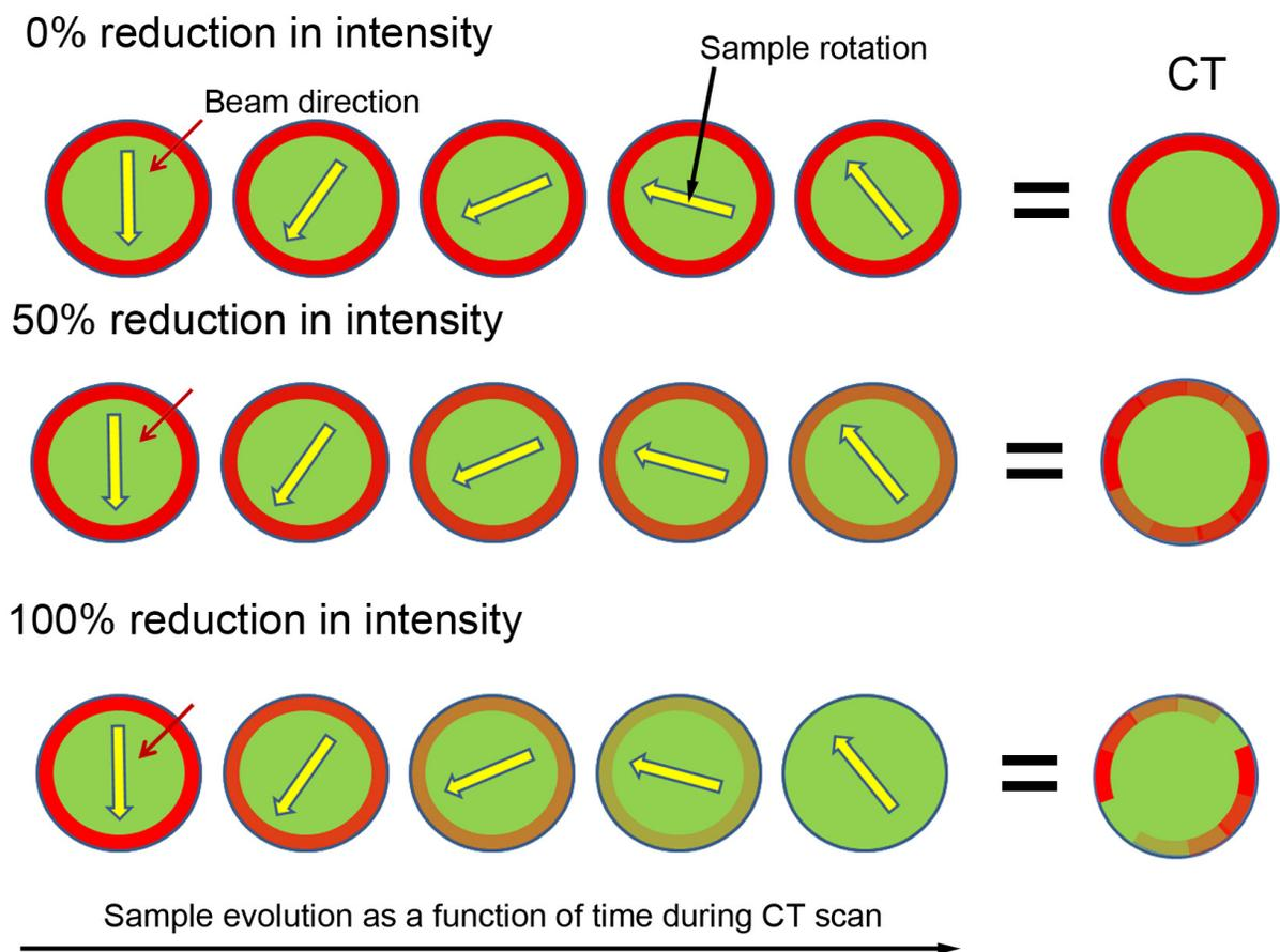
**Figure S5:** Demonstration of the effect of reduction in signal intensity due to phase consumption during a CT scan. In each case the time frame is the same but the reduction in intensity is different. The resulting CT image is also given.
