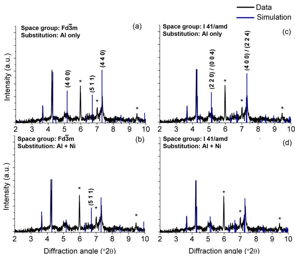
**Figure S6:** individual 1D XRD patterns for the region of the extrudate containing minority phases after treatment in O<sub>2</sub> along with several simulated patterns. The reflections with the most significant mismatch in intensity are labeled. The phase marked \* remains unidentified.
