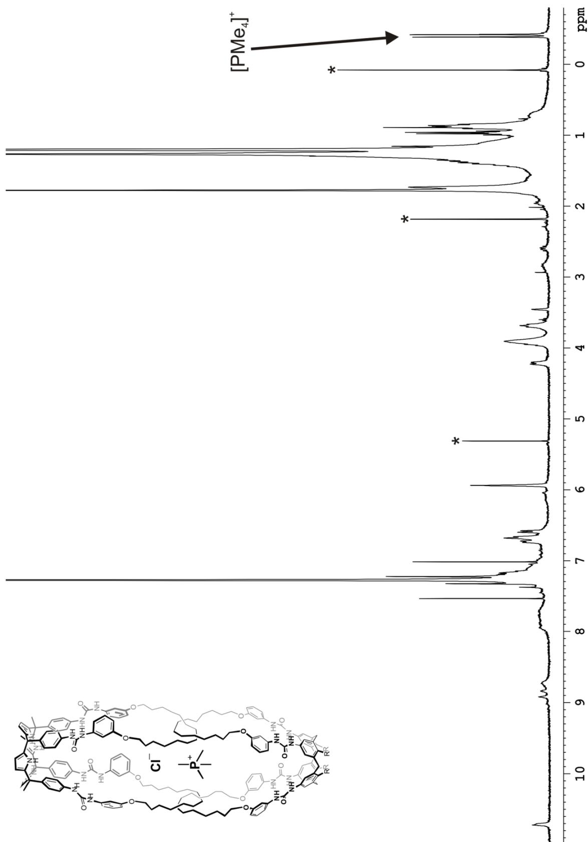
**Figure S16.**  $^1\text{H}$  NMR ( $\text{CDCl}_3$ ) of  $10\cdot\text{Cl}^- \cdot 3\cdot 5$ . The signal for the  $\text{TMP}^+$  cation at high field is indicated with an arrow. \* indicates solvent signals (DCM, acetone and silicone oil).
