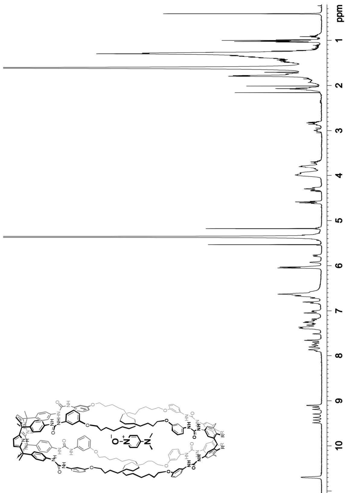
Figure S6.  $^1\text{H}$  NMR ( $\text{CDCl}_3$ ) of  $8\text{c} \cdot 3\cdot 5$ .
