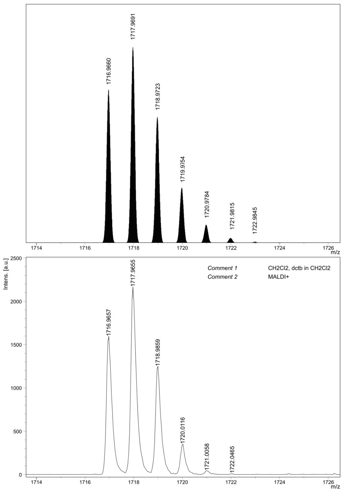
**Figure S1.** Exact MS (MALDI+) of calix[4]pyrrole **4b**; experimental (below) and theoretical calculated for  $C_{108}H_{124}N_{12}O_8^+$  (above).
