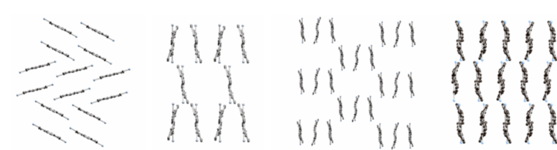
Figure S10. Packing structures of DPDC3 , DPDC7 , DPDC9 and DPDC11 (left to right). Solid-state packing changes from herringbone-type to aligned stacks of oligoenes as oligoene length is increased.
