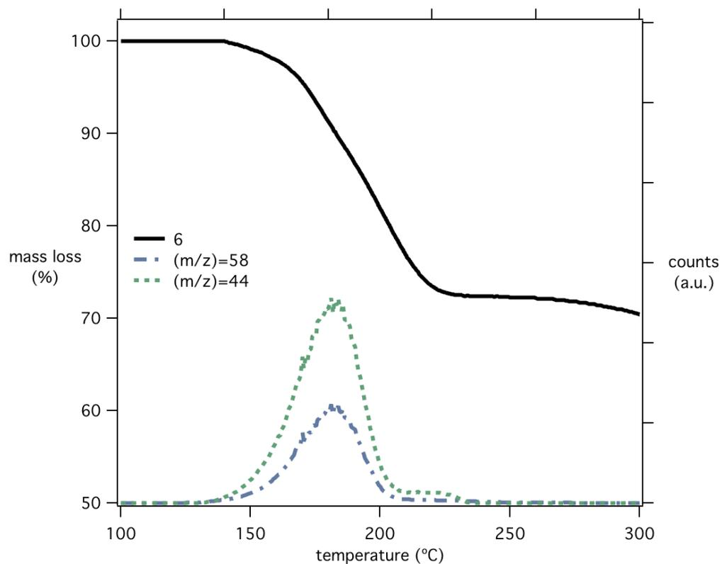
**Figure S1:** TGA coupled mass spectroscopy for polymer **6** showing the coincident loss of acetone and CO<sub>2</sub> upon thermolysis.
