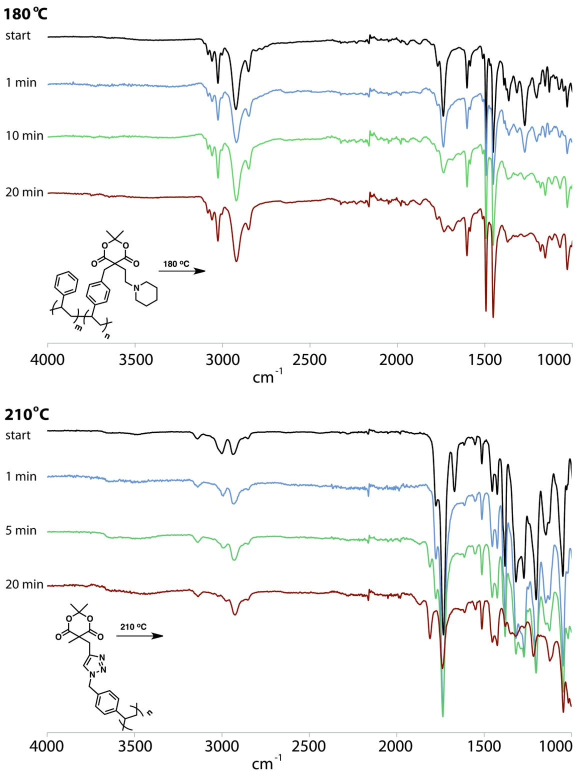
**Figure S2:** IR plots of polymers at various points during thermolysis. All materials were highly insoluble (crosslinked), but no stable ketene is observed at  $\sim 2100\text{ cm}^{-1}$ . The evolution of the carbonyl region is visible in both samples.
