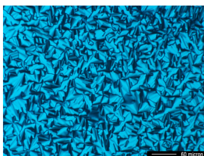
Figure S39. Polarising optical micrograph of mixture 3/4 in a 7:3 molar ratio in the Col H2 at 80 °C.
