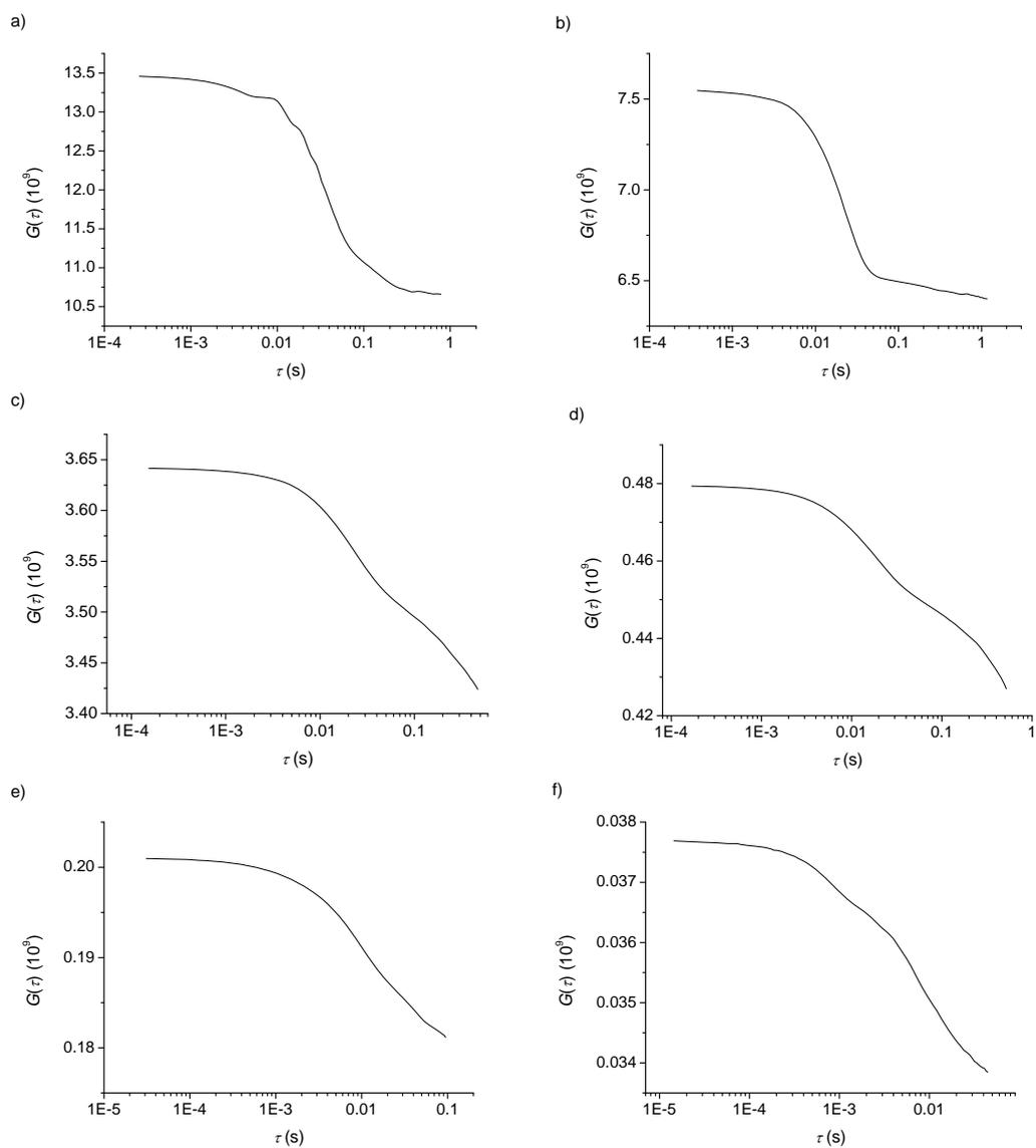
**Fig. S13** Autocorrelation functions  $G(\tau)$  of **4** in toluene solution (293 K) plotted against the delay time  $\tau$  for scattering angles a)  $10^\circ$ , b)  $14^\circ$ , c)  $20^\circ$ , d)  $26^\circ$ , e)  $66^\circ$ , and f)  $90^\circ$ .
