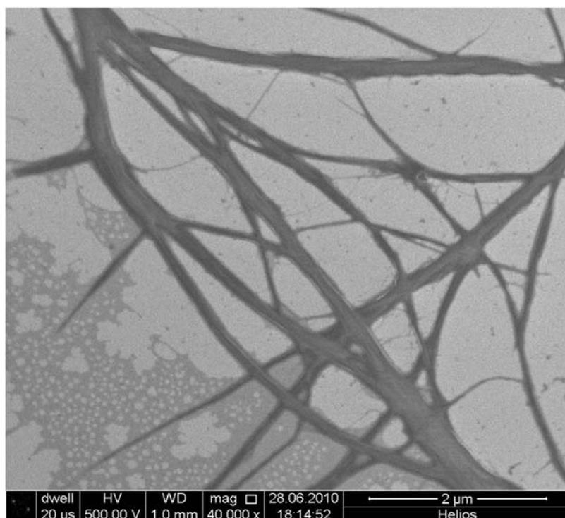
**Fig. S15** SEM image of a toluene solution of squaraine **4** ( $c = 1 \times 10^{-3}$  M).
