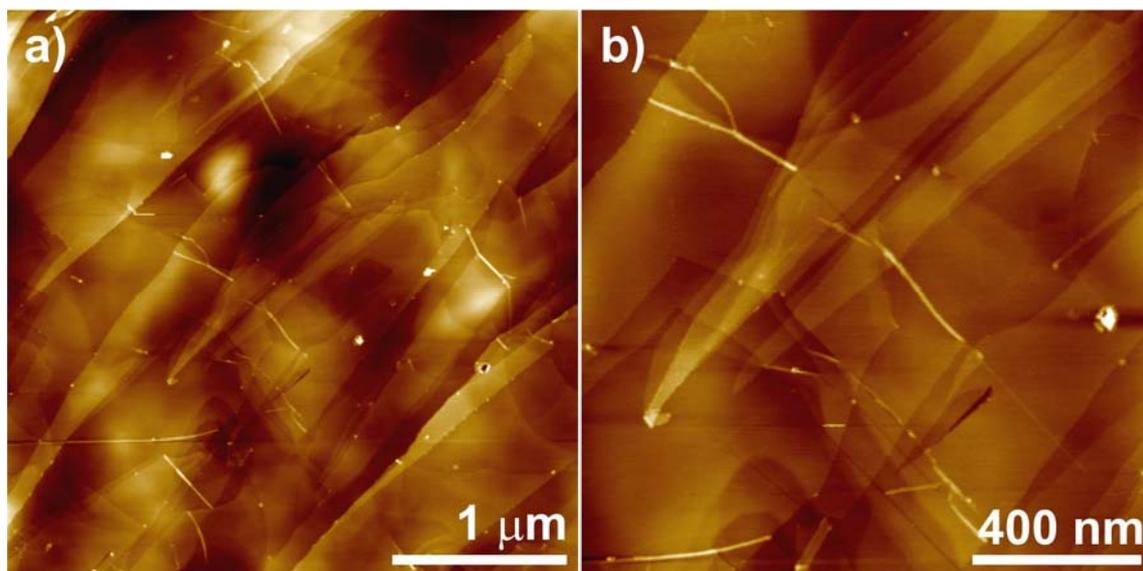
**Fig. S14** a), b) AFM images of samples spin-coated from a MCH solution of **4** ( $c = 5 \times 10^{-4}$  M, 5000 rpm) on HOPG.
