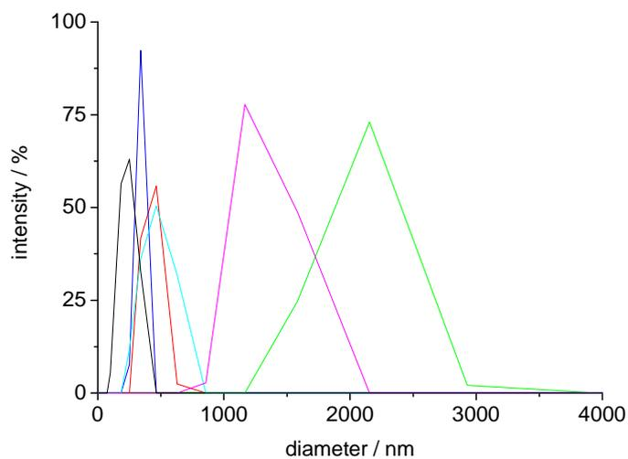
**Fig. S12** Angle-dependent intensity distribution obtained by dynamic light scattering experiments of **4** in toluene (black: 90°; blue: 14°; red: 10°; cyan: 26°; magenta: 66°; green: 20°) at 20 °C.
