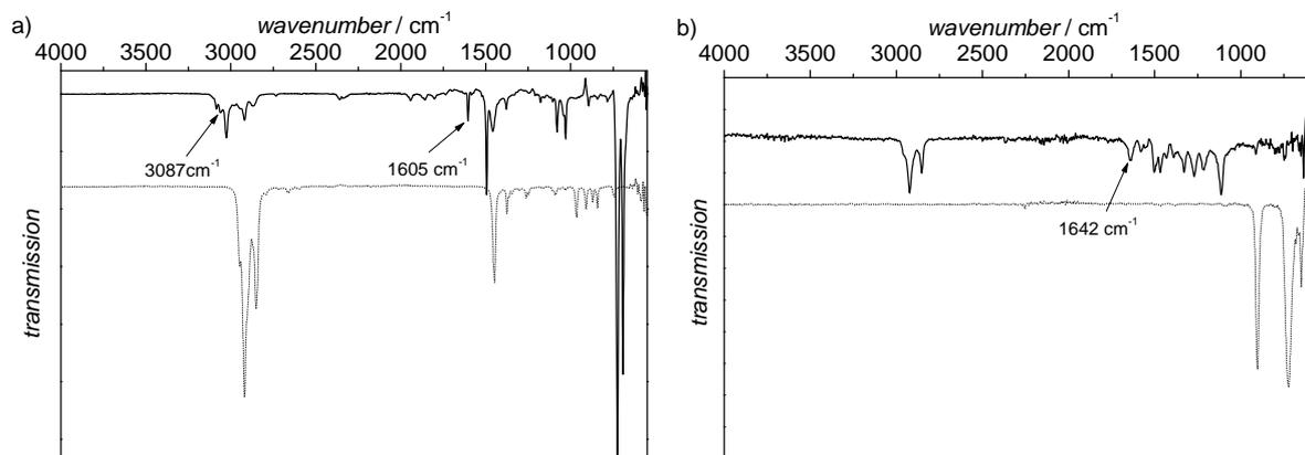
**Fig. S11** a) FTIR spectrum of MCH (dotted line) and a solution of squaraine **4** ( $10^{-3}$  M) in MCH (solid line) at 25 °C; b) FTIR spectrum of CDCl<sub>3</sub> (dotted line) and a solution of squaraine **4** ( $10^{-3}$  M) in CDCl<sub>3</sub> (solid line) at 25 °C.
