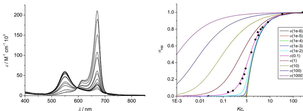
**Fig. S10** Left: Second set of concentration-dependent UV/vis/NIR absorption measurements of squaraine **4** in toluene. Right: Fraction of aggregated species  $\alpha_{\text{agg}}$  plotted as function of  $Kc_T$  with different  $\sigma$  values according to the cooperative growth model for the UV/vis concentration study (Fig. S6) at 670 nm (black points) for **4** in toluene at 20 °C.
