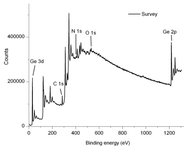
Fig. S8: XPS survey spectrum of a HCl-treated Ge surface functionalized with NMe<sub>2</sub>-BD
