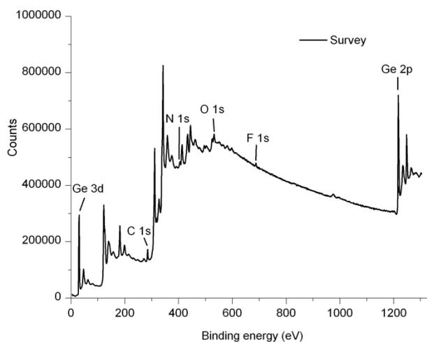
Fig. S9: XPS survey spectrum of a HCl-treated Ge surface functionalized with CF<sub>3</sub>-BD
