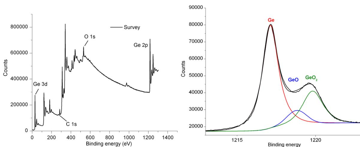
Fig. S1: XPS survey and Ge 2p core level spectra of a pristine Ge surface
