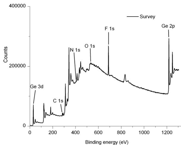
Fig. S10: XPS survey spectrum of a HCl-treated Ge surface functionalized with C<sub>8</sub>F<sub>17</sub>-BD
