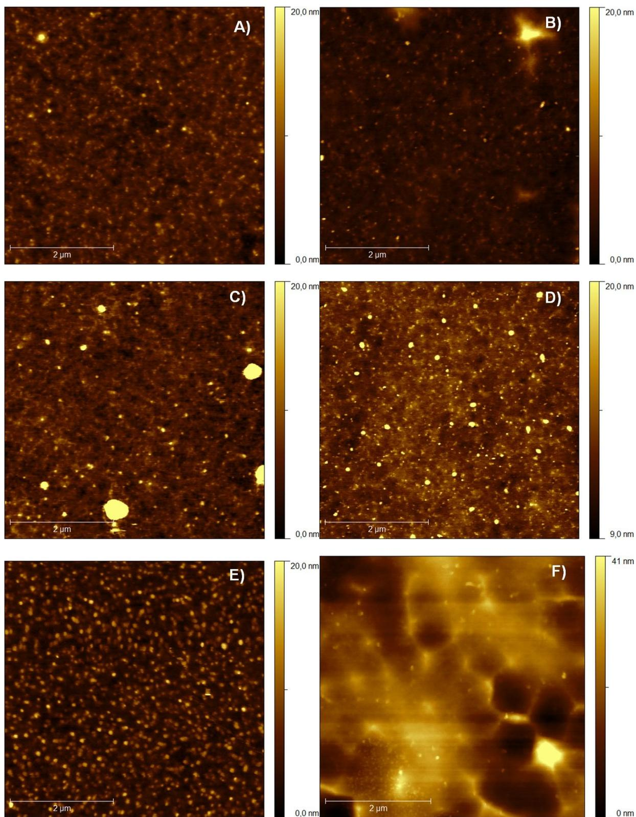
Fig. S14: AFM images of Ge surfaces grafted with CN-BD for 5 min (A) ( $R_q = 1.58$  nm), 10 min (B) ( $R_q = 1.75$  nm), 15 min (C) ( $R_q = 1.16$  nm), 30 min (D) ( $R_q = 1.64$  nm), 45 min (E) ( $R_q = 2.28$  nm) and 60 min (F) ( $R_q = 6.10$  nm).
