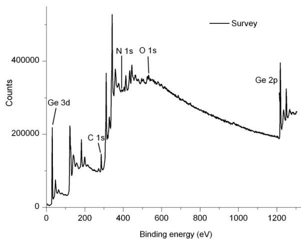
Fig. S4: XPS survey spectrum of a HCl-treated Ge surface functionalized with BD
