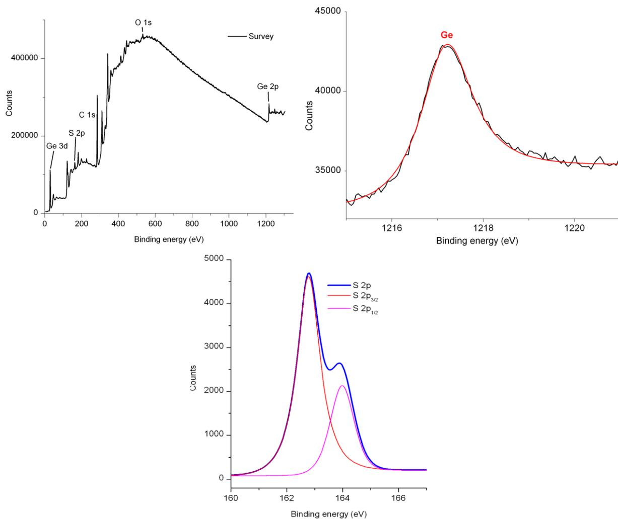
Fig. S3: XPS survey, Ge 2p and S 2p core level spectra of a HCl-treated Ge surface protected with a SAM of nonanethiol
