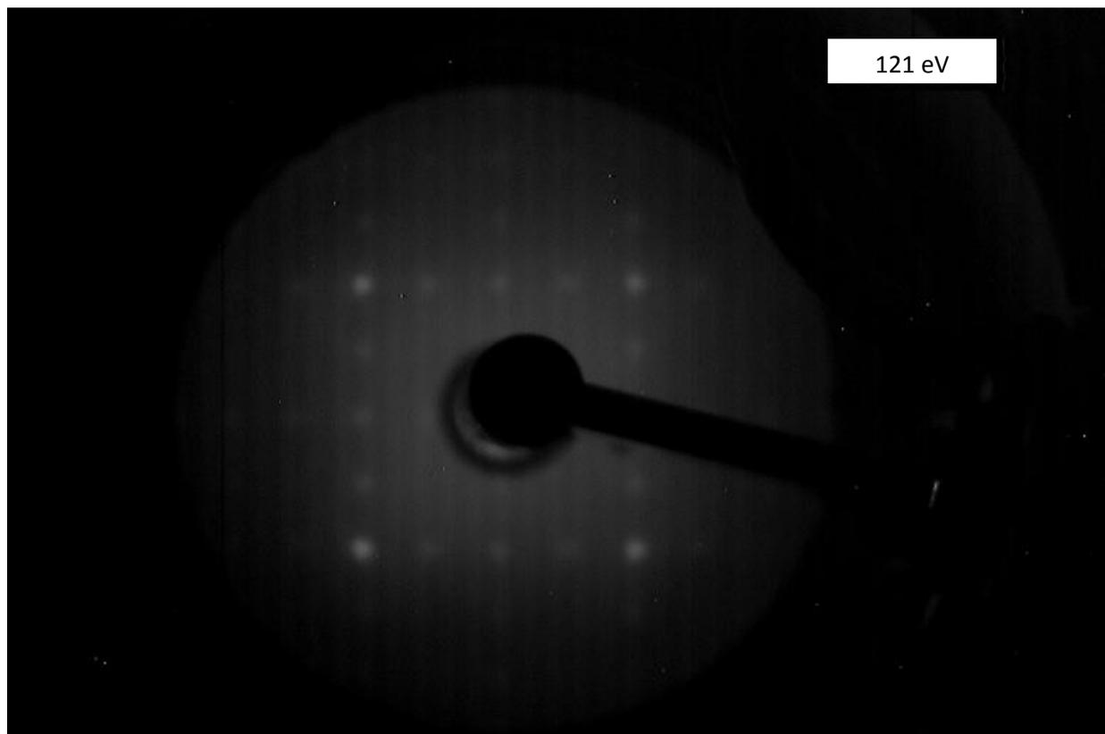
Fig. S15: LEED pattern of a HCl-treated Ge surface at 121 eV showing the (100) orientation and the 2x1 reconstruction.
