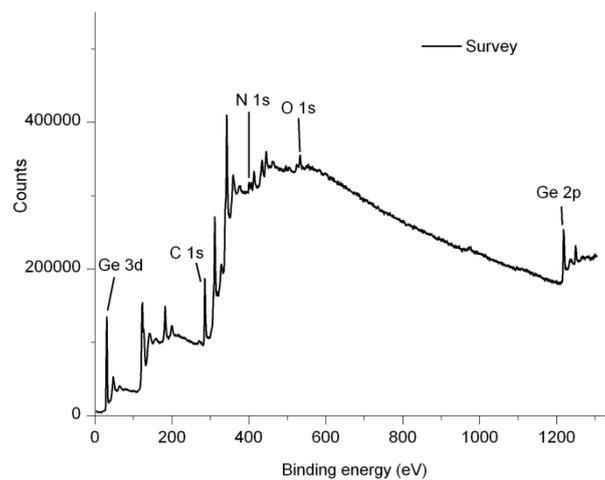
Fig. S11: XPS survey spectrum of a HCl-treated Ge surface functionalized with DO-BD
