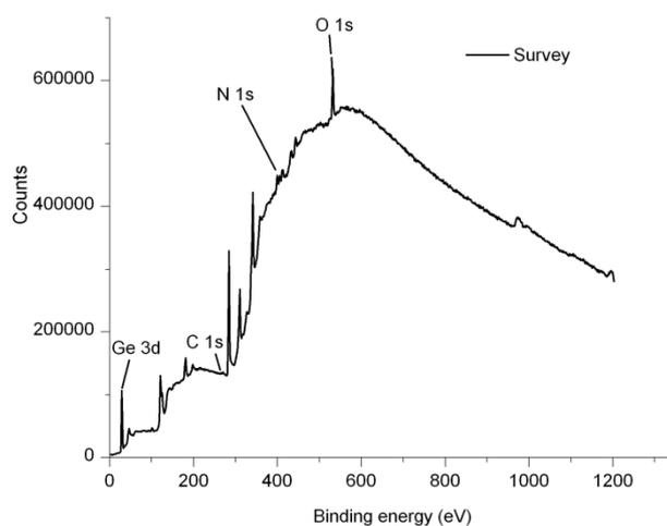
Fig. S6: XPS survey spectrum of a HCl-treated Ge surface functionalized with NBD
