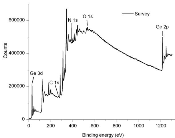
Fig. S5: XPS survey spectrum of a HCl-treated Ge surface functionalized with CN-BD
