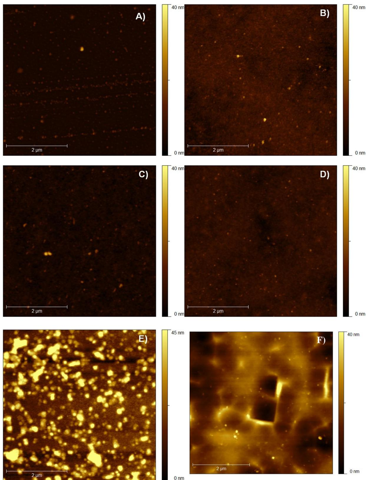
Fig. S13: AFM images of Ge surfaces grafted with CN-BD at -18°C (A) ( $R_q = 1.26$  nm), 0°C (B) ( $R_q = 2.05$  nm), 25°C (C) ( $R_q = 1.43$  nm), 40°C (D) ( $R_q = 1.47$  nm), 60°C (E) ( $R_q = 6.88$  nm) and 80°C (F) ( $R_q = 5.00$  nm).
