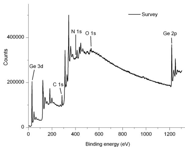
Fig. S7: XPS survey spectrum of a HCl-treated Ge surface functionalized with OMe-BD
