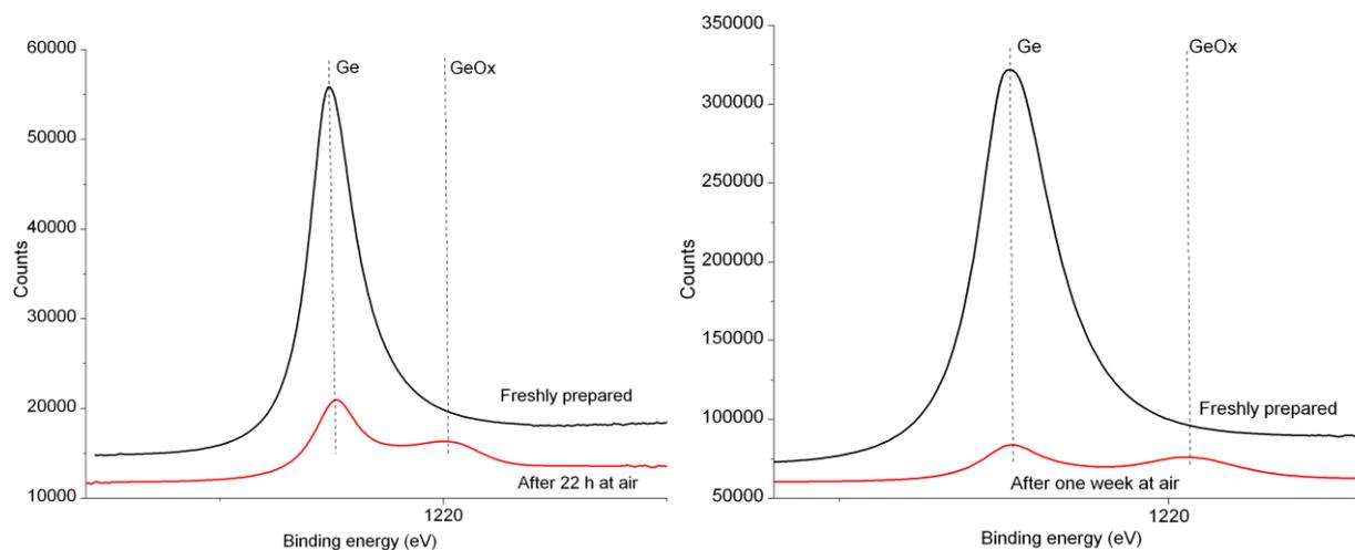
Fig. S12: XPS survey spectra of a nonathiolate SAM on a HCl-treated Ge surface freshly prepared (left, black line), after 22 hours at air exposure (30 % reoxidation, left, red line) and XPS survey spectra of a HCl-treated Ge surface functionalized with CF<sub>3</sub>-BD freshly prepared (right, black line), after one week at air exposure (54 % reoxidation, right, red line)
