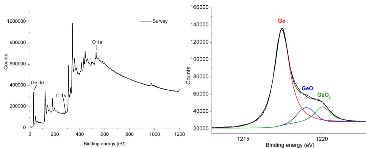
Fig. S2: XPS survey and Ge 2p core level spectra of a HCl-treated Ge surface
