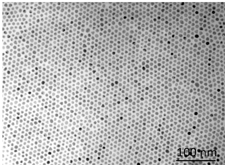
**Figure S6.** TEM image of Pt<sub>60</sub>Cu<sub>40</sub> nanocubes used for electrochemical study.
