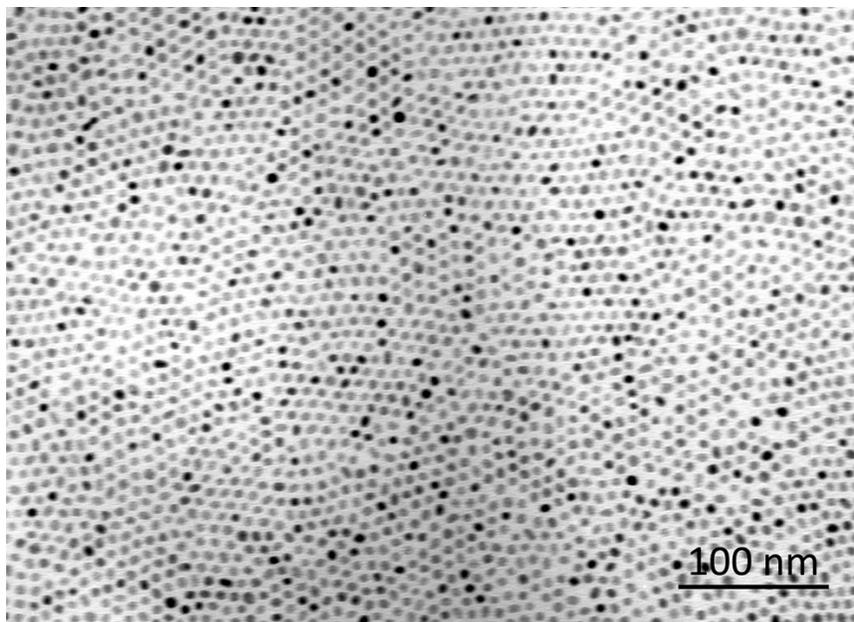
**Figure S4.** TEM images of Pt-Cu nanoparticles for tuning the particle morphology as a function of input  $\text{Cu}^{2+}/\text{Cu}^+$  molar ratio while other synthesis conditions were kept the same: (a), 8:1; (b), 6:1; (c), 5:1; (d), 4:1; (e), 1:1; (f), 1:6; (g), 1:10; (h), 0:1. Data bar: 100 nm.
