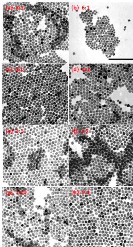
**Figure S5.** TEM image of Pt-Cu nanocrystals prepared using oleylamine as the reaction solvent without oleic acid, while the other conditions were same as those of typical Pt-Cu nanooctahedron synthesis.
