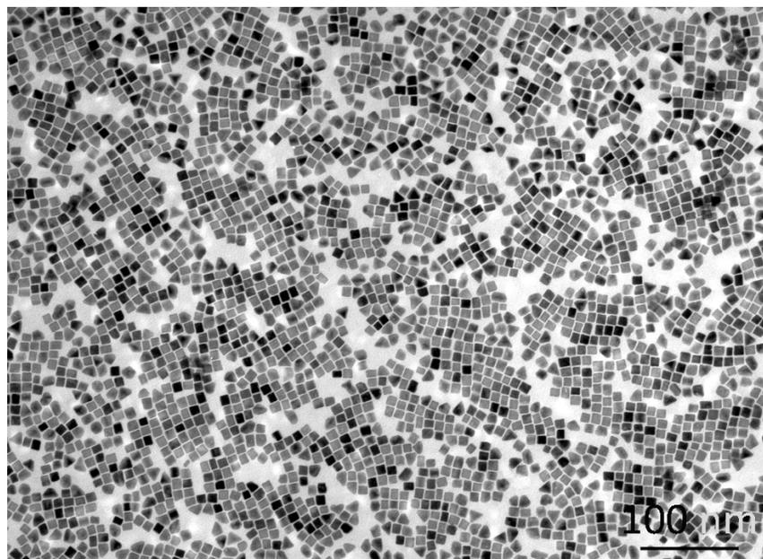
**Figure S7.** TEM image of the Pt-Cu nanooctahedra after an electrochemical measurement.
