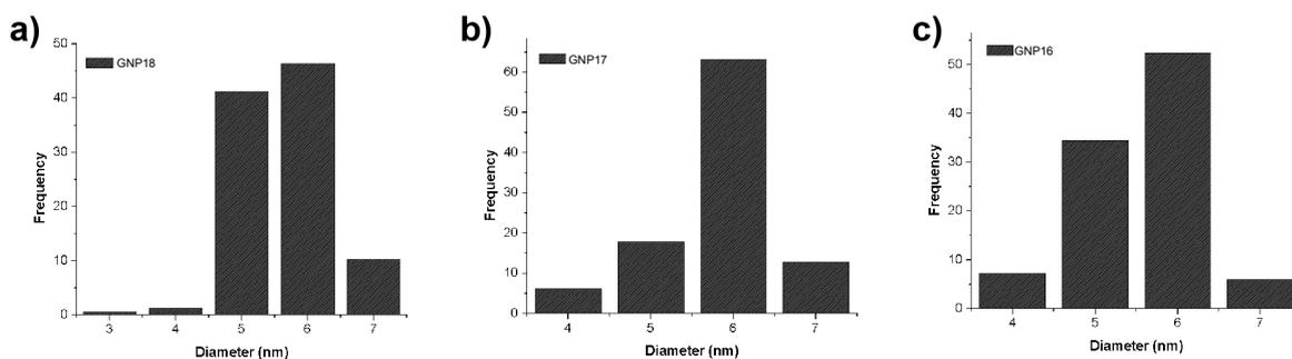
**Figure S17.** Particle size distribution (PSD) charts obtained counting a population of 150 nanoparticles from TEM micrographs of samples (a) GNP18, (b) GNP17 and (c) GNP16.
