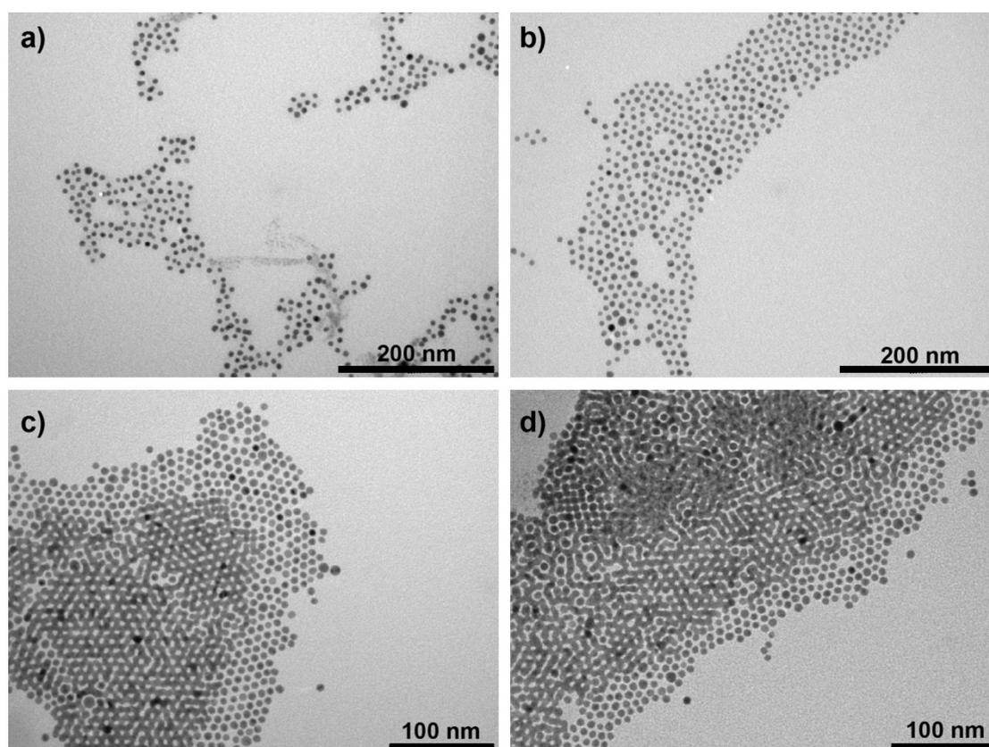
**Figure S16.** Transmission electron micrographs of (a) PEGylated GNPs (GNP18) and RNA-functionalized GNPs (b) GNP17; (c, d) GNP16.
