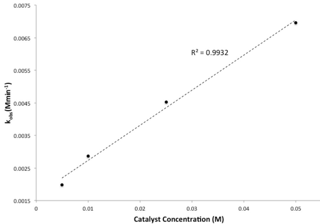
**Scheme 7:** Plot of  $k_{\text{obs}}$  vs. catalyst concentration, using method of initial rates.
