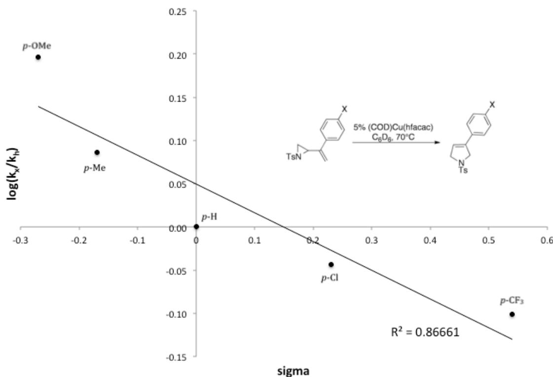
Scheme 4: Hammett plot of *para*-substituted aryl olefin substrates with (COD)Cu(hfacac).
