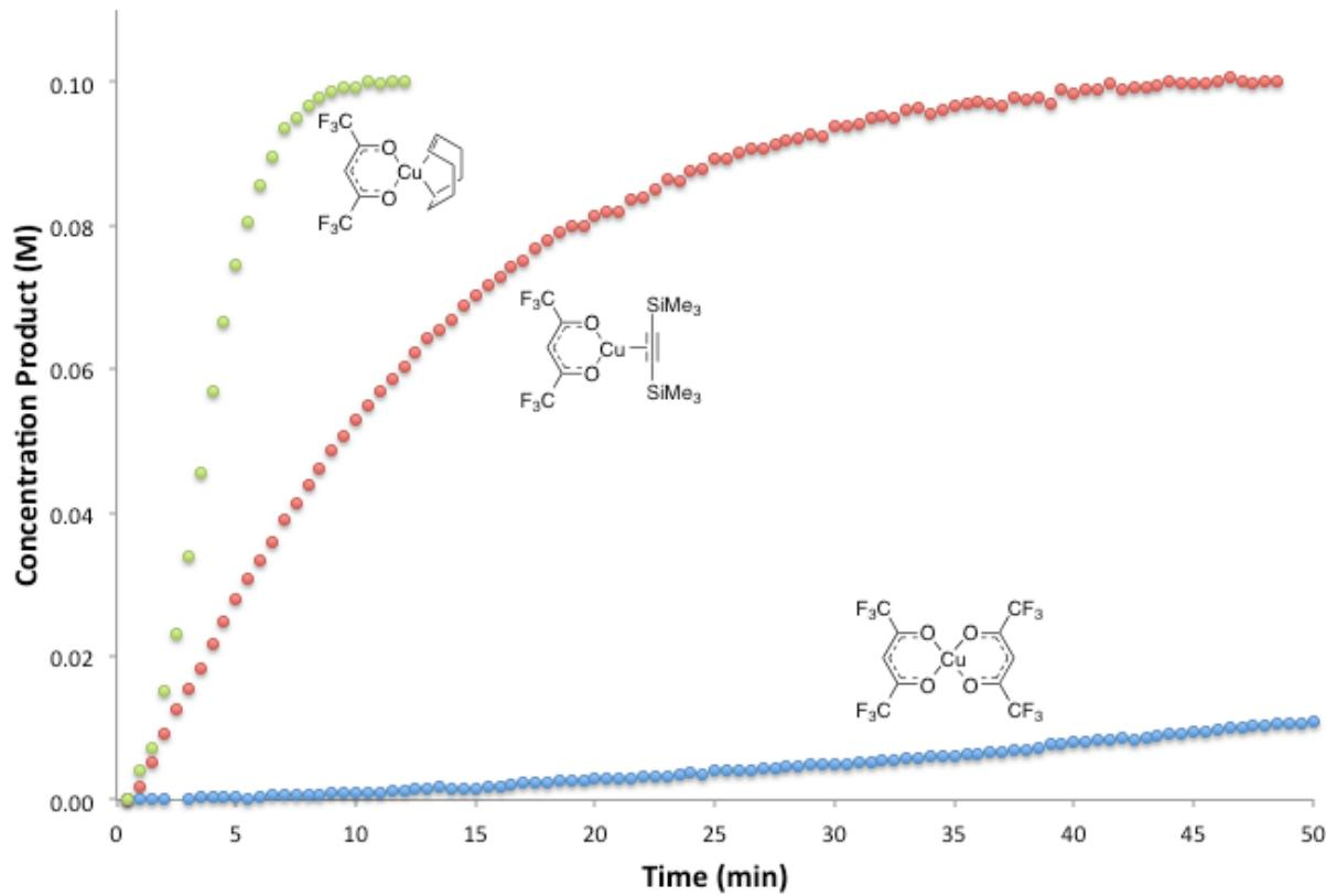
**Scheme 2:** Kinetic traces of rearrangement of 1 with different catalysts.
