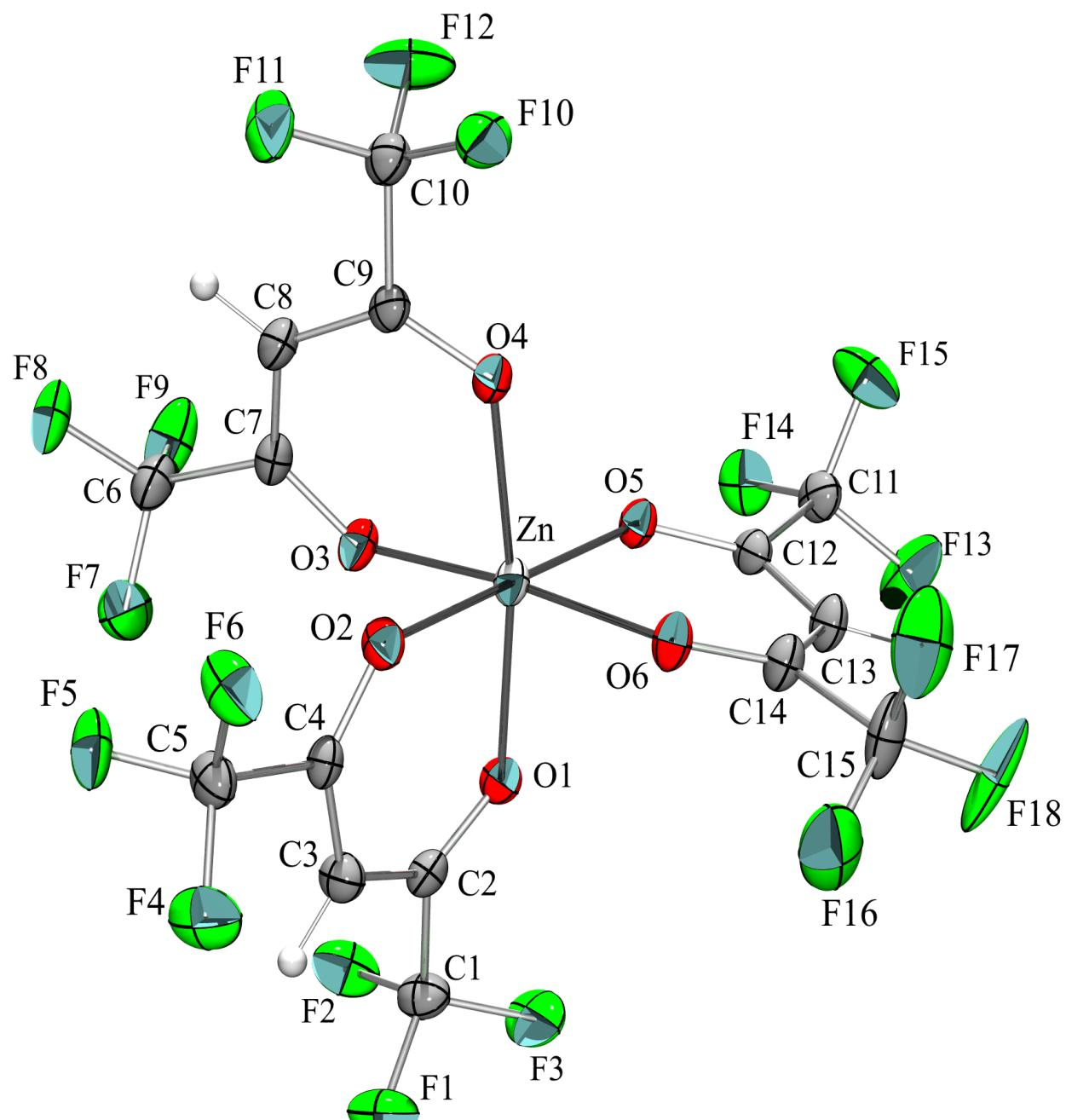
**Zn(hfacac)<sub>3</sub>NEt<sub>4</sub> (tetraethylammonium salt and hydrogens omitted for clarity)**
