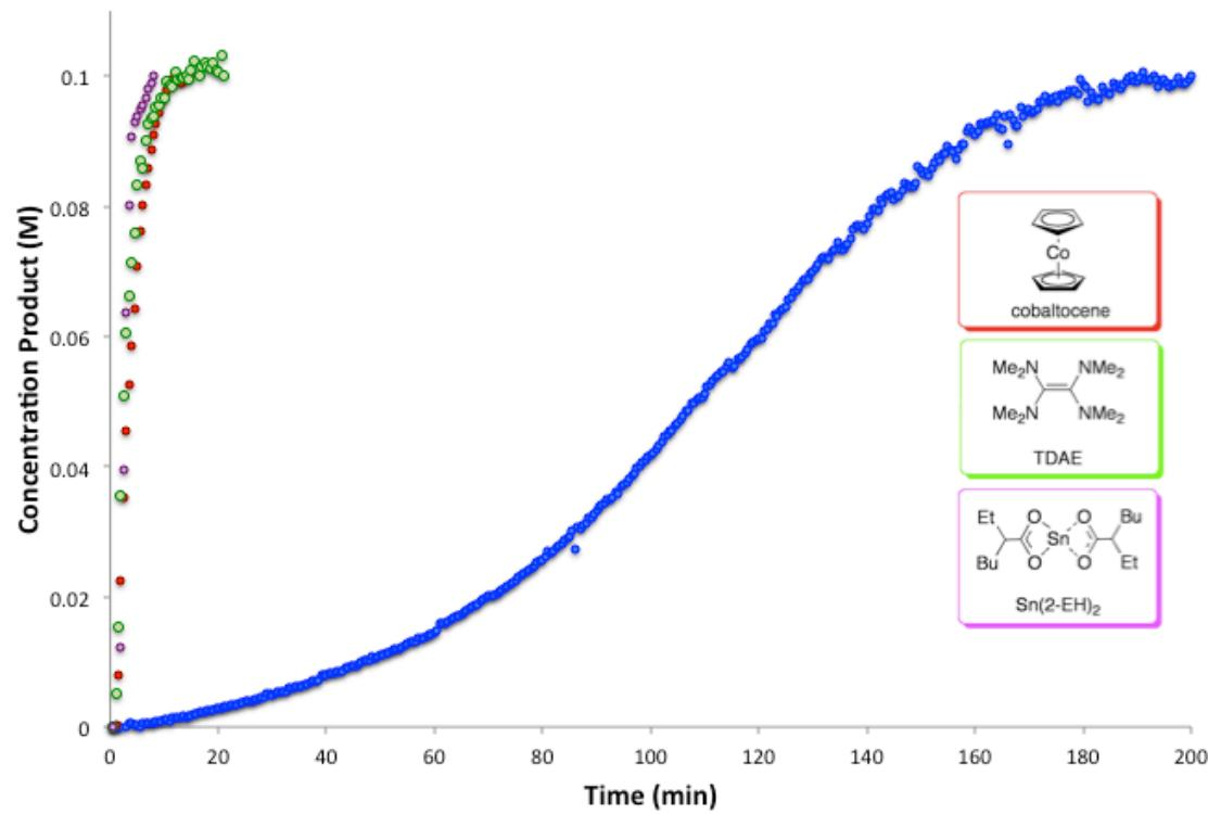
**Scheme 1:** Kinetic traces of rearrangement of 1 with and without added reductants.
