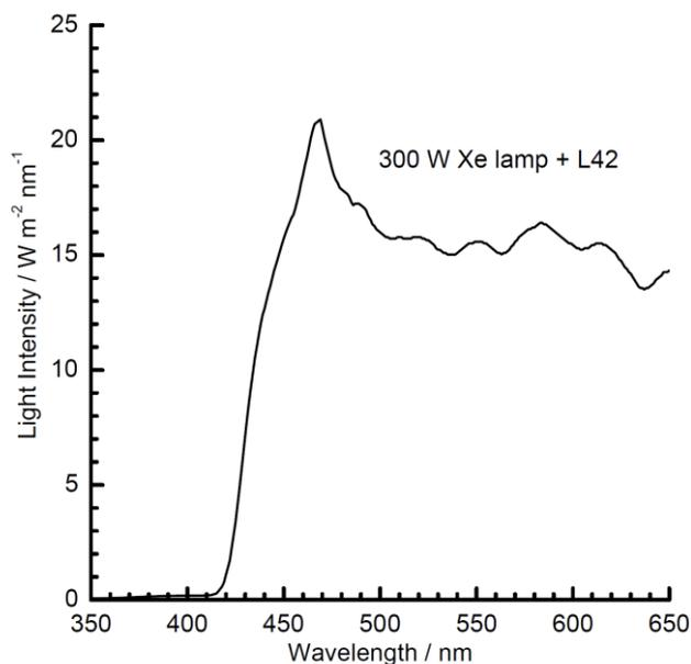
**10 Fig. S2** The spectrum of 300 W Xe lamp equipped with cut-off filter (HOYA, L42).
