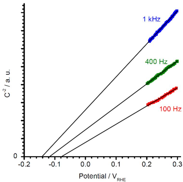
**Fig. S5** Mott-Schottky plot of the LaTiO<sub>2</sub>N/Ta electrode in 1 M aqueous Na<sub>2</sub>SO<sub>4</sub> solution (pH = 6). The flat band potential was estimated to be -0.08 to -0.14 V<sub>RHE</sub> by extrapolating C<sup>-2</sup> to 0.
