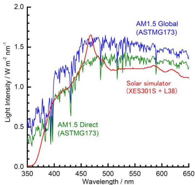
**Fig. S1** The spectrum of used solar simulator. As a solar simulator, the commercially-supplied solar simulator (SAN-EI ELECTRIC, XES301S) equipped with cut-off filter (HOYA, L38) was employed. The spectrum of the solar simulator shown in FigS1 is calibrated to AM1.5 Direct (AM1.5D).
