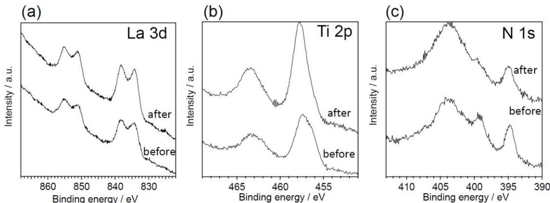
**Fig. S3** XPS results for La3d, Ti2p and, N1s of electrodes with modifying IrO<sub>2</sub> colloids. The binding energies determined by XPS were corrected in reference to the C 1s peak (284.6 eV).
