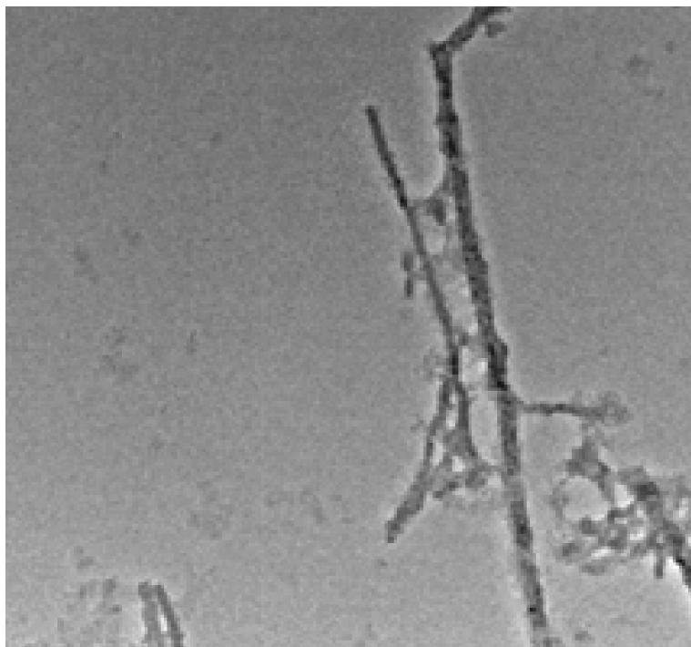
Figure S10. Additional TEM image of the 1D-0D ZnTe/ZnS-CdTe/CdS NW-QD NHSs.
