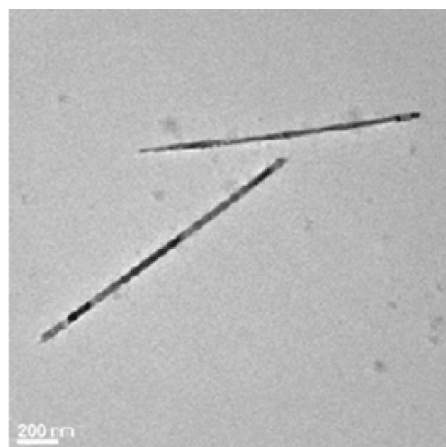
Figure S3. Additional TEM images of the ZnTe/ZnS core/shell nanowires functionalized with DNA.
