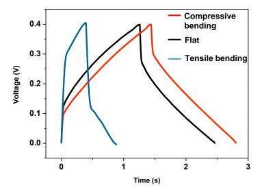
**Fig. S2.** Typical shapes of charge/discharge curve were observed for the different bending states of transparent and ultra-bendable supercapacitor with interdigitated patterned electrode system; flat, compressive and tensile bending state. Current density is  $150\mu A$  cm<sup>-2</sup> and bending radius is 1.5 mm (curvature is 6.7 cm<sup>-1</sup>).
