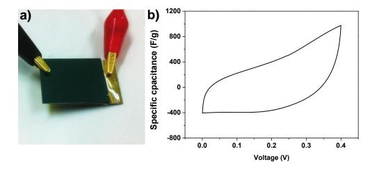
**Fig. S3.** a) Photograph and b) Cyclic voltammogram for a conventional sandwich type supercapacitor based on the same hierarchical MnO<sub>2</sub> structure.
