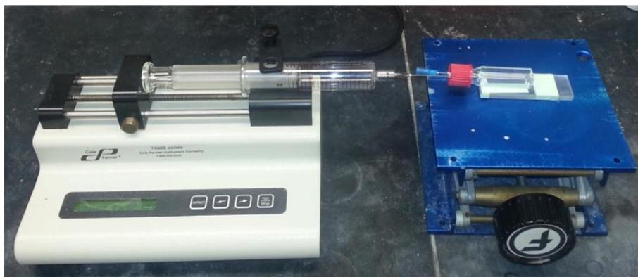
**Figure S6.** Syringe pump and optical cell used for analyzing headgas from contaminated soils.
