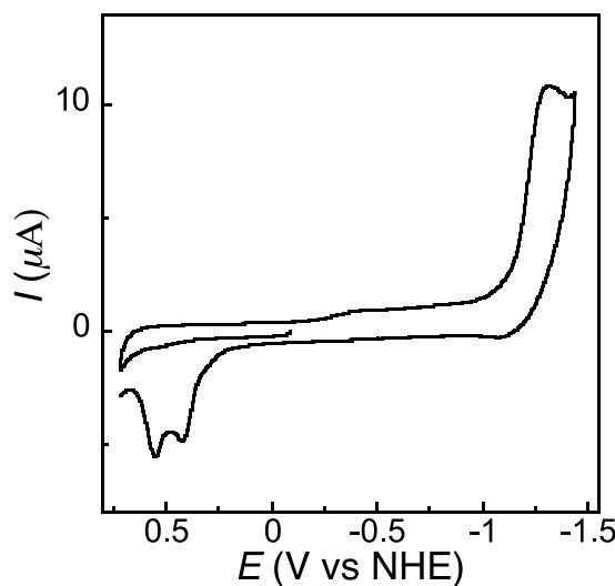
**Figure S2.** Cyclic voltammograms of  $\mathbf{2}^{\text{MeCN}}$  in water under Ar. (glassy carbon working electrode,  $7.1 \text{ mm}^2$ ,  $0.1 \text{ M NaHCO}_3$ ,  $200 \text{ mV/s}$ ,  $1\% \text{ v/v MeCN}$ , room temperature)
