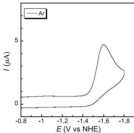
**Figure S6.** Cyclic voltammograms of  $2^{\text{OTf}}$  in THF under 1 atm Ar. (glassy carbon working electrode,  $7.1 \text{ mm}^2$ , 0.1 M  ${}^n\text{Bu}_4\text{NPF}_6$ , scan rate 100 mV/s, room temperature)
