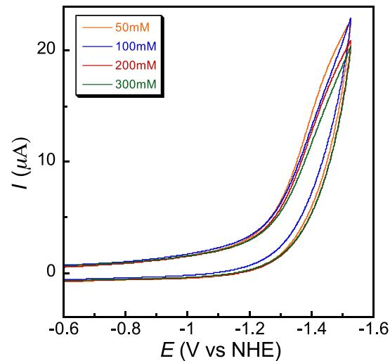
**Figure S5.** Cyclic voltammograms of  $\mathbf{2}^{\text{MeCN}}$  in water with 50–300 mM  $\text{NaHCO}_3$  under 1 atm  $\text{CO}_2$ . (glassy carbon working electrode,  $7.1 \text{ mm}^2$ , 0.3 M ionic strength balanced with  $\text{NaNO}_3$ , scan rate 100 mV/s, 1% v/v MeCN, room temperature)
