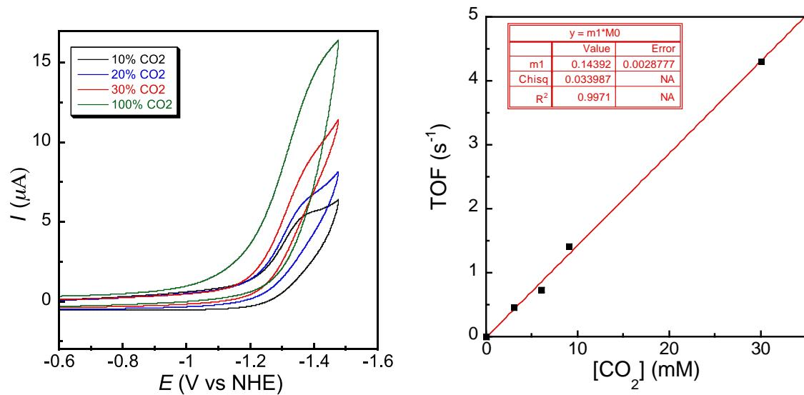
**Figure S4.** Left: cyclic voltammograms of  $\mathbf{2}^{\text{MeCN}}$  in water under 0.1–1 atm  $\text{CO}_2$ ; Right: plot of catalytic TOF vs.  $\text{CO}_2$  concentration in water. (glassy carbon working electrode,  $7.1 \text{ mm}^2$ , 0.1 M  $\text{NaHCO}_3$ , scan rate 50 mV/s, 1% v/v MeCN, room temperature, 1 atm total pressure balanced with Ar)
