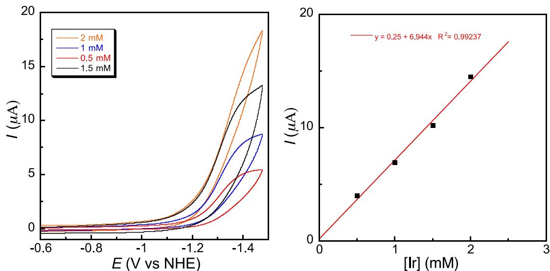
**Figure S3.** Left: cyclic voltammograms of  $0.5\text{--}2 \text{ mM } \mathbf{2}^{\text{MeCN}}$  in water under  $1 \text{ atm CO}_2$ ; Right: plot of catalytic current  $i_{\text{cat}}$  at the catalytic peak potential vs. Ir concentration. (glassy carbon working electrode,  $7.1 \text{ mm}^2$ ,  $0.1 \text{ M NaHCO}_3$ , scan rate  $100 \text{ mV/s}$ ,  $1\% \text{ v/v MeCN}$ , room temperature)
