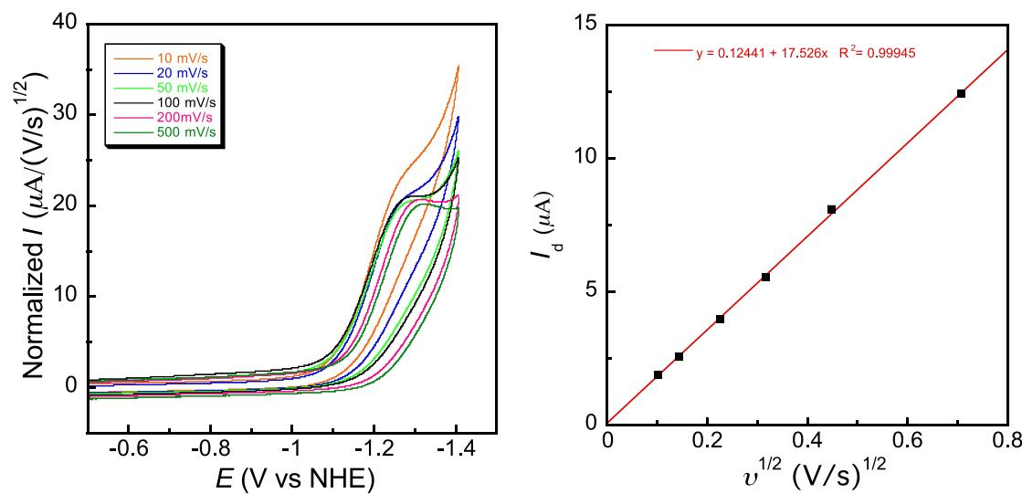
**Figure S1.** Left: cyclic voltammograms of **2**<sup>MeCN</sup> at various scan rates under Ar with currents normalized with respect to the square root of the scan rates. Right: plot of peak current  $i_d$  under Ar against the square root of the scan rate ( $v^{1/2}$ ,  $v$  in V/s). (glassy carbon working electrode, 7.1 mm<sup>2</sup>, 1mM Ir, 0.1 M NaHCO<sub>3</sub>, 1% v/v MeCN, room temperature)
