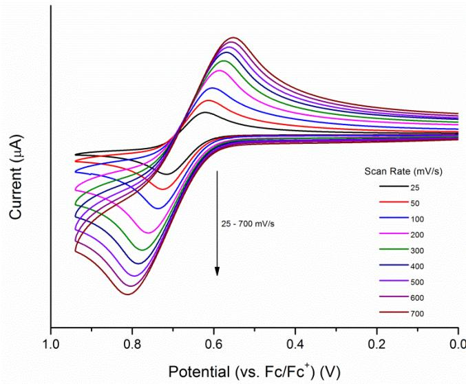
**Figure S4.** Cyclic voltammograms of  $\mathbf{1}$  ( $1 \times 10^{-3} \text{ M}$ ) at increasing scan rates (25 mV/s → 700 mV/s) (0.1 M *n*-Bu<sub>4</sub>PF<sub>6</sub> in CH<sub>2</sub>Cl<sub>2</sub>)
