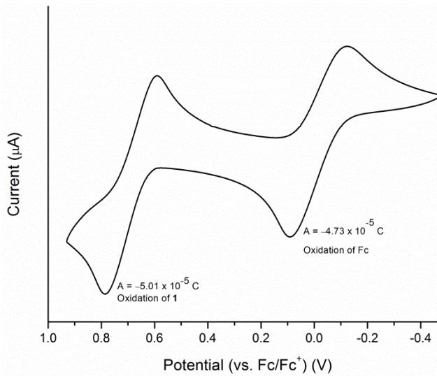
**Figure S5.** Cyclic voltammogram of **1** ( $1 \times 10^{-3} \text{ M}$ ) containing 1 equivalent of ferrocene (0.1 M  $n\text{-Bu}_4\text{PF}_6$  in  $\text{CH}_2\text{Cl}_2$ , scan rate = 50 mV/s).  $A_{\mathbf{1}} / A_{\text{Fc}} = 1.06$ .
