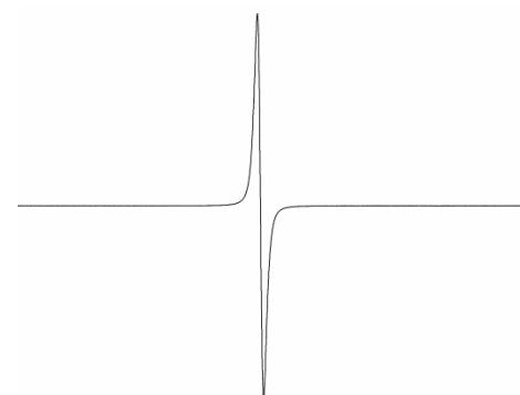
**Figure S9.** X-band EPR spectrum of charge-resonance dimer  $(\mathbf{1})_2^{\cdot+}$  in  $\text{CH}_2\text{Cl}_2$  after the completion of titration experiments (Frequency = 9.389929 GHz, *g* = 2.007 G)
