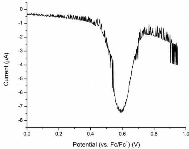
**Figure S6.** Differential pulse voltammogram of radical cation  $\mathbf{1}^+$  (0.1 M  $n\text{-Bu}_4\text{PF}_6$  in  $\text{CH}_2\text{Cl}_2$ ) (pulse height = 25 mV, scan increment = 2 mV)
