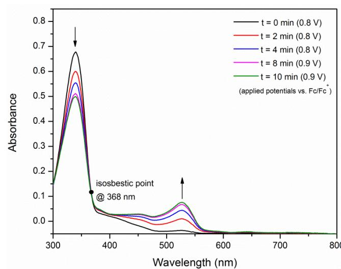
**Figure S7.** UV-vis spectrum (in CH<sub>2</sub>Cl<sub>2</sub>) depicting the gradual oxidation over time of neutral **1** to radical cation **1**<sup>+</sup> with an applied potential. Applied potentials are all relative to the Fc/Fc<sup>+</sup> couple for consistency when referring to cyclic voltammogram (Figure S4)
