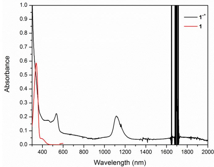
**Figure S1.** UV-vis-NIR spectrum of  $\mathbf{1}^+$  ( $2.7 \times 10^{-4}$  M) and  $\mathbf{1}$  ( $6.4 \times 10^{-6}$  M). The absence of an absorption at 340 nm and a CR band in the NIR confirms the purity of  $\mathbf{1}^+$ .
