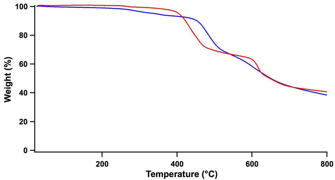
**Fig. S4.** TGA curves of  $D_{TP}-A_{NDI}-COF$  (blue) and  $D_{TP}-A_{PyrDI}-COF$  (red).
