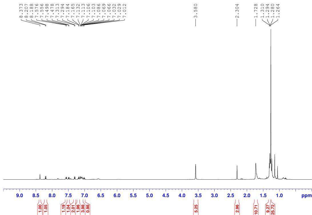
**Figure S7.** <sup>1</sup>H NMR spectrum of **6**·C<sub>7</sub>H<sub>8</sub> (400.13 MHz, 300 K, d<sub>8</sub>-THF).
