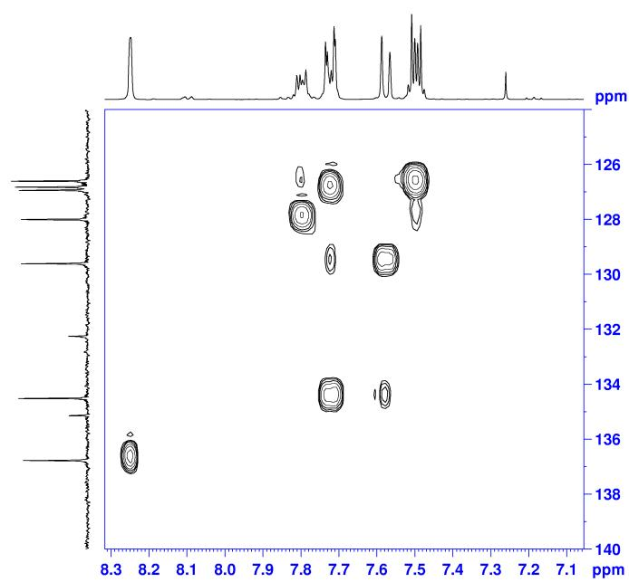
**Figure S23.** <sup>1</sup>H, <sup>13</sup>C-HSQC NMR spectrum of **9** (400.13 MHz, 300 K, CDCl<sub>3</sub>).
