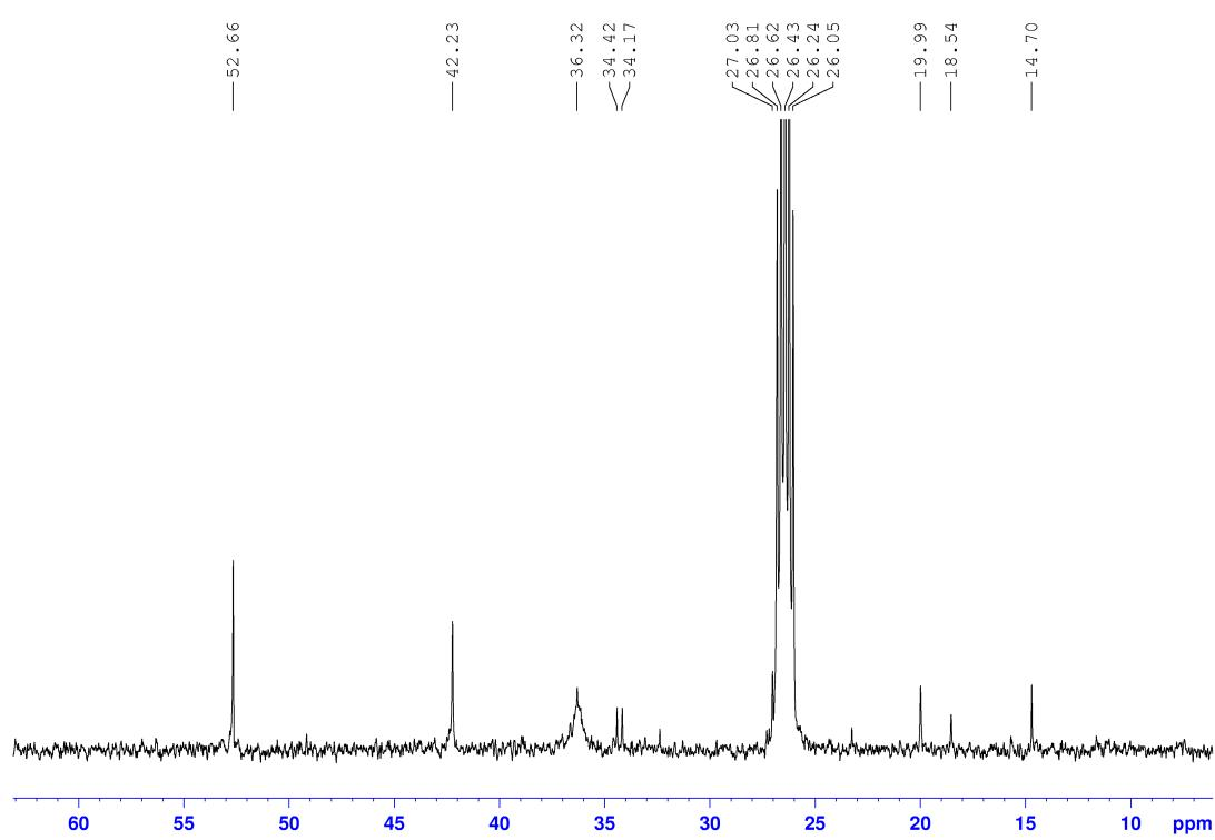
**Figure S2.**  $^{13}\text{C}\{^1\text{H}\}$  NMR spectrum of **3** (100.62 MHz, 300K, *cyc*- $\text{C}_6\text{D}_{12}$ ).
