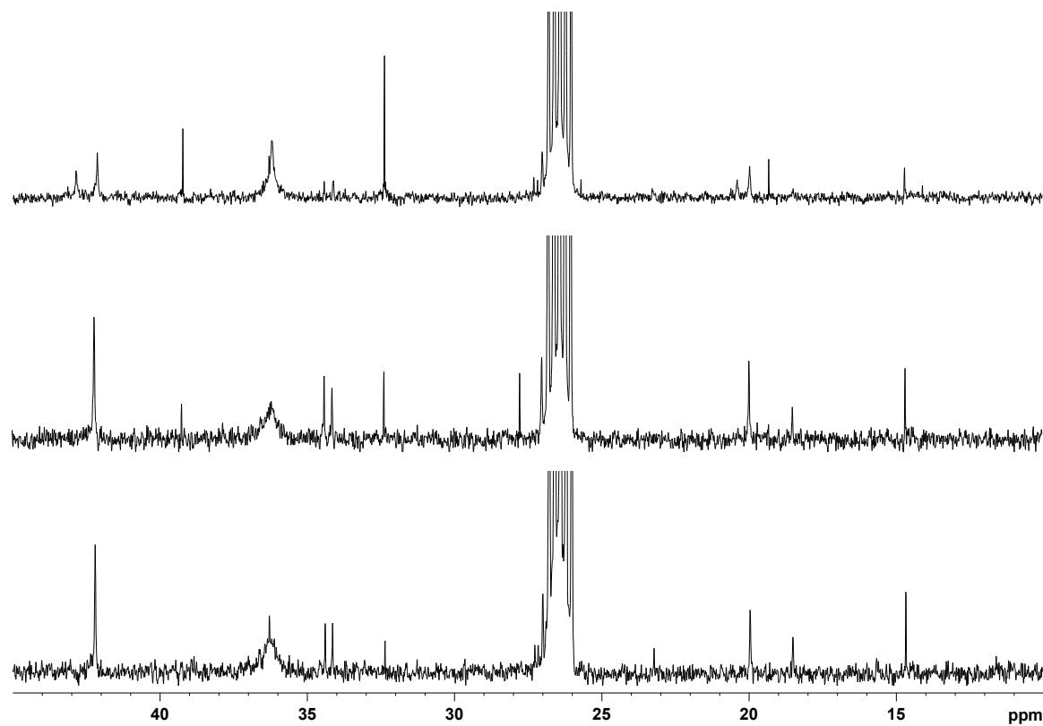
**Figure S6.** <sup>13</sup>C NMR spectrum of **4** (up), **5** (middle) and reaction crude from KTMP·TMPMgBu (*in situ*) mixture (100.62 MHz, 300K, cyc-C<sub>6</sub>D<sub>12</sub>).
