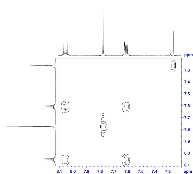
**Figure S26.**  $^1\text{H},^1\text{H}$ -COSY NMR spectrum of **10** (400.13 MHz, 300 K,  $\text{CDCl}_3$ ).
