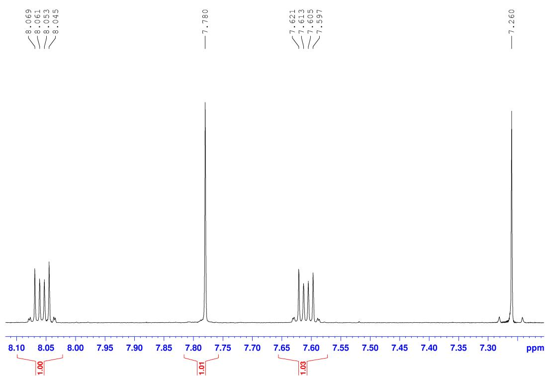
**Figure S24.** <sup>1</sup>H NMR spectrum of **10** (400.13 MHz, 300 K, CDCl<sub>3</sub>).
