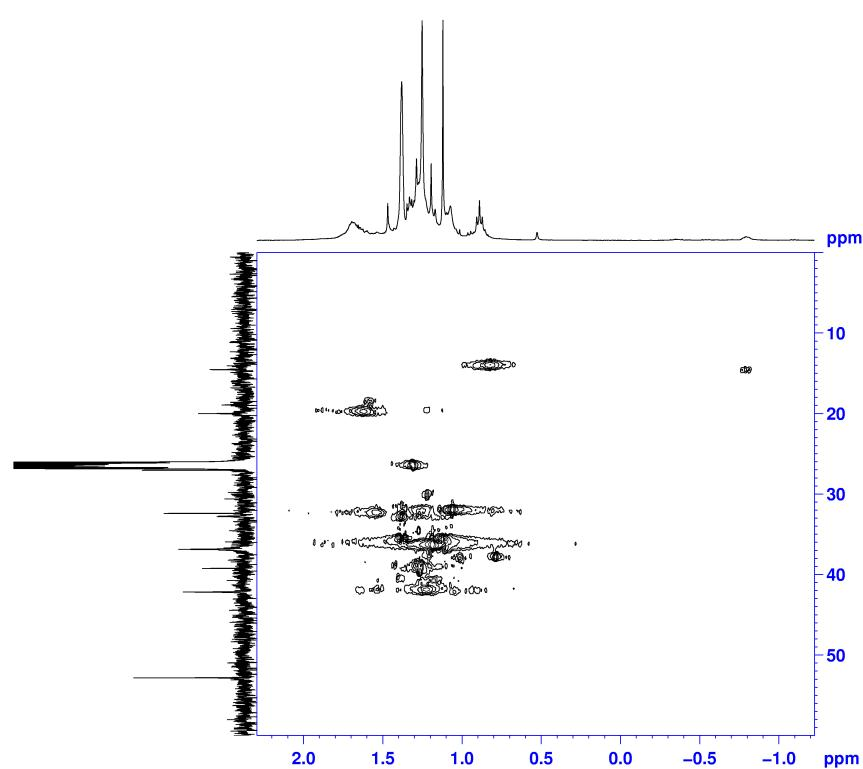
**Figure S14.**  $^1\text{H}$ ,  $^{13}\text{C}$ -HSQC NMR spectrum of **7** (400.13 MHz, 300 K, *cyc*- $\text{C}_6\text{D}_{12}$ ).
