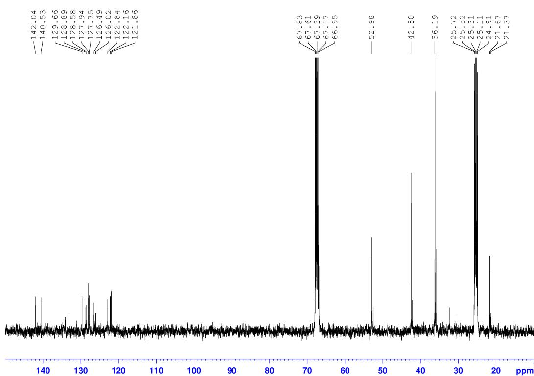
**Figure S8.**  $^{13}\text{C}\{^1\text{H}\}$  NMR spectrum of **6**· $\text{C}_7\text{H}_8$  (100.62 MHz, 300K,  $d_8$ -THF).
