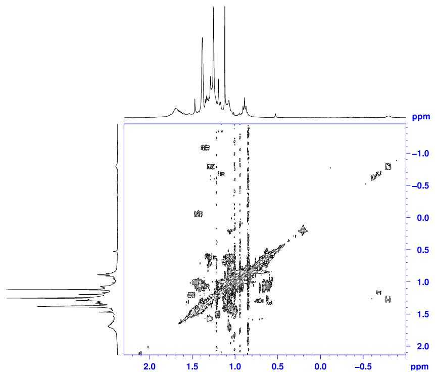
**Figure S13.**  $^1\text{H}$ ,  $^1\text{H}$ -COSY NMR spectrum of **7** (400.13 MHz, 300 K, *cyc*- $\text{C}_6\text{D}_{12}$ ).
