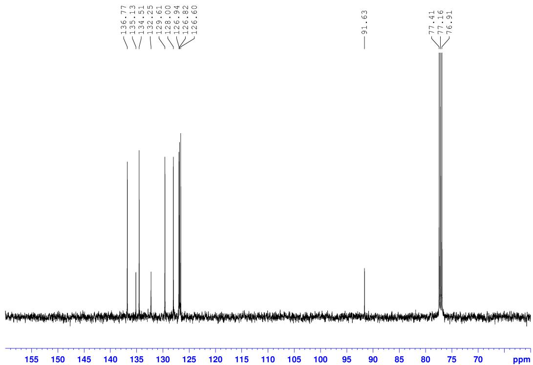
**Figure S21.**  $^{13}\text{C}\{\text{H}\}$  NMR spectrum of **9** (100.62 MHz, 300K,  $\text{CDCl}_3$ ).
